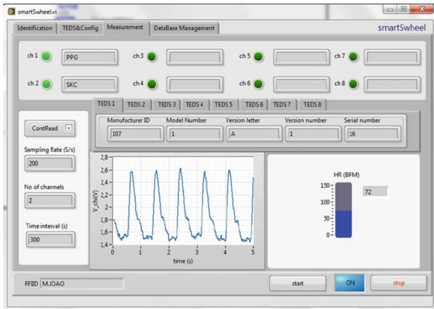
**Fig. 6** The graphical user interface of smart sensors for wheelchair (SmartWheel) LabVIEW application
