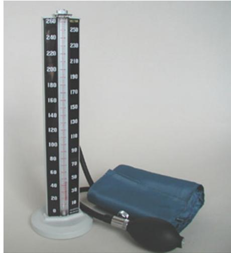
From the measurement of  $h_u$ , with the knowledge on the acceleration due to gravity  $g$  at the measurement site, and the density of the fluid  $\rho_u$ , we can compute the pressure difference  $(P_1 - P_2)$  as:
