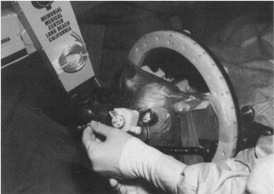
FIGURE 20-5. A biopsy probe is passed through the robotic "hand" on a trajectory predetermined by CT scan and computer-driven robotic positioning.
