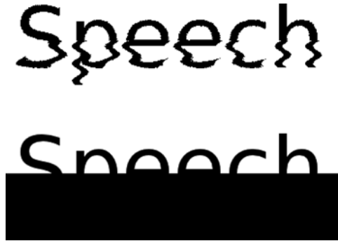
Figure 14.1 A visual analogy comparing two views of the robust ASR problem: noise as a source of model mismatch versus noise as a source of information loss. The distortion in the top panel is invertible and the original signal could theoretically be recovered if the model for the distortion was known. The occlusion in the bottom panel is not invertible and information has been genuinely lost.
