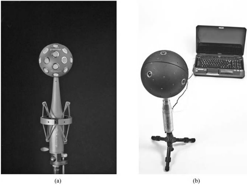
Figure 6.19 (a) A 32-channel Eigenmike ® spherical array; photo reproduced courtesy of mh acoustics, Inc. (b) A 64-channel spherical array with five integrated video cameras; photo reproduced courtesy of VisiSonics Corporation.
