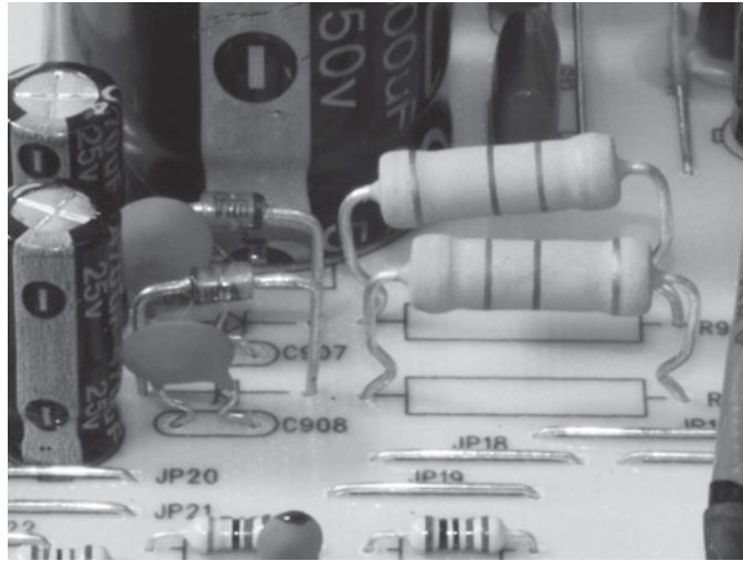
FIGURE 9-4 Zener diodes and fusible resistors on the power board
