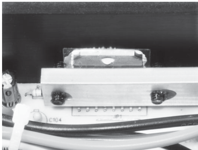
FIGURE 9-8 Mica insulator sheet between heat sink and amplifier IC
