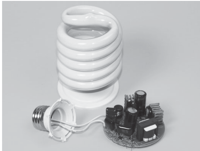
FIGURE 6-1 Compact fluorescent lamp, partially disassembled
