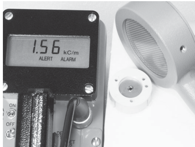
FIGURE 1-5 Radiation meter reading Americium alpha particle activity
