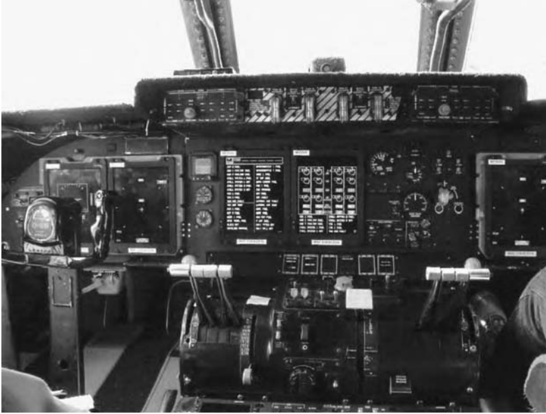
FIGURE 12.6 Navigation displays in the U.S. Air Force C-5 transport showing flat-panel displays in front of each pilot; vertical situation display outboard and horizontal situation display inboard. Waypoints are entered on the horizontally mounted control-display unit just visible aft of the throttles. In the center of the instrument panel are status and engine displays and backup analog instruments. (Photo courtesy of Honeywell, Copyright 2004.)
