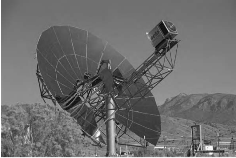
FIGURE 2.7 Advanced dish development system (ADDs) on test at Sandia National Laboratories’ National Solar Thermal Test Facility. (Photograph courtesy of Sandia National Laboratories.)
