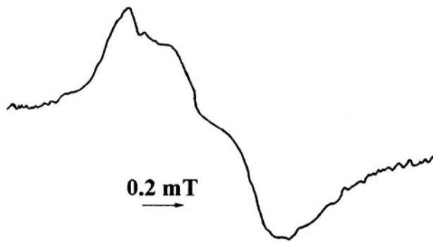
Figure 9. EPR spectrum of C_{\infty} in a mixture of toluene and sulfuric acid at 77 K. 23
