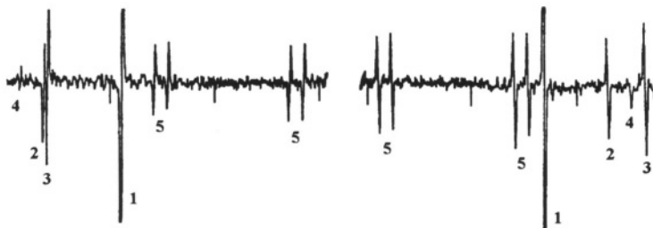
Figure 12. EPR spectra of ^{\bullet}C_{70}H (1-4) and ^{\bullet}C_{70}H_3 (5). Adapted from ref 14.
