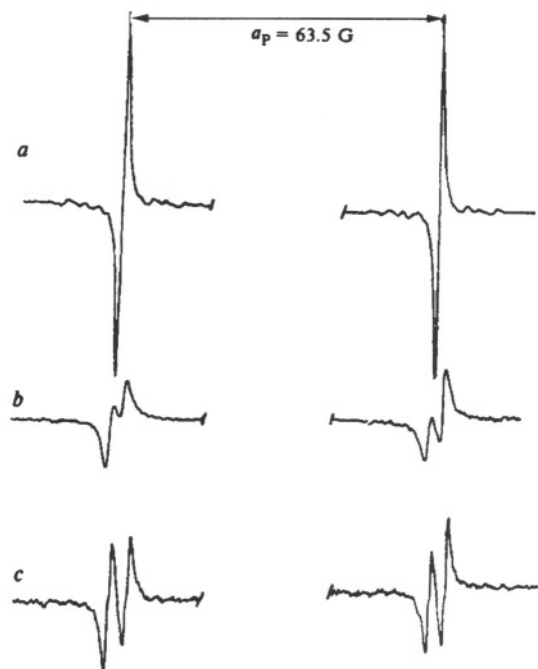
Figure 19. EPR spectrum of radical \cdot\text{C}_{60}\text{P}(\text{O})(\text{OPr})_2 at 300 K (a), 233 K (b), and 200 K (c). 52
