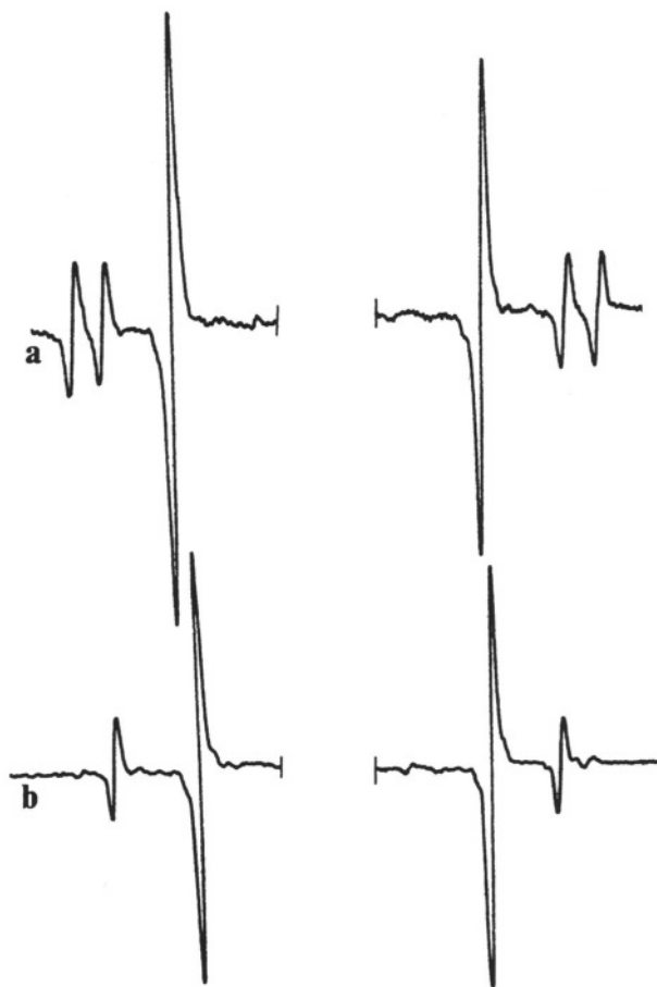
Figure 9. EPR spectra of \cdot\text{C}_{x}\text{P}(\text{O})(\text{OEt})_2 at (a) 300 K and (b) 400 K. 11
