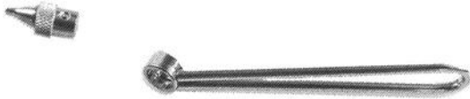
Fig. 114. DCP drill guide with handle, 2.0 mm diam., with two settings marked 0 and 0.8. The 0 setting centers the guide for drilling the 2.0-mm thread hole at the exact center of the DC hole, resulting in a neutral screw position. The 0.8 setting places the guide for the 2.0-mm thread hole off-center in the plate hole so that the screw effects compression (see Fig. 31)
