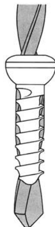
◁ Fig. 143. The gliding hole matches the thread diameter of the 2.7-mm screw
