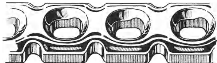
Fig. 58. The reconstruction plate has two-way DC holes or applying compression in either longitudinal direction
