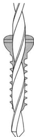
Fig. 144. The compression hole matches the core diameter of the screw (1.9 or 2.0 mm diam.). (From Brinker et al. 1984) ▷
