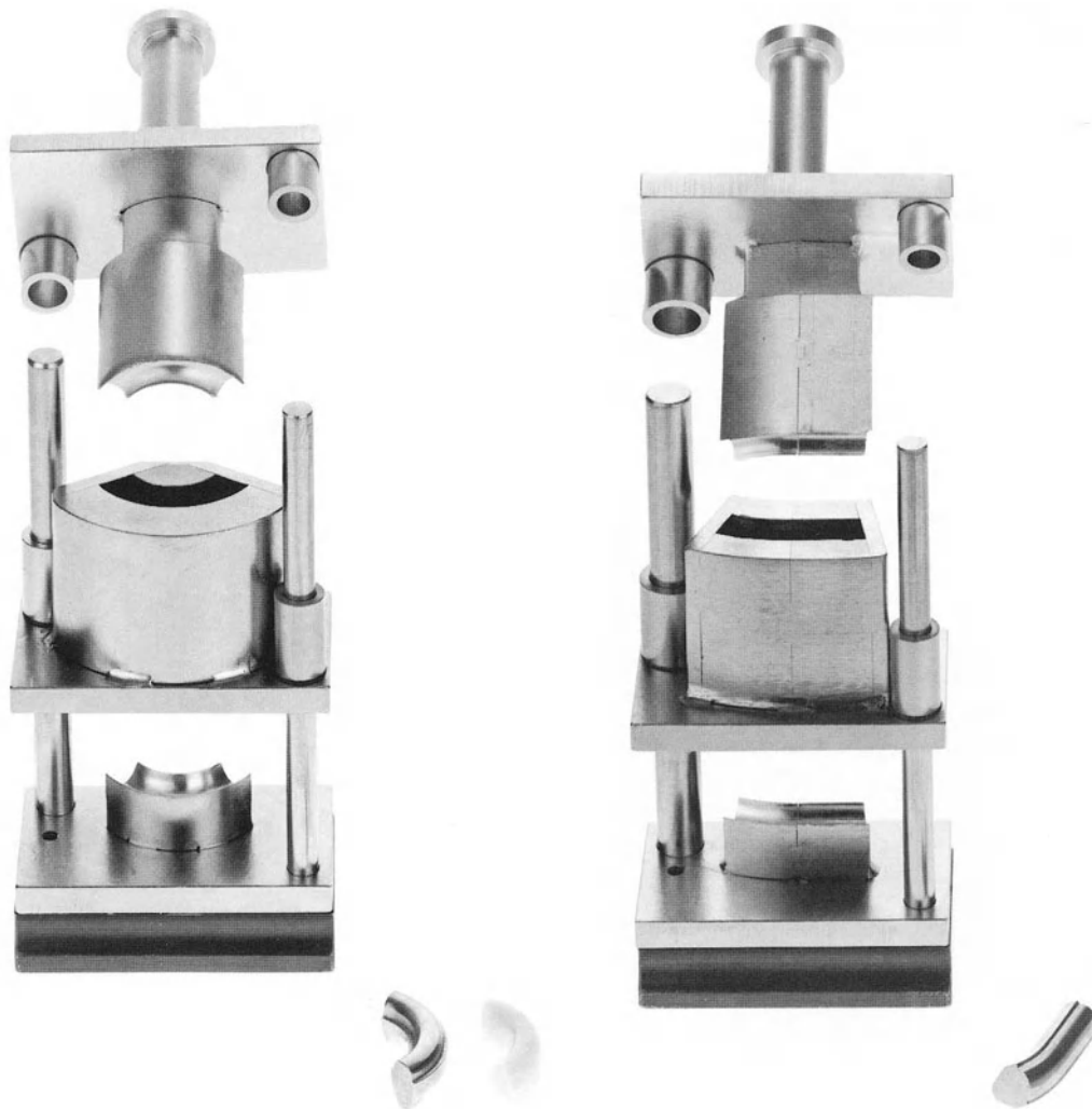
Fig. 342. Upper and lower dies of the cancellous bone press. Left: For production of the central (chin) segment. Right: For production of a lateral segment
