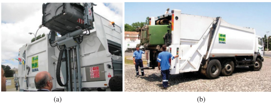
FIGURE 2.7 Vehicles with a side loader (a) and a rear loader (b). Courtesy: SUMA – Serviços Urbanos e Meio Ambiente
