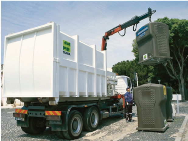
FIGURE 2.8 Cyclea container discharge to a crane vehicle. Courtesy: SUMA – Serviços Urbanos e Meio Ambiente
