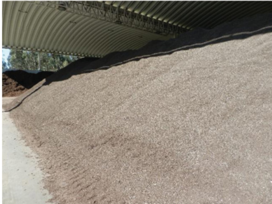
FIGURE 2.19 Compost produced from digestate of mixed MSW anaerobic digestion. Courtesy: Valorlis, S.A.
