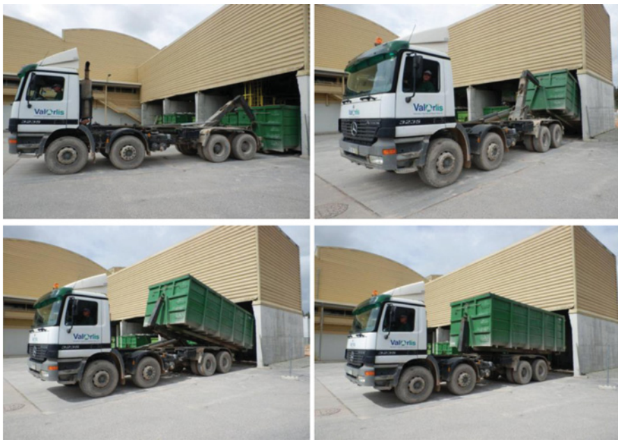
FIGURE 2.9 Hooklift hoist collection system. Courtesy: Valorlis, S.A.
