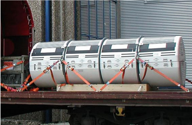
Fig. 4.9 UF 6 container for low enriched uranium leaving of enrichment plant (URENCO)
