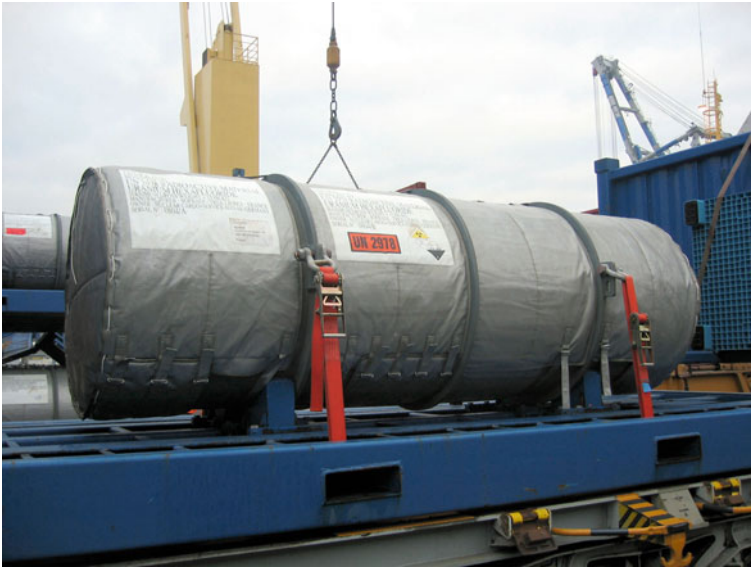
Fig. 4.1 UF 6 transport container going to enrichment plant (URENCO)
