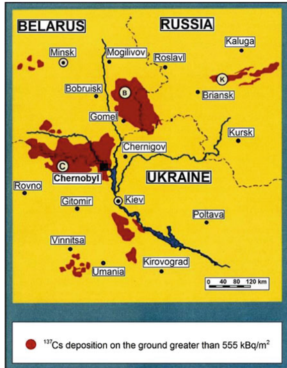
Fig. 11.31 Cs-137 contamination from Chernobyl accident in different areas of the Ukraine, Belarus and Russia [75]
