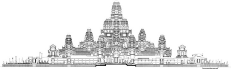
Fig. 8 Reconstruction of the eastern façade of the Bayon as suggested by Dumarçay (ESEO, 1967). The author decided not to reconstruct the outer gallery superstructures. Yet, in his 1973 publication, Dumarçay suggested faceless tower roofing on the pavilion of this gallery (Dumarçay and Groslier 1973, 26) (Source: Dumarçay 1967, plate LXVII)
