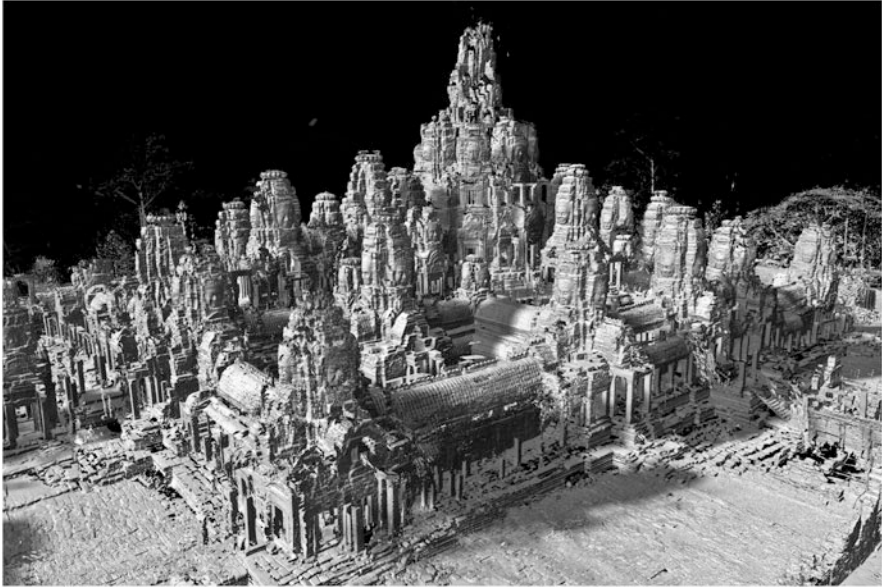
Fig. 6 Results of the 3D laser scanning of the Bayon temple, Ikeuchi Laboratory (Japan 2007) (Ikeuchi Laboratory—Institute of Industrial Science, University of Tokyo, Japan 2007)
