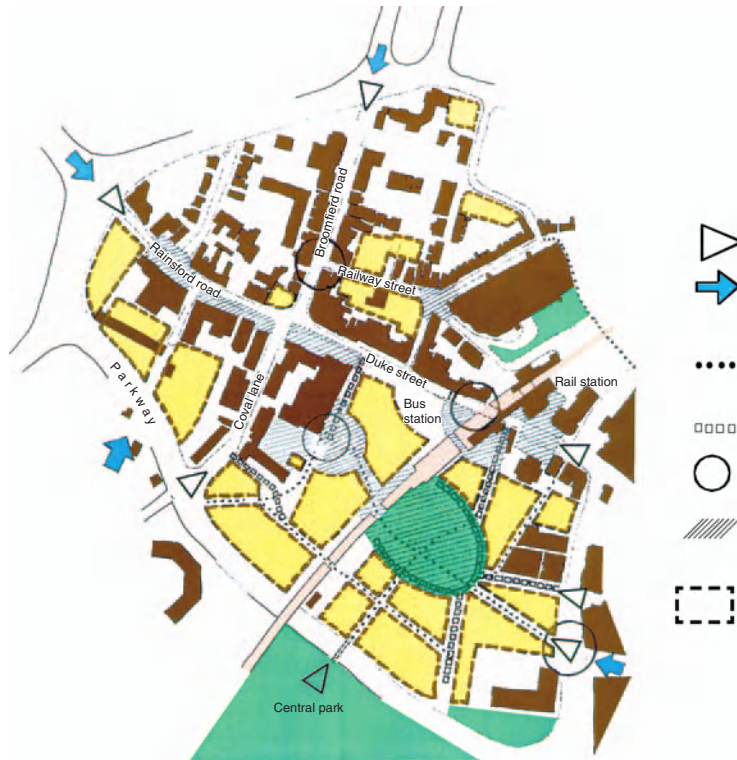
Plate 6.2 An extract from the West End master plan (CBC, 2000a) showing the proposed reconfiguration of pedestrian spaces. Reproduced with the permission of Chelmsford Borough Council and the Ordnance Survey on behalf of HMSO. © Crown Copyright 2007. All rights reserved. Licence number 100046642.
