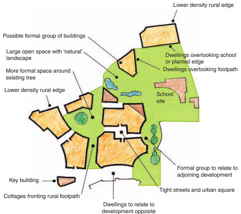
Plate 5.8 The diagram from the Beaulieu Park North Master Plan (CBC, 2001a) showing how character areas should be formed. Source: Chelmsford Borough Council.
