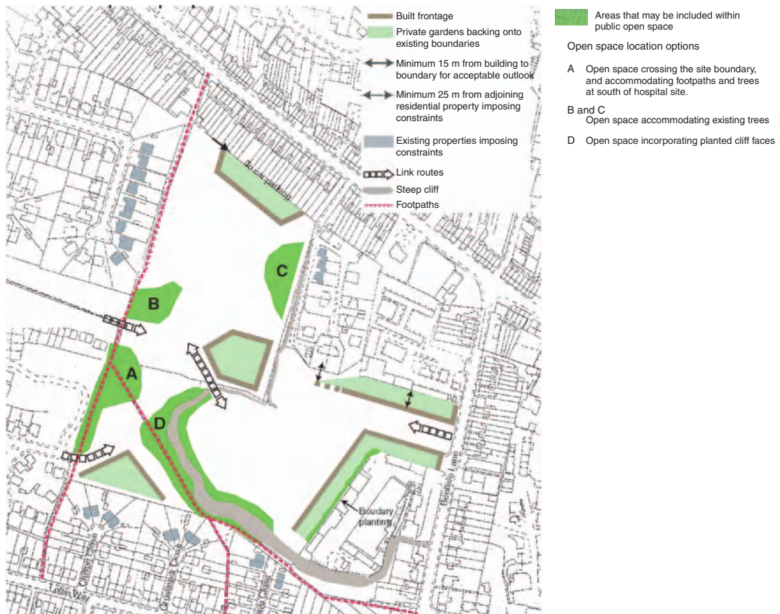
Plate 5.9 The diagram from the Planning Brief (CBC, 2001b) showing built frontage and open space options for the site of the Clarendon Park scheme. Reproduced with the permission of Chelmsford Borough Council and the Ordnance Survey on behalf of HMSO. © Crown Copyright 2007. All rights reserved. Licence number 100046642.
