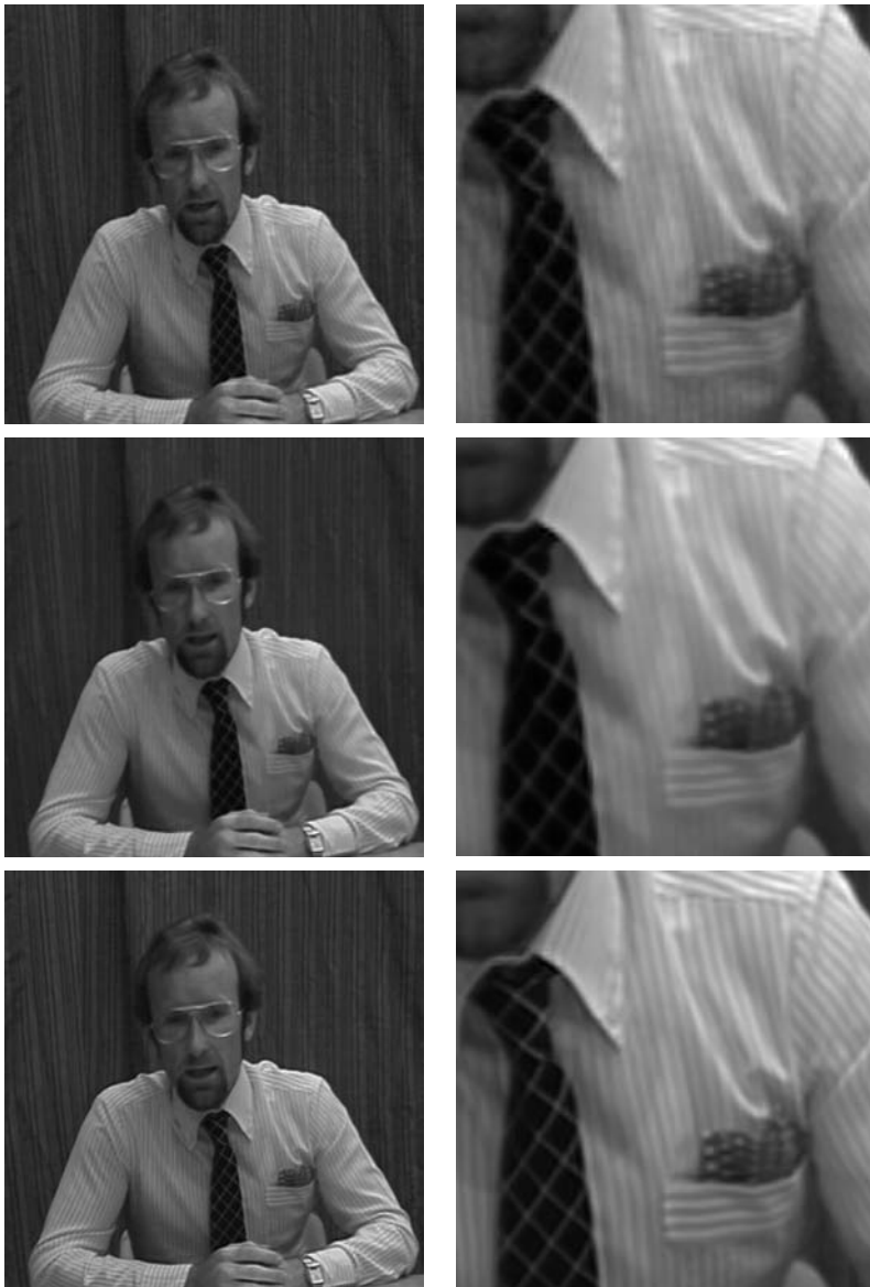
FIGURE 4.6: Original “Trevor” sequence. Top: Interpolated image. Middle: Interpolation, followed by NLM processing and deblurring. Bottom: Proposed algorithm. The right column offers a close-up of a portion of the images.
