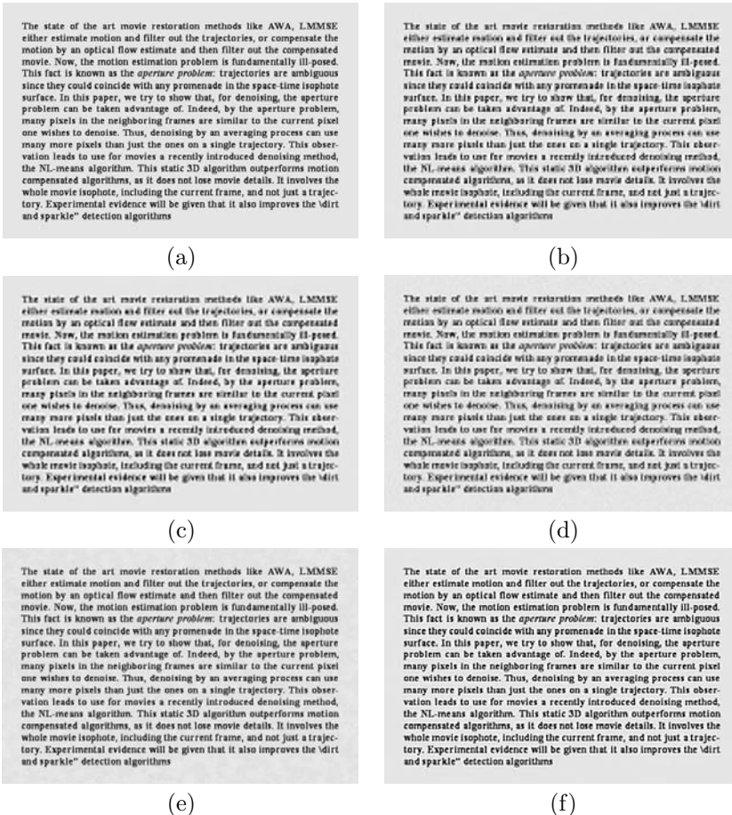
FIGURE 4.1: Results for the synthetic text sequence. (a) Original (ground-truth) image. (b) Pixel replicated image, 13.47dB. (c) Lanczos interpolation, 13.84dB. (d) Deblurred Lanczos interpolation, 13.9dB. (e) Result of shift-and-add algorithm [5, 7], 18.4dB. (f) Result of proposed algorithm, 18.48dB.
