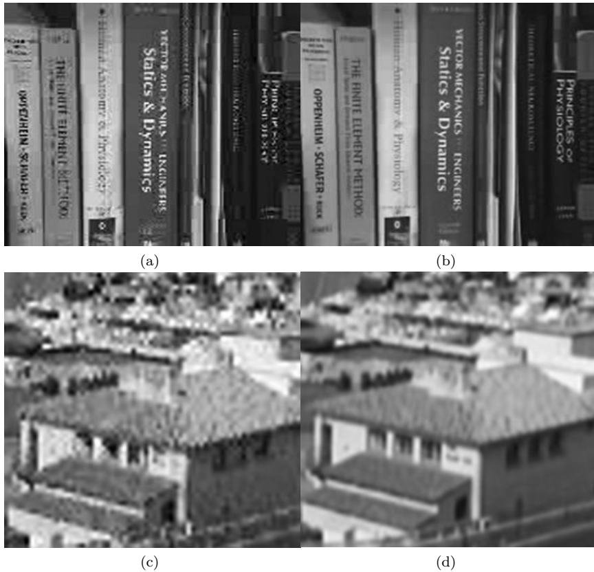
FIGURE 14.4: Sample super-resolution results for cellphone (top) and digital still camera video (bottom). (a) Original frame, upscaled 2\times using bicubic interpolation. Source: H.263 video at 170 kbps, 176\times 144 at 5 fps, (b) Super-resolution results ( 2\times ) using 21 matching frames. (c) Detail from original frame, upscaled 2\times using bicubic interpolation. Source: MotionJPEG video at 2.7 Mbps, 320\times 240 at 15 fps, (d) Super-resolution results ( 2\times ) using 31 matching frames.
