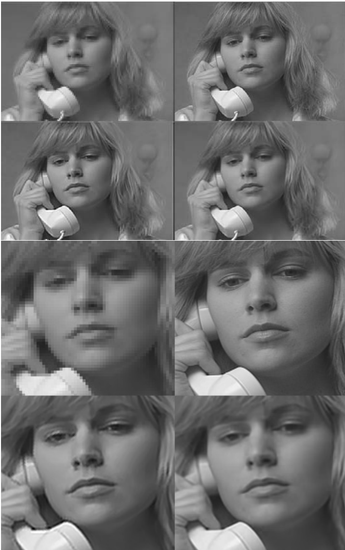
FIGURE 5.13: Results for the 23rd frame from the Suzie sequence. From left to right and from top to bottom: pixel-replicated low-resolution image; original image (ground truth); super-resolved by the algorithm [29]; super-resolved by the proposed algorithm and their respective zoomed fragments.
