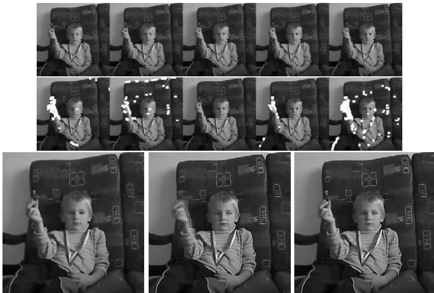
FIGURE 7.5: Super-resolution of a scene with local motion. The first row shows five consecutive input frames acquired by a web camera. The second row shows masks (white areas), which indicate regions with possible local motion. The third row shows the estimated original image using simple interpolation (left), super-resolution without masking (central), and proposed super-resolution with masking (right).
