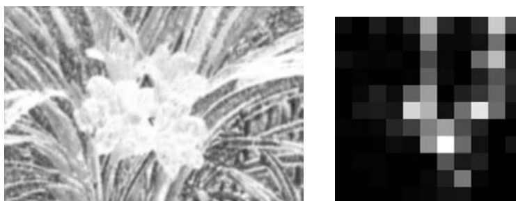
FIGURE 7.10: Depth map corresponding to images in Figure 7.9 and the PSF estimated locally around the flowers close to the center of the left input image.
