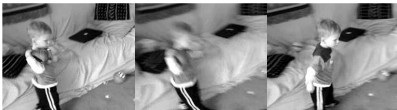
FIGURE 14.8: Three frames from the sequence affected by motion blur. Automatic detection of blurred frames could improve SR results in general by excluding these frames from processing.
