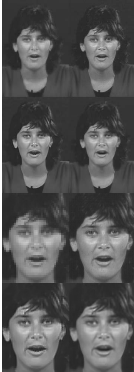
FIGURE 5.14: Results for the 23rd frame from the Miss America sequence. From left to right and from top to bottom: pixel-replicated low-resolution image; original image (ground truth); super-resolved by the algorithm [29]; super-resolved by the proposed algorithm and their respective zoomed fragments.
