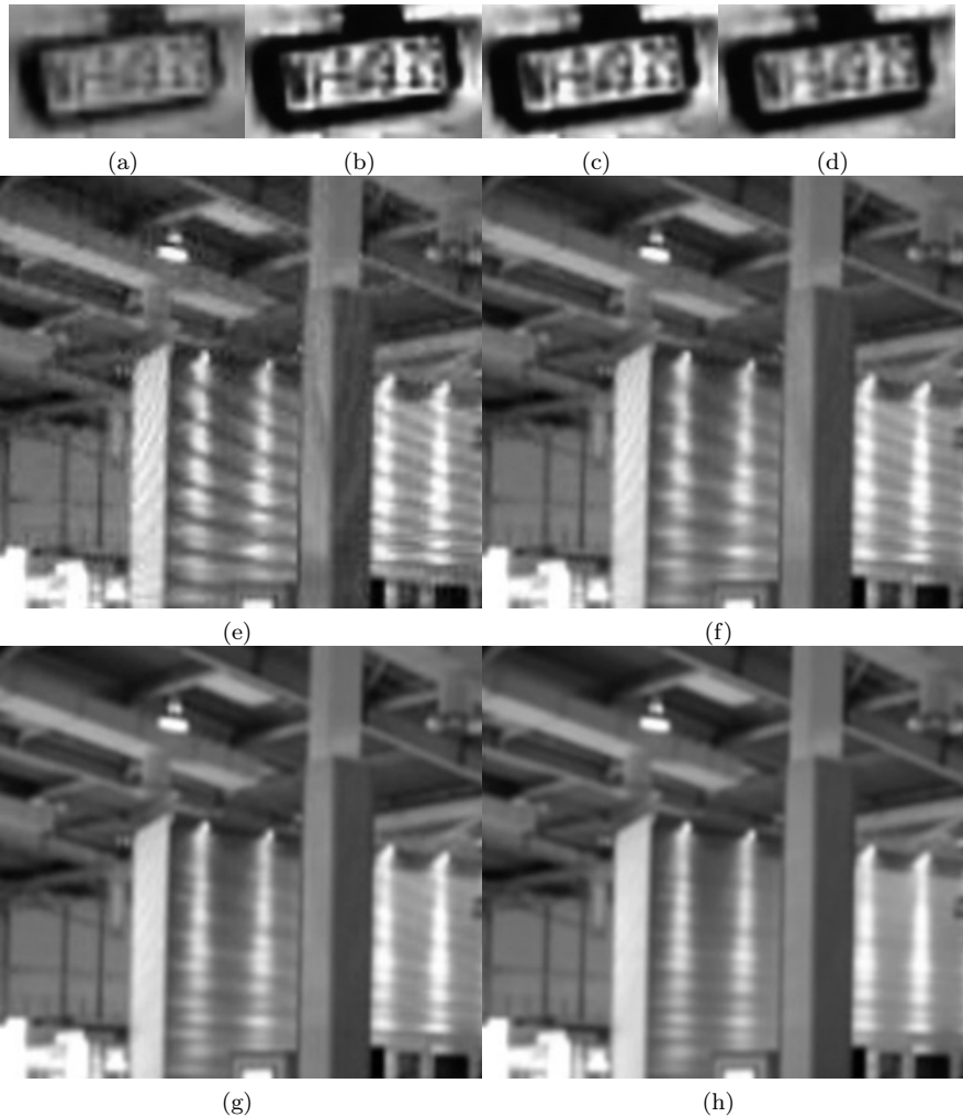
FIGURE 14.7: Demonstrating visual improvements in reconstruction when increasing the number of matching frames. (a)–(d) Improving resolution. a) Original frame upscaled 2\times using bicubic interpolation, b) Original frame after contrast adjustment ( 2\times bicubic upscaling), c) 2\times SR result using 5 matching frames, d) 2\times SR result using 15 matching frames. The license plate number is clearly readable only in the last image (NI-949 29). (e)–(h) Removing compression noise and Moiré patterns. (a) no SR ( 2\times bicubic upscaling), (b) 2\times SR, 5 matching frames, (c) 2\times SR, 15 matching frames, (d) 2\times SR, 50 matching frames. Notice how in this example 15 frames are not sufficient to completely remove Moiré patterns. MotionJPEG at 3.4 Mbps, 320 \times 240 at 20 fps.
