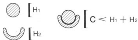
Fig. 12. Forceps with a hollowed blade. One blade is trough-shaped, the other cylindrical. The stability of each blade depends on its height ( H ). Since the two blades interlock, the total cross-section ( C ) is smaller than the sum of the blade heights ( H ). Owing to the curvature of the grasping surfaces, the advantages of grooving are present
