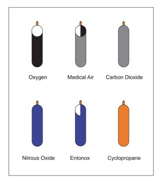
Figure 4.2 United Kingdom colour codes for medical gas cylinders.
