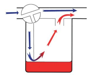
**Figure 4.7** Diagrammatic representation of a simple plenum vaporiser. Anaesthetic gas passes through the vaporiser (black arrows). That which passes through the vaporisation chamber becomes saturated with volatile anaesthetic vapour (white arrows). The output of the vaporiser is altered by turning the control knob to alter the relative flow through and past the vaporisation chamber.
