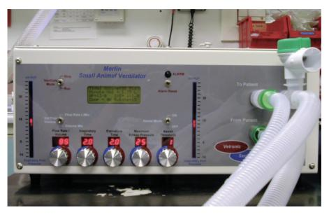
Figure 4.11 A small animal mechanical ventilator unit. This unit can deliver pressure, volume or time cycled intermittent positive pressure ventilation.
