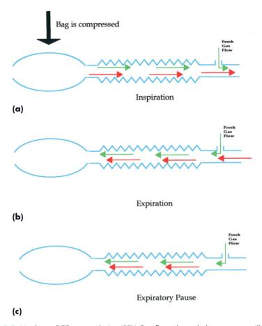
**Figure 5.7** Mapleson DEF system during IPPV. Gas flows through the system are illustrated in (a) inspiration, (b) early expiration, (c) late expiration. White arrows – fresh gas; black arrows – rebreathed gas containing carbon dioxide; dotted arrows – gas which has entered the anatomical dead space but has not undergone gas exchange and so does not contain carbon dioxide. See text for a full explanation.
