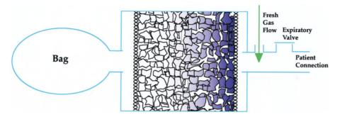
Figure 5.9 Water's canister (to-and-fro) breathing system.
