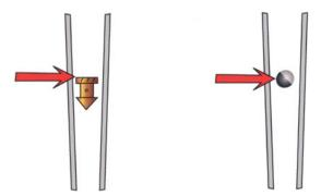
**Figure 4.6** Vane rotameters should be read from the top; ball rotameters should be read from the centre of the ball. The correct level at which to read these two rotameters is indicated by the arrow.
