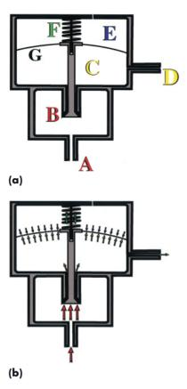
**Figure 4.3** (a) Simplified diagrammatic section through reducing valve. (A) high pressure inlet, (B) high pressure chamber, (C) regulated pressure chamber, (D) regulated pressure outlet, (E) atmospheric pressure chamber, (F) spring.
