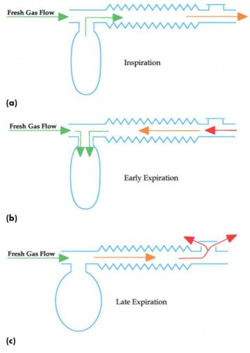
**Figure 5.3** Mapleson A system during spontaneous ventilation. Gas flows through the system are illustrated in (a) inspiration, (b) early expiration, (c) late expiration. White arrows – fresh gas; black arrows – rebreathed gas containing carbon dioxide; dotted arrows – gas which has entered the anatomical dead space but has not undergone gas exchange and so does not contain carbon dioxide. See text for a full explanation.
