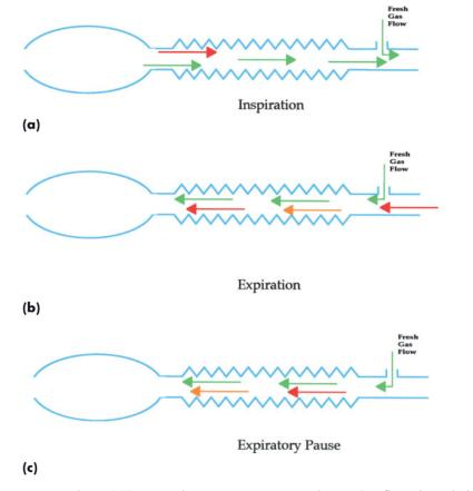
**Figure 5.6** Mapleson DEF system during spontaneous ventilation. Gas flows through the system are illustrated in (a) inspiration, (b) expiration, (c) expiratory pause. White arrows – fresh gas; black arrows – rebreathed gas containing carbon dioxide; dotted arrows – gas which has entered the anatomical dead space but has not undergone gas exchange and so does not contain carbon dioxide. See text for a full explanation.
