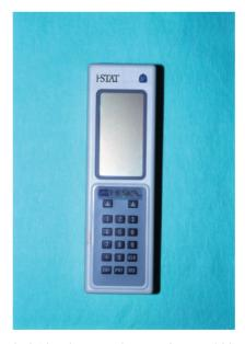
Figure 8.3 i-STAT® 'bedside' biochemistry, haematology and blood gas analyser.
