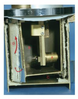
Figure 4.8 Cut-away of early Bowring Medical Engingeering vaporiser.
