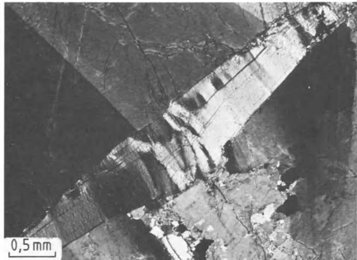
Fig. 158 Tectonically deformed phlogopite with clearly developed kink bands and undulatory extinction, next to deformed olivine. Phlogopite peridotite. Finero, Ivrea area, northern Italy. Crossed polars.
