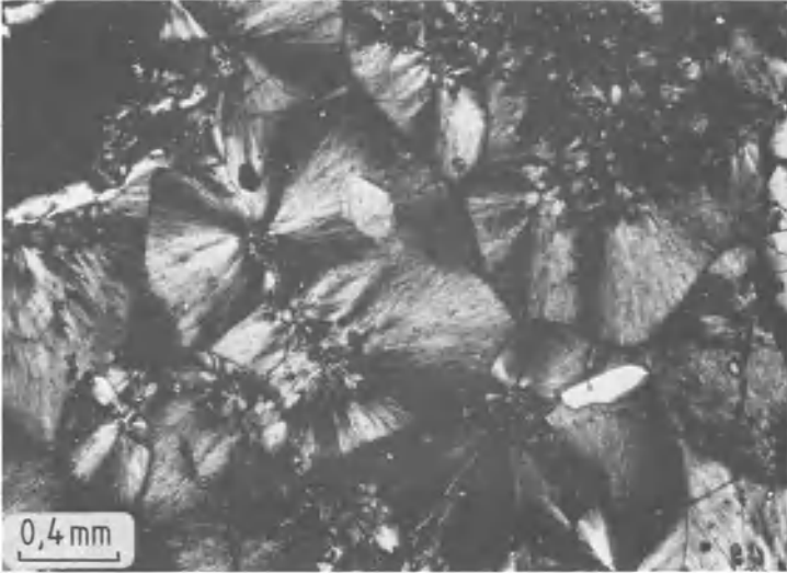
Fig. 66 Acidic volcanic glass with spherulites (devitrification to alkali feldspar and low-cristobalite). Rhyolite. Kremnica, Slovakia. Uncrossed polarizers.
