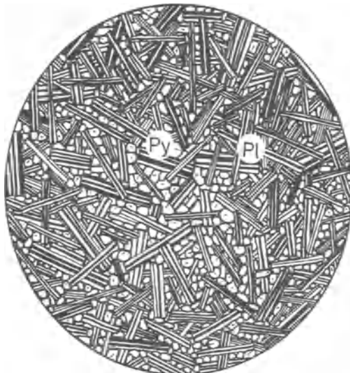
Fig. 265 Intersertal texture. Plagioclase laths randomly oriented embedded in a matrix of pyroxene and rock-glass (basalt).
