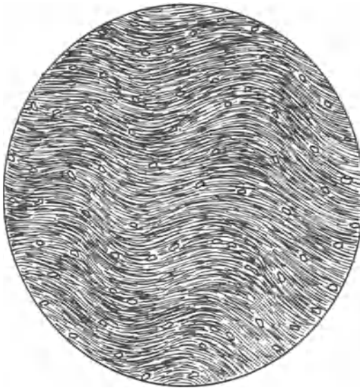
Fig. 273 Lepidoblastic texture. Plicated small-scale sericite flakes and fine quartz grains (phyllite).
