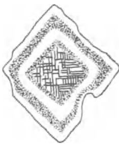
Fig. 53 Nosean and hauyne showing characteristic alignment of inclusions along growth zones (exsolved Fe-ore) and corroded edges.
