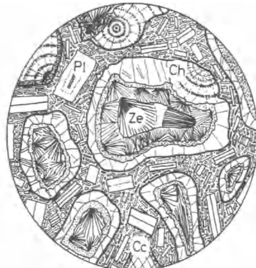
Fig. 266 Amygdaloidal texture of a volcanic rock. Filling of the amygdules by calcite, zeolite and chalcedony.
