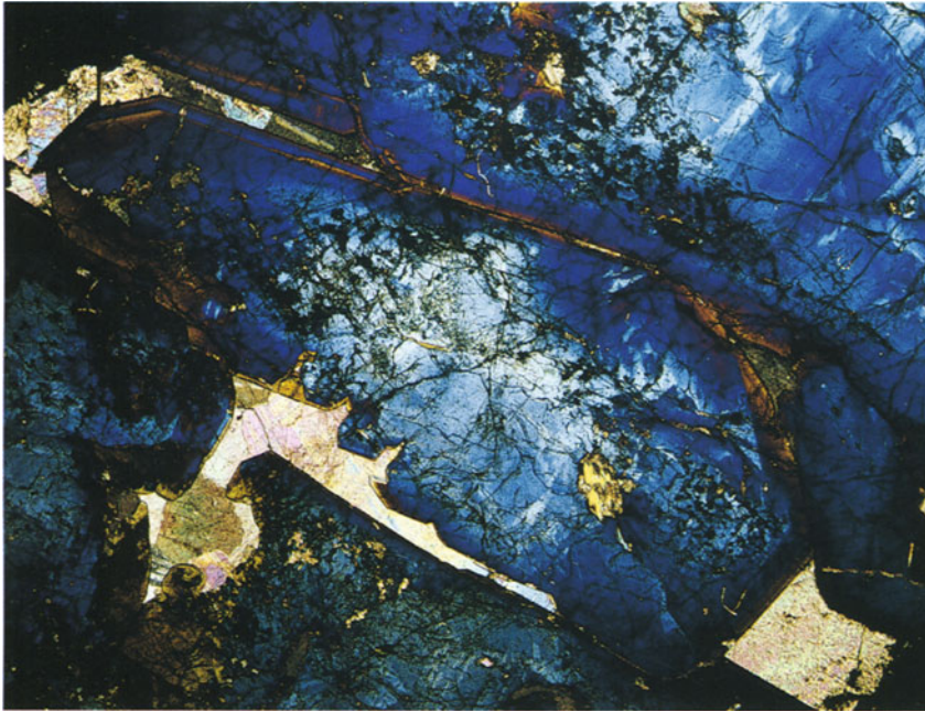
5 Hypidiomorphic vesuvianite crystals with strong anomalous interference colours (lavender-blue to leather-brown), also showing weak cleavage. Accompanying minerals are calcite with greenish to reddish-white interference colours of the higher orders. Contact-metamorphic siliceous carbonate. Predazzo, Dolomites, northern Italy. Crossed polarizers, 8.0 \times 11.0 mm.
