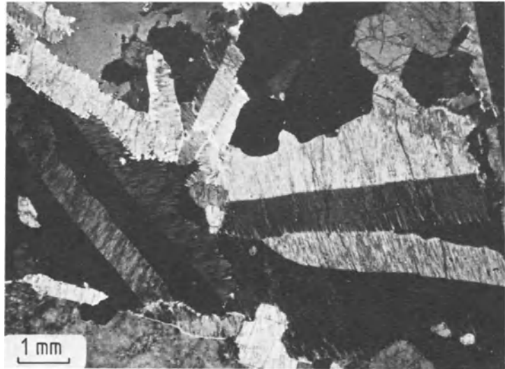
Fig. 182 Orthoclase showing perthite exsolution and characteristic Carlsbad twins. Sodalite syenite. Ditro, Transylvania, Romania. Crossed polars.
