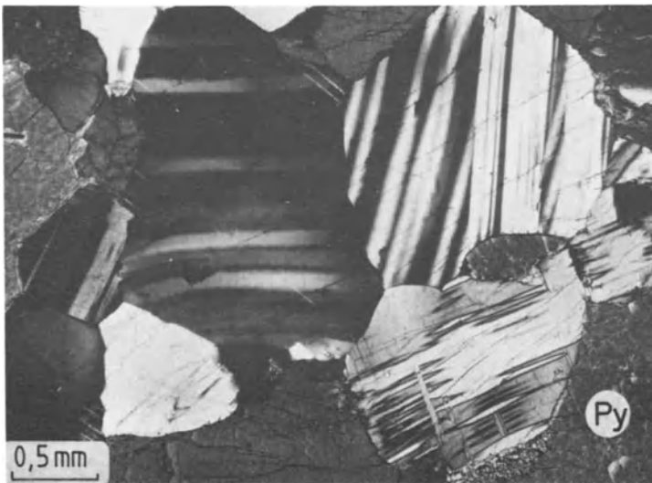
Fig. 192 Hypidiomorphic plagioclase crystal with clearly visible glide-twins next to augite. Tectonized gabbro. Northern Italy. Crossed polars.
