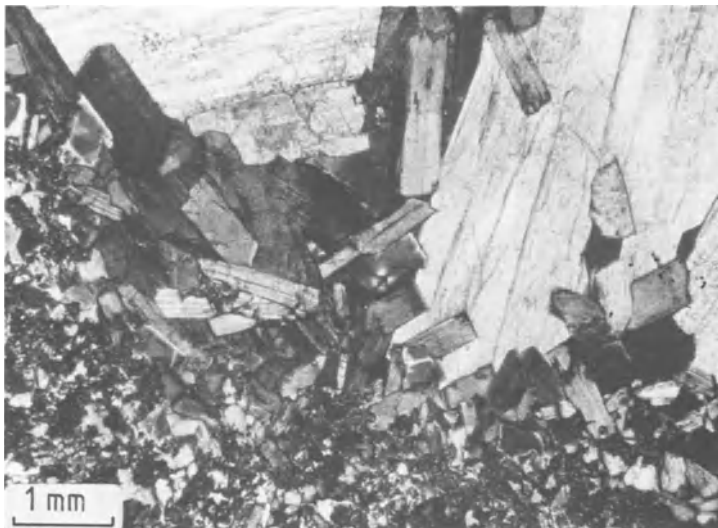
Fig. 212 Columnar to acicular zeolite crystal (phillipsite) filling a cavity. Tertiary zeolite-rich tholeiitic basalt. Teigarhorn, eastern Iceland. Crossed polars.
