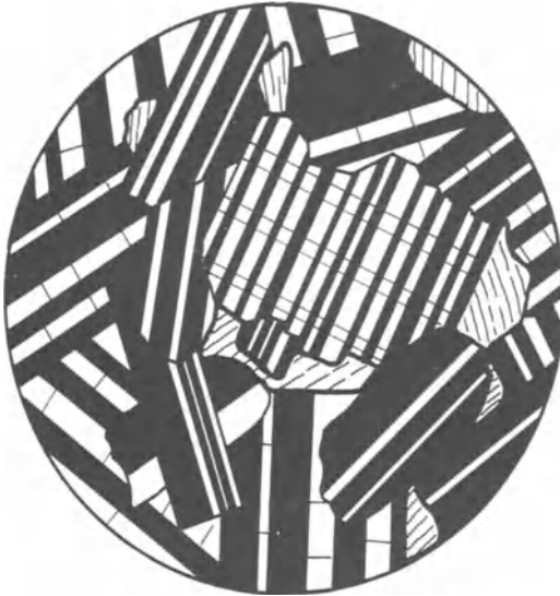
Fig. 191 Polysynthetic twinning plagioclase in anorthosite. The high anorthite content is visible by the broad twin lamellae. Crossed polars.
