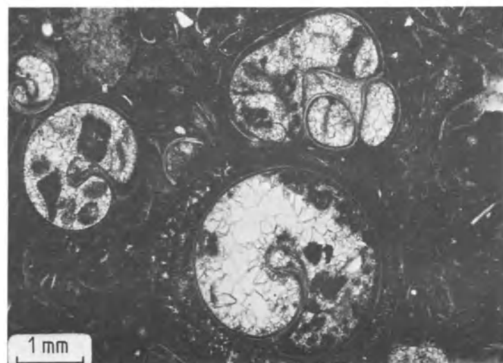
Fig. 93 Organically formed calcite (gastropod shell and other fossils) (sparite) with calcite cement (micrite). Miocene limestone (Hydrobia-limestone) from the Mainz Basin. Crossed polars.
