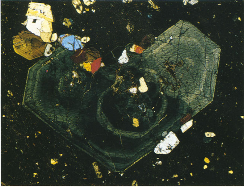
7 Simple twinning in titanite with clear zonal growth pattern and typical anomalous interference colours of the 1st order (grey-blue to dark brown). Clearly developed pyroxene cleavage and crystal outlines. Hyalobasanite. Sasbach, Kaiserstuhl volcano, Germany. Crossed polars, 4.0 × 5.5 mm.
