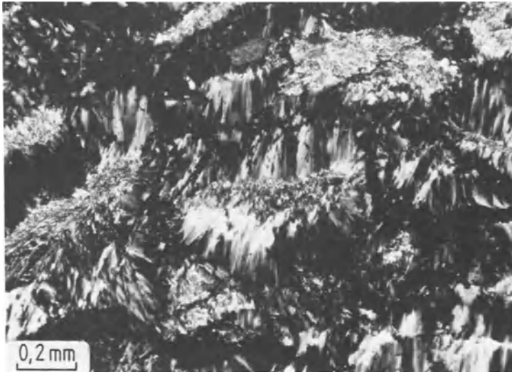
Fig. 172 Fibrous serpentine (chrysotile), formed from serpentinization of olivine. Serpentinite. Finero, Ivrea area, northwestern Italy. Crossed polars.
