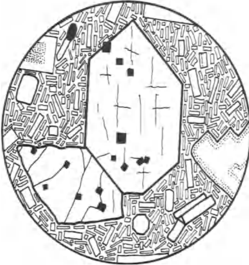
Fig. 114 Idiomorphic olivine crystal with spinel inclusions in a tholeiitic basalt of the Vogelsberg, Germany. Characteristic poor cleavage in olivine. Uncrossed polarizers.
