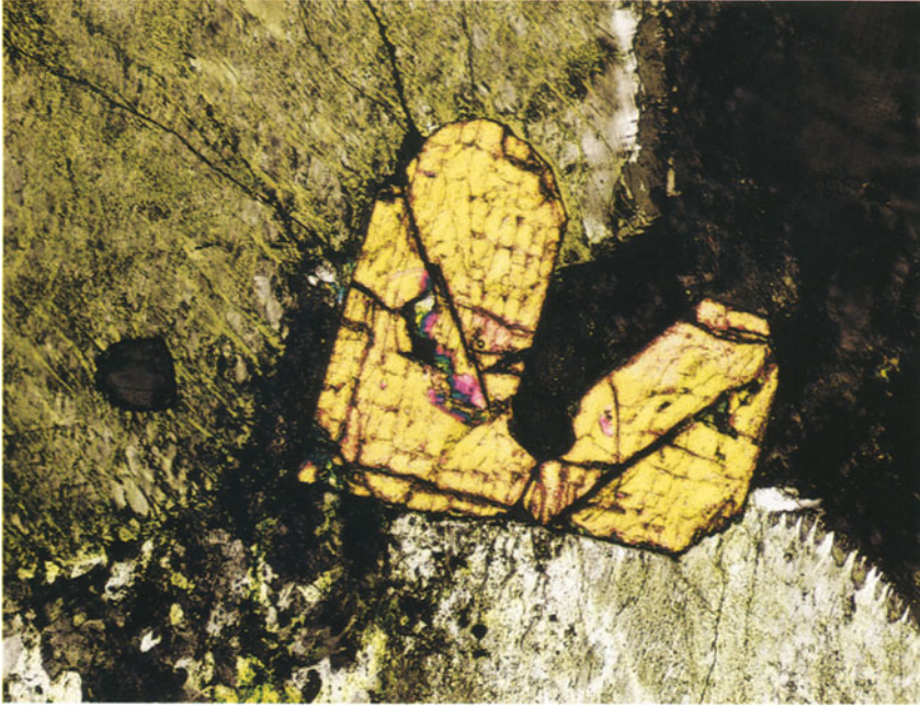
3 Zircon forming an idiomorphic crystal which has crystallized early from the magma. It shows bright-yellow to blue interference colours of the 2nd order, weak cleavage and sharply defined fractures. It is surrounded by microcline-perthite (grey to white interference colours of the 1st order), spindles are mostly sericitized (brown); nepheline shows grey-black to grey interference colours of the 1st order, and apatite (inclusion in microcline-perthite; section is nearly perpendicular to the optic axis, therefore almost isotropic). Nepheline syenite. Laugen valley in southern Norway. Crossed polars, 2.2 \times 3.1 mm.
