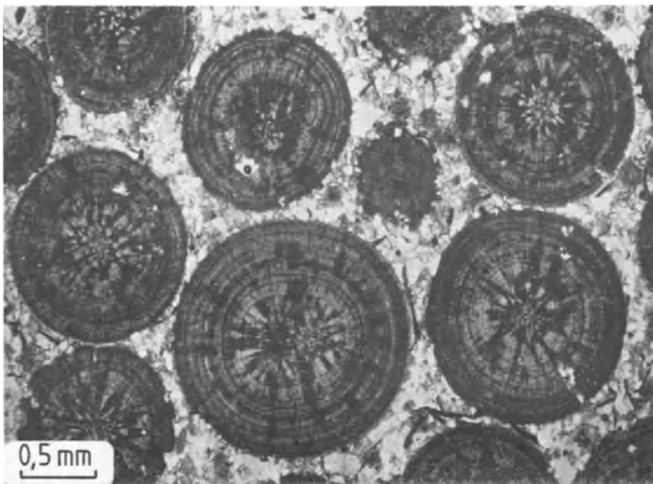
Fig. 247 Aragonite spherulite (peastone) in a fine-grained carbonaceous sinter deposit (pisolite). Carlsbad, Germany. Uncrossed polarizers.
