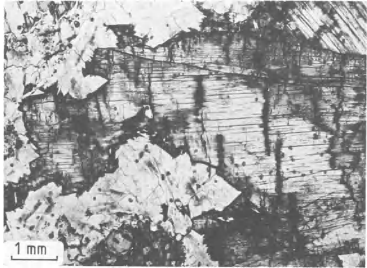
Fig. 205 Laumontite showing red coloration along its rims and fractures; characteristic cleavage. Cavity in leucite tephrite. Vesuvius volcano, Italy. Uncrossed polarizers.
