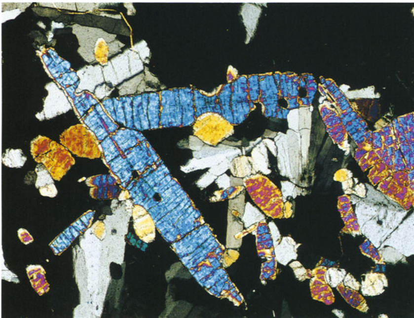
6 Short to long prisms of cancrinite phenocrysts, showing well-developed cleavage and interference colours of the 1st order (straw-yellow) and 2nd order (blue). Accompanied by alkali feldspar, apatite and ore. Foyaite-syenite ejecta. Laacher volcanic area, Germany. Crossed polars, 2.4 \times 3.2 mm.
