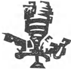
Fig. 33 Skeletal ilmenite crystal showing leucoxene alteration (white parts in the crystal).
