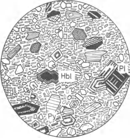
Fig. 263 Microcrystalline-porphyric texture. Very common in volcanic rocks. Phenocrysts of at least two generations are embedded in a matrix comprised of microlites and glass (dacite).
