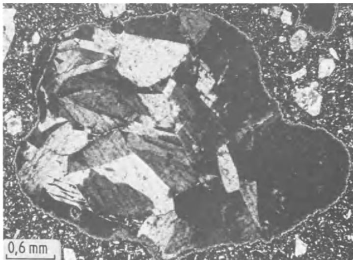
Fig. 58 Paramorphous analcite filling an amygdale in an alkaline hawaiite. Cyclope Islands near Catania, Sicily. Crossed polars.
