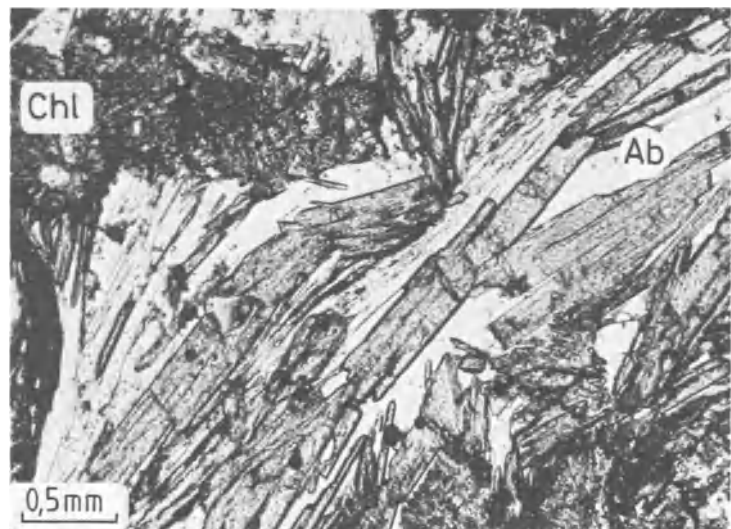
Fig. 238 Columnar chloritoid together with albite and chlorite. Albite-chlorite-chloritoid schists. Baños, eastern Cordillera, Ecuador. Uncrossed polarizers.
