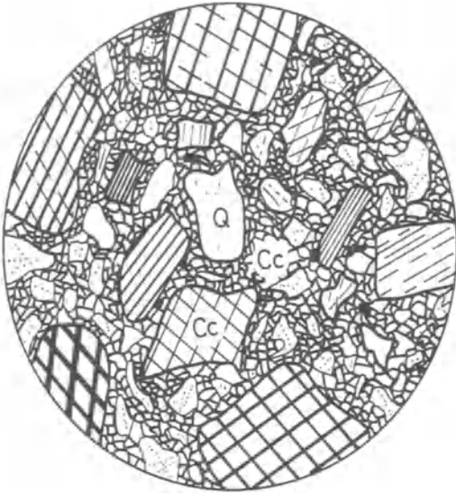
Fig. 280 Pseudosparitic-cataclastic texture with angular quartz and calcite phenocryst fragments in a carbonate cement.
