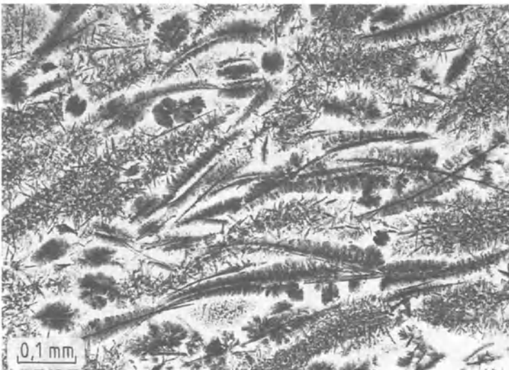
Fig. 68 Fern-like devitrification microlites (green hornblende?) in a Tertiary largely devitrified glass. Arran Island, Scotland. Uncrossed polarizers.
