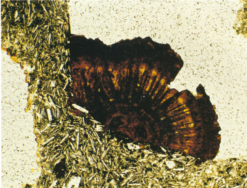
1 Spheroidal hematite, coloured red-brown, filling cavities in a microcrystalline matrix comprised of plagioclase, pyroxene and rock-glass. Pyroxene andesite. Mojanda volcano, northern Ecuador. Uncrossed polarizers, 1.4 × 2.0mm.
