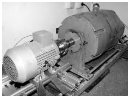
Figure 14.3 Laboratory test rig with IM and DC motor load
