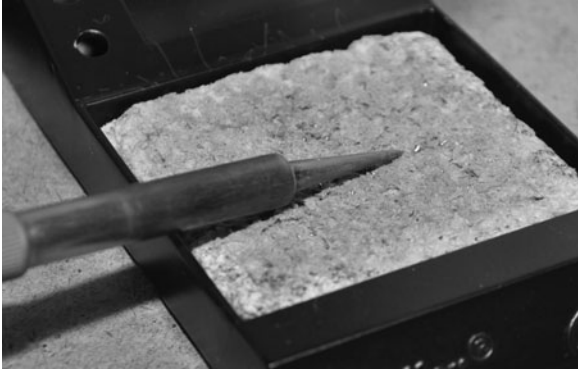
Figure 1-20 Drag the tip with a turning motion to clean off the old solder blobs.
