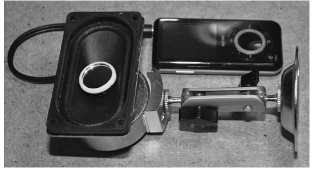
Figure 16-5 Creating an easy-to-align speaker base.
