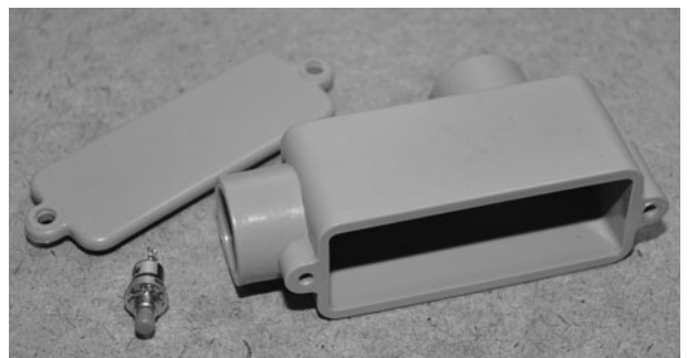
Figure 19-25 A PVC wiring box makes a for a strong enclosure.
