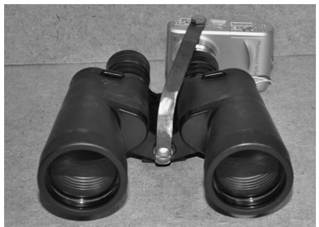
Figure 25-14 The metal flat bar holds the camera over the right eyepiece in perfect alignment.
