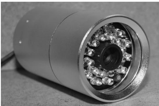
Figure 2-9 An outdoor security camera with built-in night vision LEDs.
