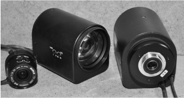
Figure 2-6 C-type lenses offer the highest quality and range of features.
