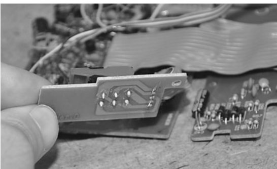
Figure 13-6 Identifying the receiver hook switch to decode the wiring.
