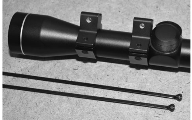
Figure 8-18 Modifying the rifle mounts to hold the laser in place.
