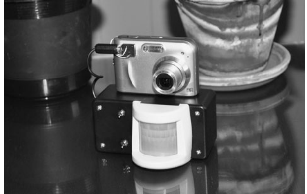
Figure 24-19 The motion-activated camera waiting for the next victim to set it off.
