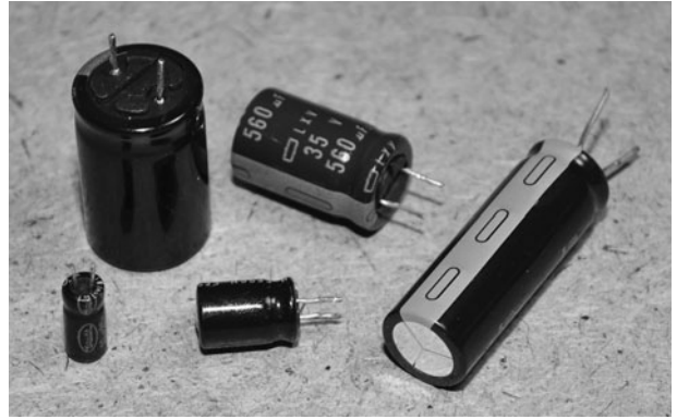
Figure 22-4 Various capacitor values we tried in order to control the frame rate.
