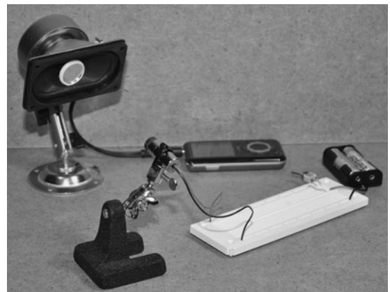
Figure 16-9 Setting up the laser and speaker on a test bench.
