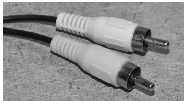
Figure 2-10 This is the most common type of composite video connector.
