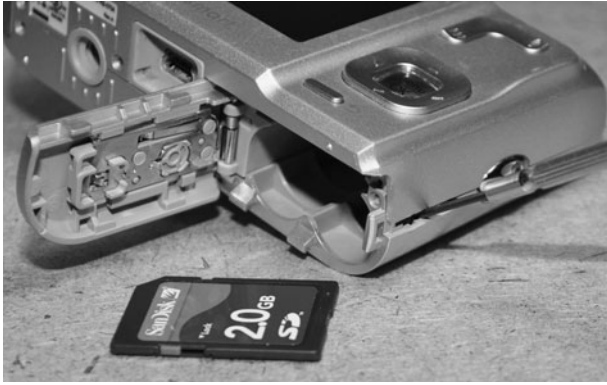
Figure 21-4 The plastic casing will usually be snapped together from the inside.
