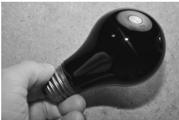
Figure 4-19 This black light is a plug-and-play illumination source for video cameras.
