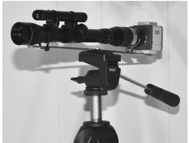
Figure 8-24 The completed long-range laser illuminator and camera zoom system.
