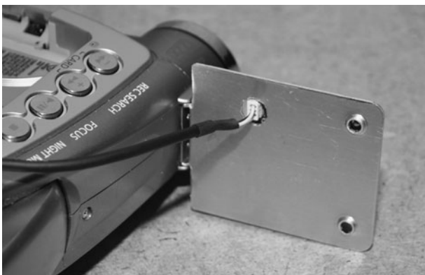
Figure 9-20 This small spy camera uses a tiny connecting plug on the back.
