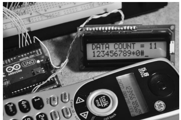
Figure 11-11 Decoding DTMF tones from the phone and displaying them on the LCD screen.
