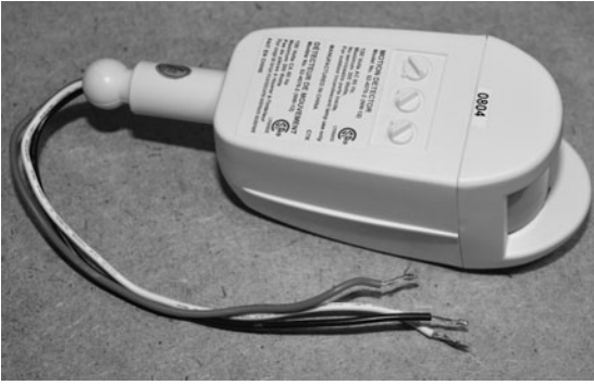
Figure 24-2 Only the motion-sensor part of the security light is needed for this project.
