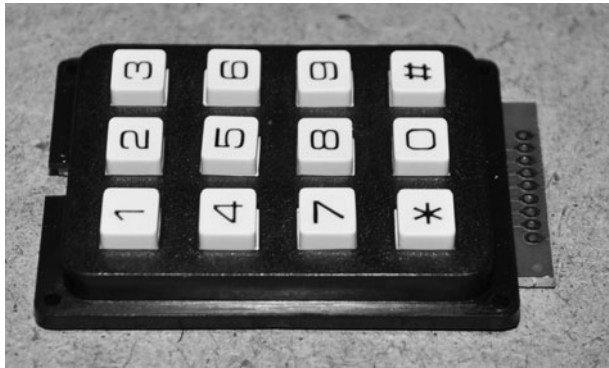
Figure 20-1 Arming and disarming the alarm is done by entering a code on a keypad.
