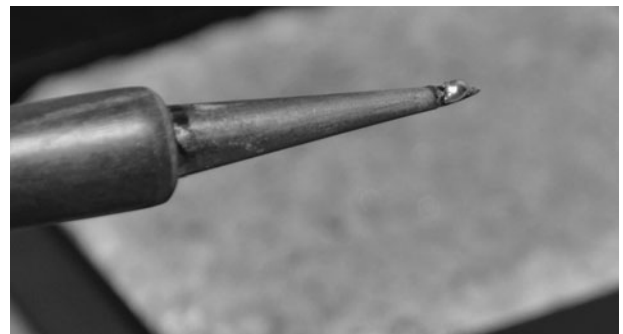
Figure 1-19 Old solder will build up on the tip of the soldering iron as it is used.
