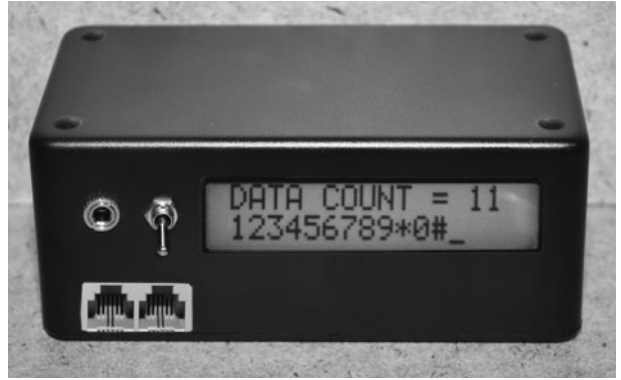
Figure 11-12 The completed DTMF decoder accepts both a phone cord and an audio input.
