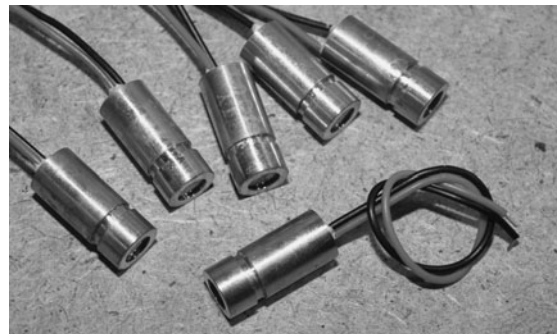
Figure 8-2 Laser modules are often higher quality and include adjustable optics.
