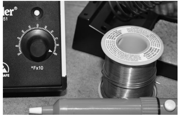
Figure 1-2 A higher heat setting is best for unsoldering larger components.
