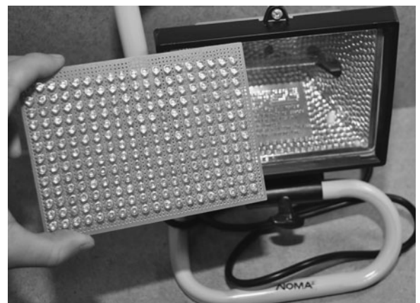
Figure 6-8 The completed 18 \times 13 LED array will be installed into the light cabinet.
