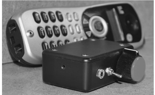
Figure 12-11 This version of the spammer jammer has direct audio and a phone interface.
