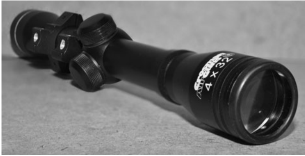
Figure 25-4 This 3× optical zoom gun sight can be used as a makeshift camera lens.
