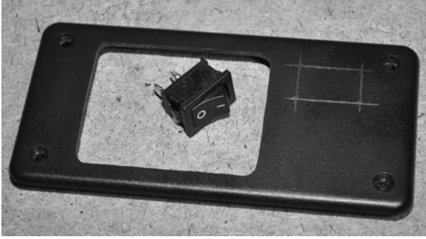
Figure 20-24 Adding the master power switch to the system.
