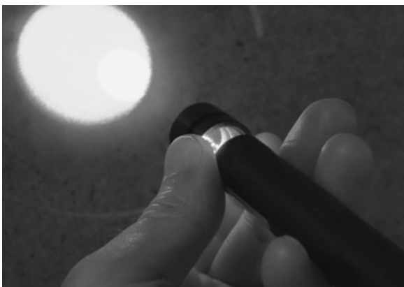
Figure 8-12 The beam spread out to 6 in at a distance of 10 ft.
