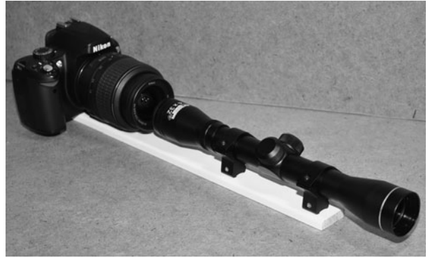
Figure 25-7 Making a solid base to align the optical device to the camera lens.
