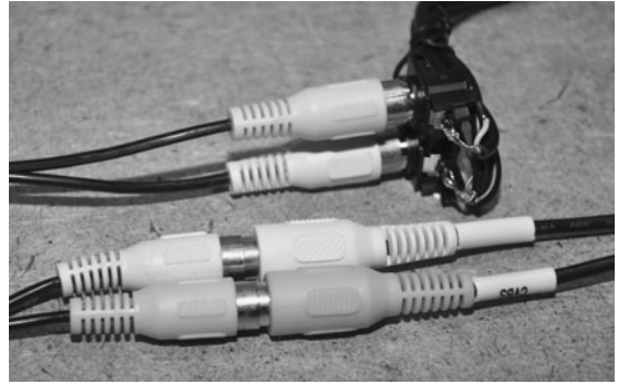
Figure 9-9 This is the most common type of composite video connector.
