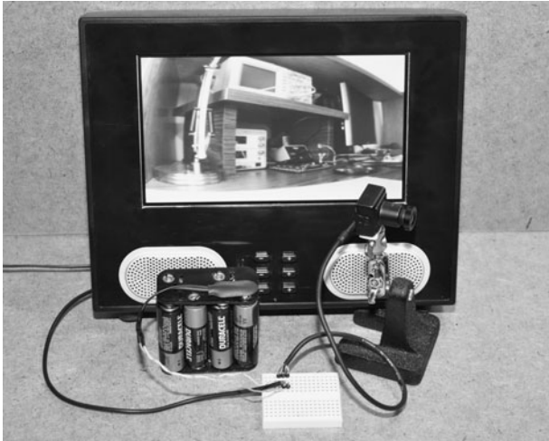
Figure 3-12 The camera is connected to a portable composite video LCD monitor.
