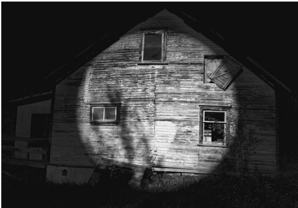
Figure 8-25 From 100-ft away, the camera can see clearly using the laser illuminator.
