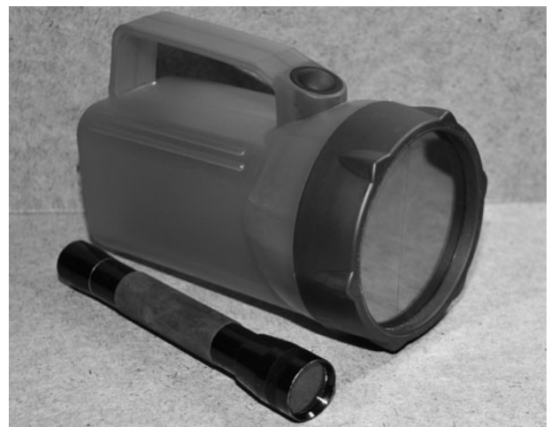
Figure 3-20 This infrared illuminator converts white light into infrared light.
