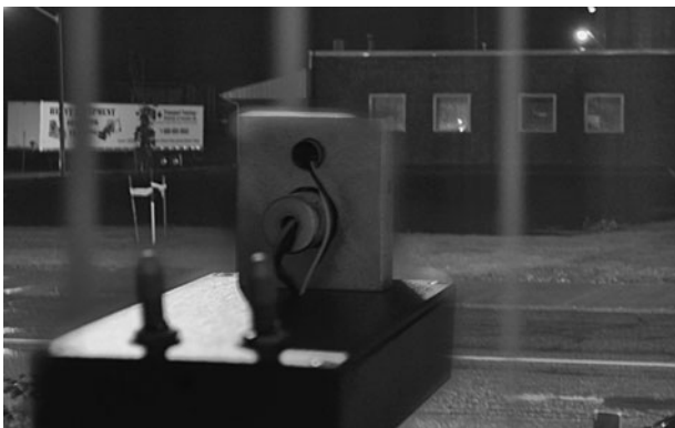
Figure 16-33 Beaming a window across the street in a controlled test.
