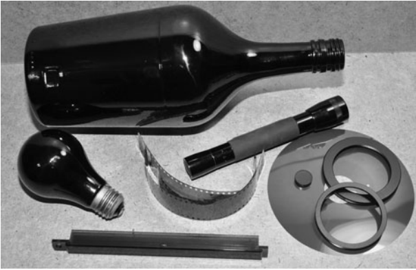
Figure 3-10 Infrared passing filters can be made from many different materials.
