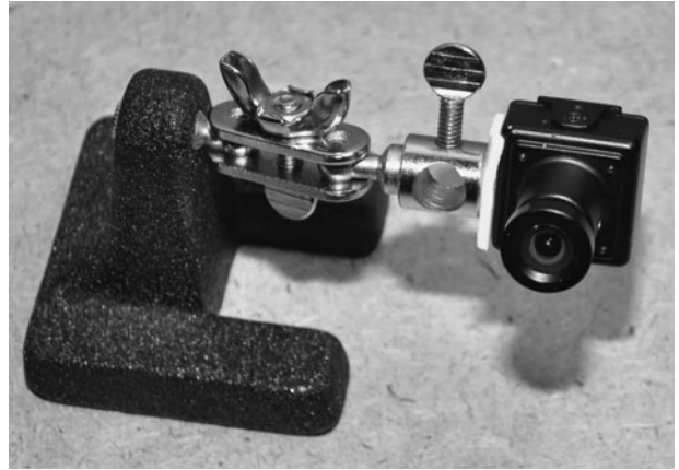
Figure 3-11 This small black and white spy cam will be used to view the infrared light.
