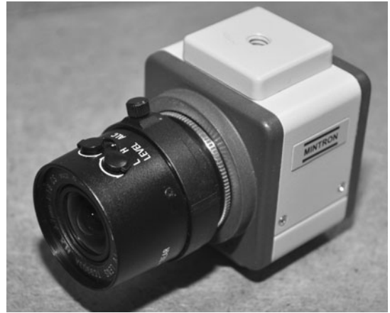
Figure 8-21 Most security cameras can see infrared radiation as white visible light.
