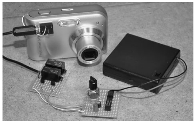
Figure 23-9 The completed sound activation system on small circuit board.
