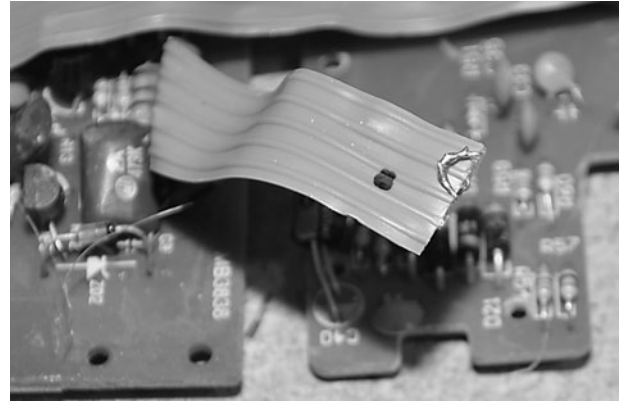
Figure 13-10 Soldering the hook switch points together to fix the phone on the hook.
