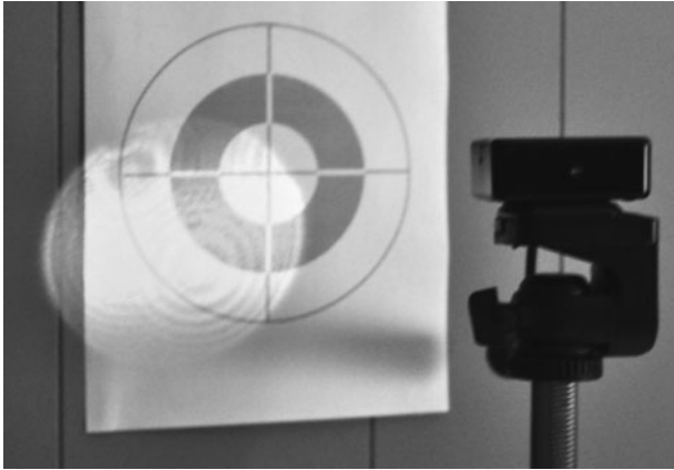
Figure 16-31 The return laser beam will no longer be a tiny spot on the wall.
