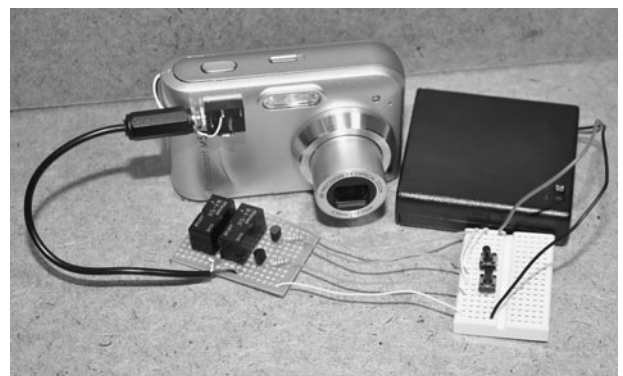
Figure 21-24 Testing the completed relay controller using manual pushbutton switches.
