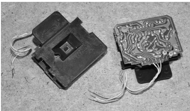
Figure 24-15 Reducing the sensor board to their absolute minimal configuration.
