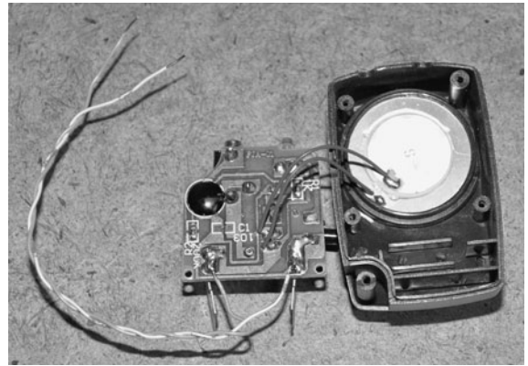
Figure 20-12 Replacing the internal batteries with a pair of wires.
