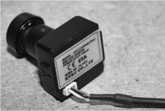
Figure 2-15 The board camera- and micro camera-style connector.
