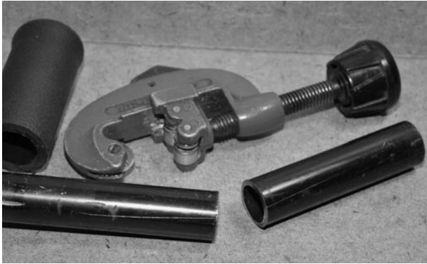
Figure 19-26 Making a pistol grip from some bicycle handlebar parts.
