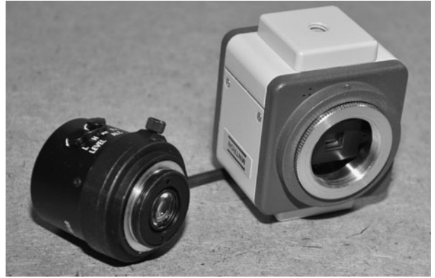
Figure 2-3 Large cameras with removable lenses have C or CS mounts.
