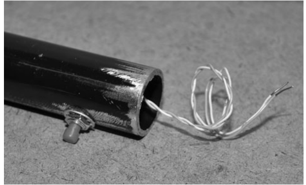
Figure 19-28 The pushbutton trigger switch installed.
