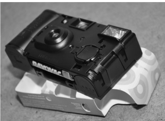
Figure 19-2 Remove the plastic or paper branding cover.
