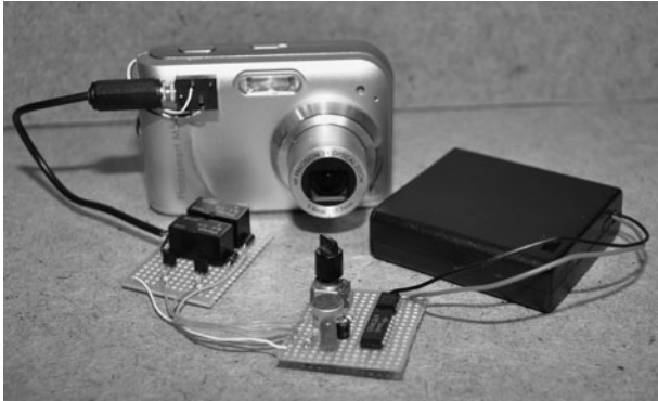
Figure 23-1 This is the relay interface that controls the camera shutter switch.
