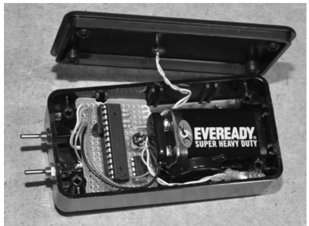
Figure 26-14 Fitting all of the parts in the box one last time.
