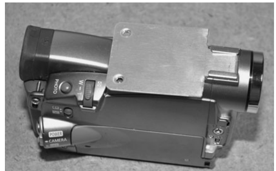
Figure 9-14 The tab is cut and fits snugly into the light mounting slot.
