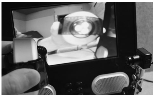
Figure 4-7 White LEDs were tested but failed to produce enough infrared light.
