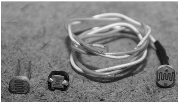
Figure 16-7 A photoresistor will respond to a change in light.
