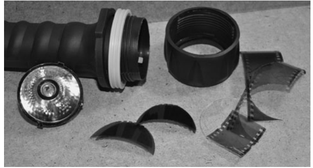
Figure 4-14 Creating a similar infrared beam flashlight using the camera film.
