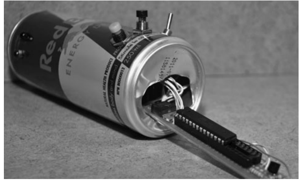
Figure 18-21 Installing the circuit board after the wiring is completed.
