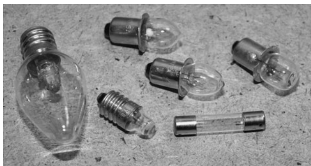
Figure 4-8 The light given off by an incandescent flashlight bulb is high in infrared.
