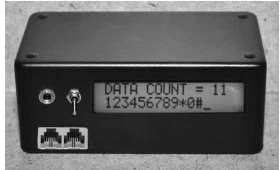
Figure 11-0 This device will decode the DTMF tones from the phone line or audio source.
