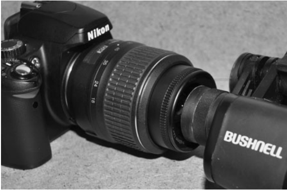
Figure 25-6 The binocular eyepieces need to be closer to the lens than the gun sight.
