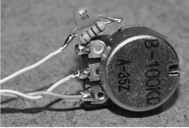
Figure 16-19 Keeping components close to the source reduces noise.
