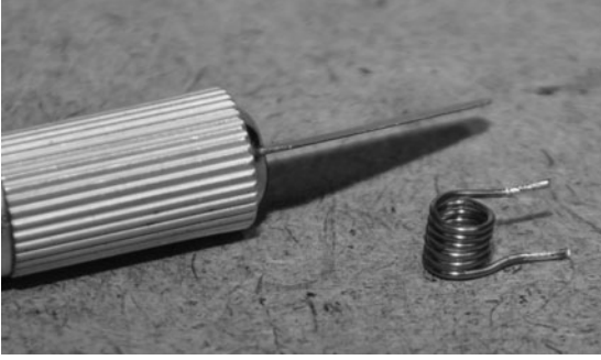
Figure 17-6 The enamel needs to be scraped from the end of the coil.
