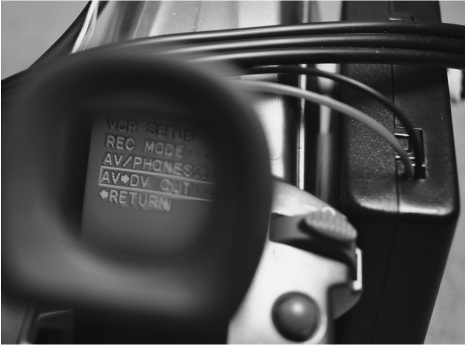
Figure 9-23 Setting up the camera to use the external camera as an input.
