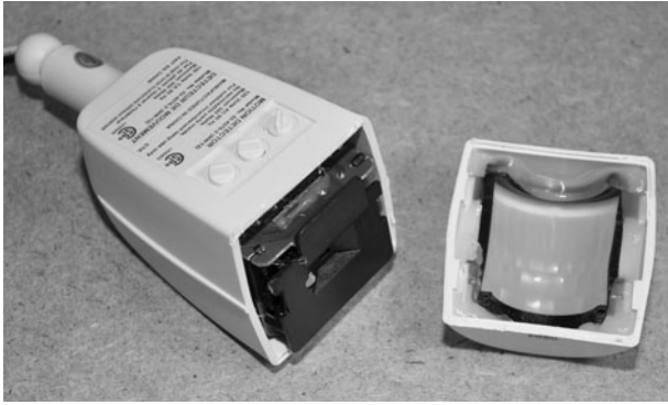
Figure 24-5 The two halves open up to reveal the circuit board inside.
