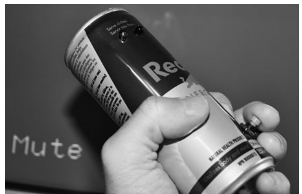
Figure 18-25 Playing back the mute command to the TV after a successful intercept.
