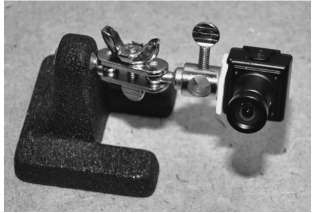
Figure 7-8 A small monochrome video camera will be used to detect the infrared light.
