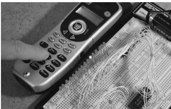
Figure 11-8 Testing the 16 LED DTMF decoder system using the telephone dial pad.
