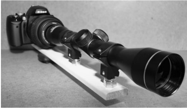
Figure 25-12 The completed gun-sight adapter sitting on the tripod mounting platform.
