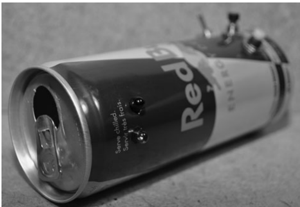
Figure 18-20 Installation of the infrared components.
