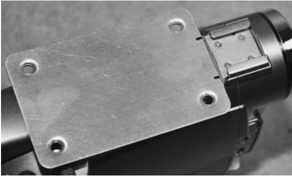
Figure 9-11 Marking the aluminum plate to cut the new slot.
