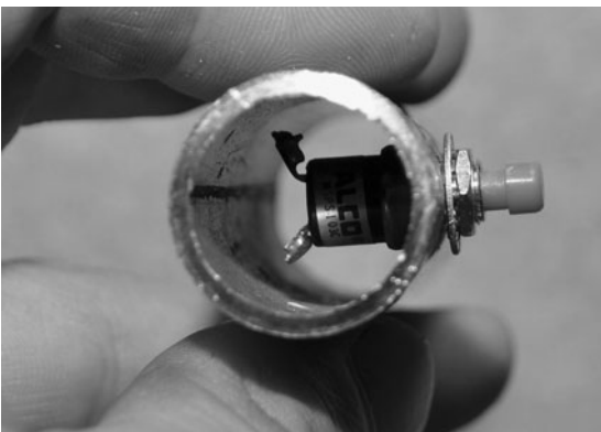
Figure 19-27 Fitting the trigger switch into the hand grip tubing.
