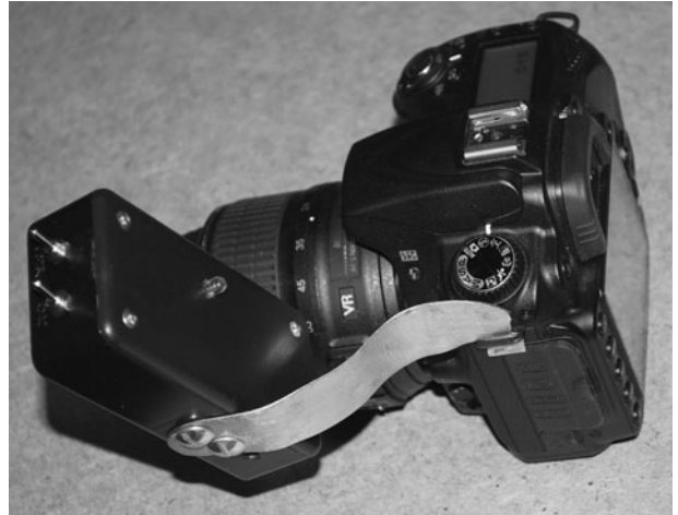
Figure 26-19 The mounting hook just drops into the strap clip.
