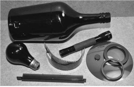
Figure 4-1 Infrared pass filters can be made from many different materials.
