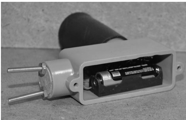
Figure 19-34 The completed circuit board and battery installation.
