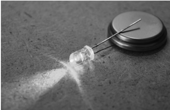
Figure 3-5 A 3-V coin battery becomes a universal LED tester.
