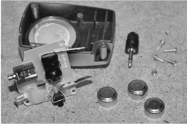
Figure 20-11 Converting the pocket alarm for relay operation.
