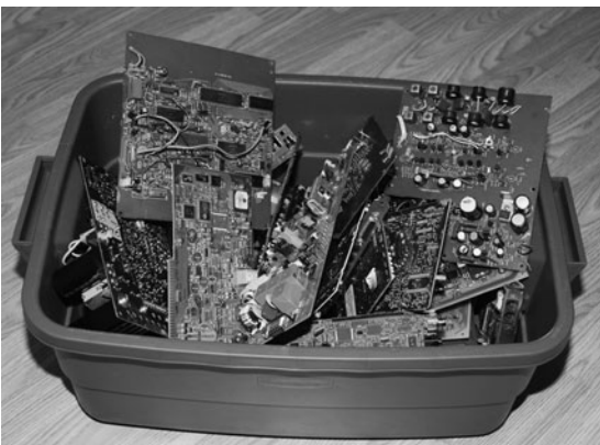
Figure 1-0 Most of your parts inventory can be salvaged from old circuit boards.
