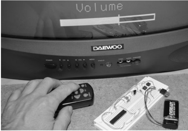
Figure 18-9 Initial testing of the prototype project (record).
