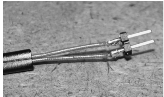
Figure 12-2 Only the two center wires are used in most residential phone systems.
