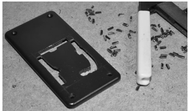
Figure 20-6 Cutting the rectangular opening one nibble at a time.
