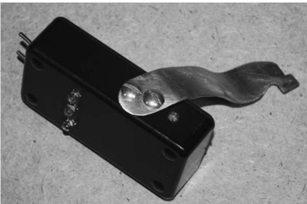
Figure 26-18 The mounting hook is bolted to the project box.
