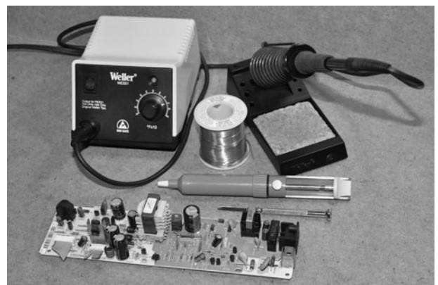
Figure 1-1 The basic tools you will require for any soldering or unsoldering work.
