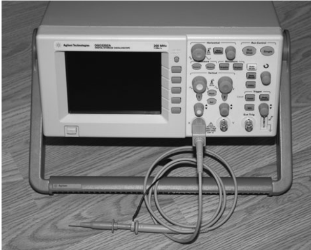
Figure 0-25 An oscilloscope for more advanced work.
