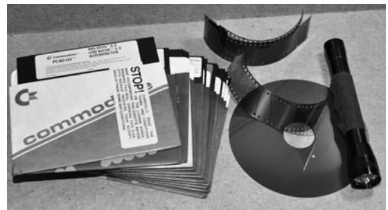
Figure 4-5 Developed film and floppy disk material can be made into infrared pass filters.
