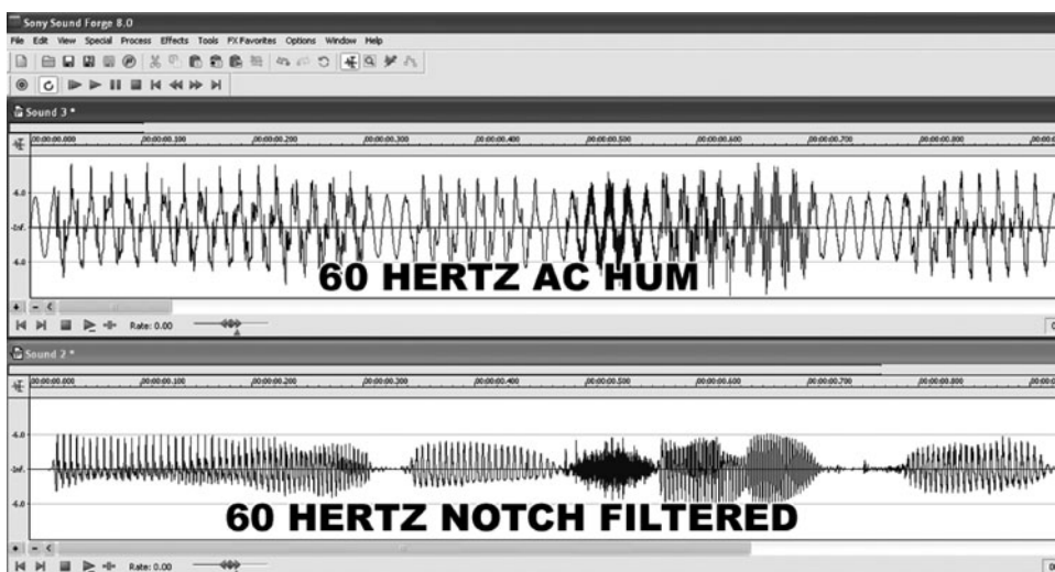
Figure 16-30 Computer software will do wonders for a noisy audio signal.
