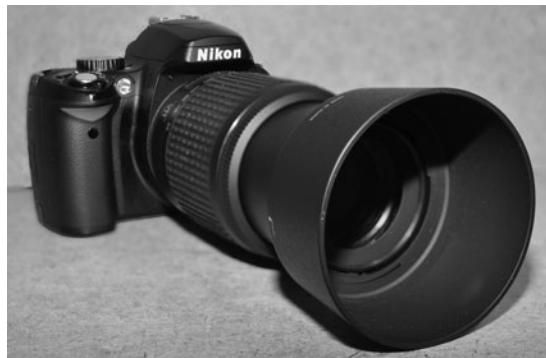
Figure 25-3 This telephoto lens will fit onto any Nikon SLR camera body.
