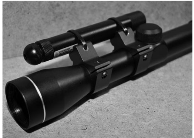
Figure 8-19 The laser tube is held in place by the rifle mounting brackets.
