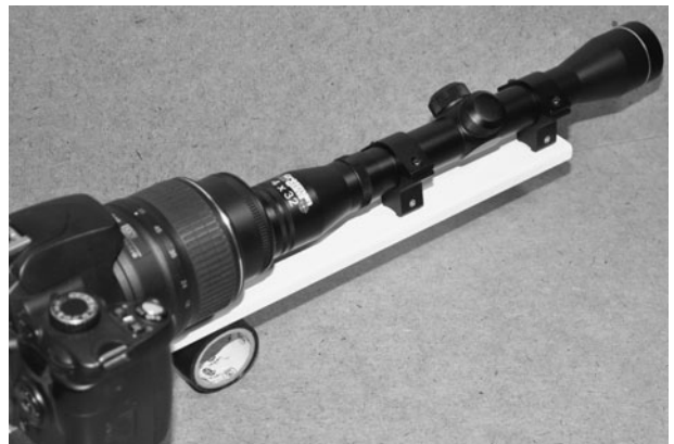
Figure 25-11 Finding the center of balance with both devices mounted to the base.
