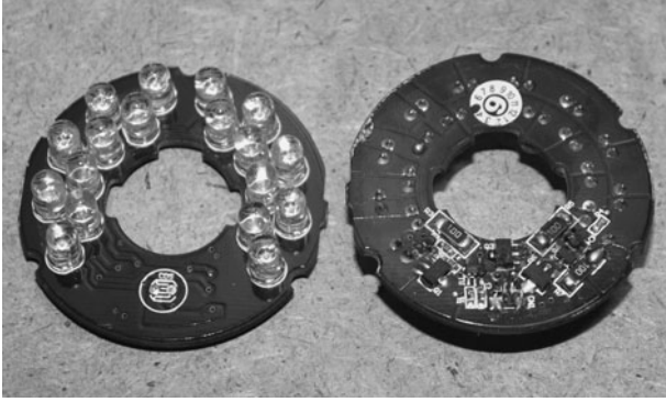
Figure 7-1 This is a pulsed-mode illuminator taken from an outdoor security camera.
