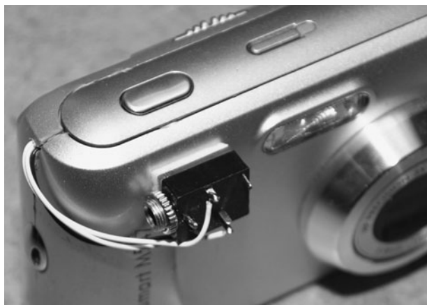
Figure 21-16 The female connector is affixed to the body of the camera.
