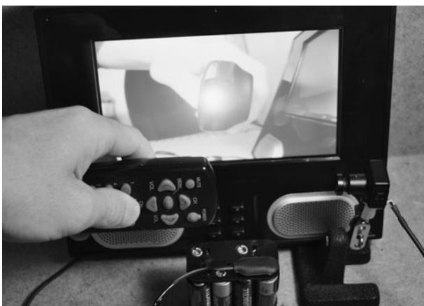
Figure 3-13 Testing the camera response using a television remote control.
