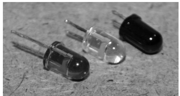
Figure 5-2 Infrared LEDs are available with various lens types and wavelengths.
