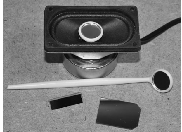
Figure 16-3 Add a reflective surface to the center of the speaker.
