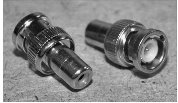
Figure 2-13 Adapting the BNC connector to the RCA-style connector.
