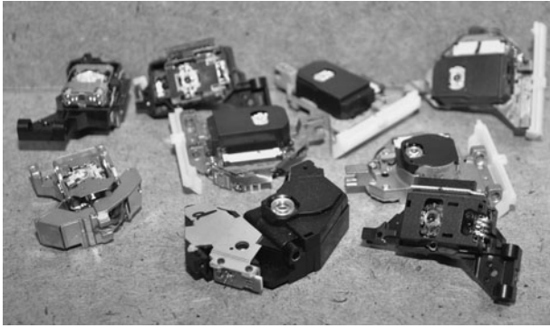
Figure 8-3 DVD and CD burners are a great source of high-power laser diodes.
