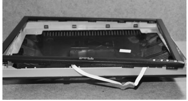
Figure 6-18 Removing the front bezel and the broken LCD panel from the monitor.
