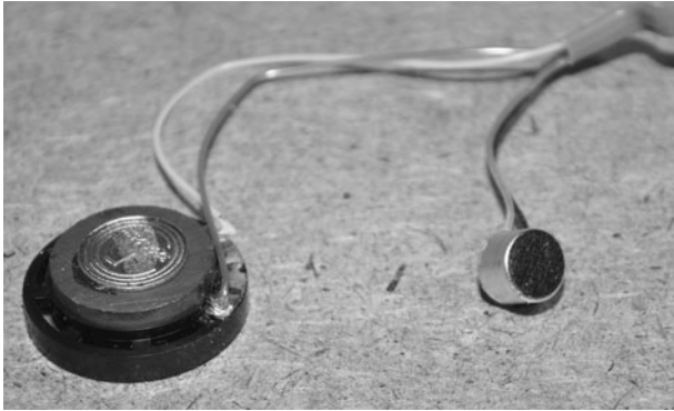
Figure 13-13 The electret microphone and speaker from the original handset.
