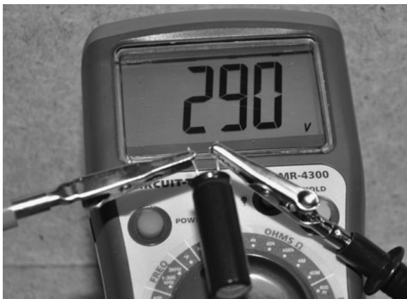
Figure 19-9 The little capacitor has more voltage than your wall outlet!
