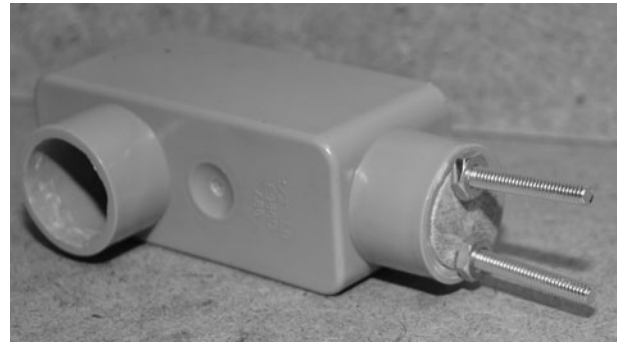
Figure 19-31 The high-voltage probes are just long bolts.
