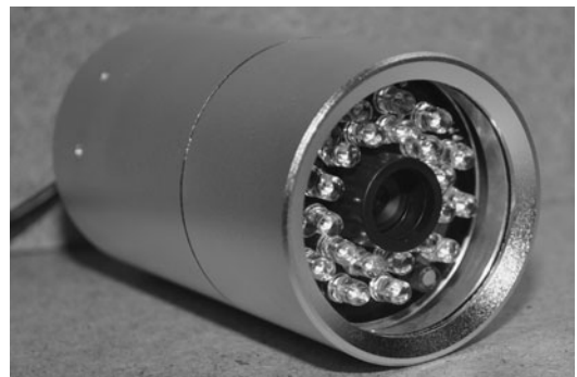
Figure 9-7 An outdoor security camera with built-in night vision LEDs.
