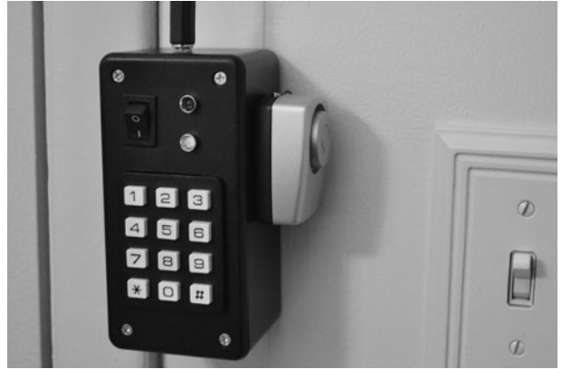
Figure 20-0 This security system works as both a permanent or portable alarm.
