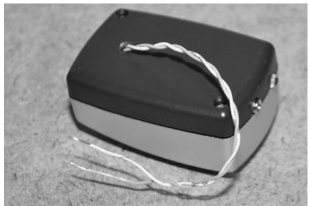
Figure 20-13 The completed externally powered pocket alarm.
