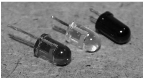
Figure 3-2 Infrared LEDs are commonly used in remote control applications.
