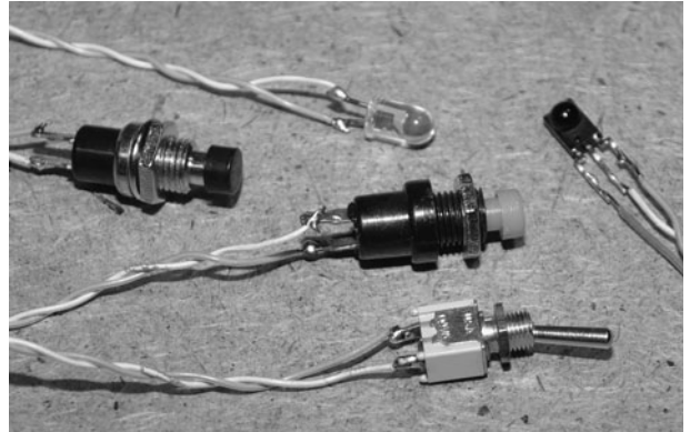
Figure 18-17 Wiring all of the external components and switches.
