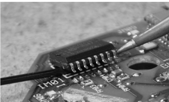
Figure 1-25 One side of the surface-mounted IC has lifted from the pads.
