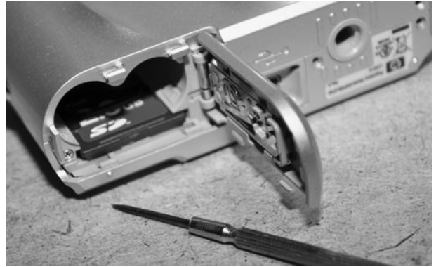
Figure 21-3 Often, the screws will be hidden behind doors or under labels.
