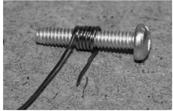
Figure 17-4 Wrap the bolt five times and you now have your RF coil.
