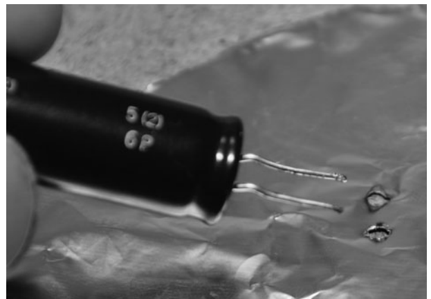
Figure 19-10 Tinfoil is no match for the capacitor’s 360-angry volts (V).
