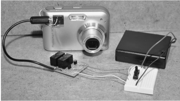
Figure 22-1 This is the relay interface that controls the camera shutter switch.
