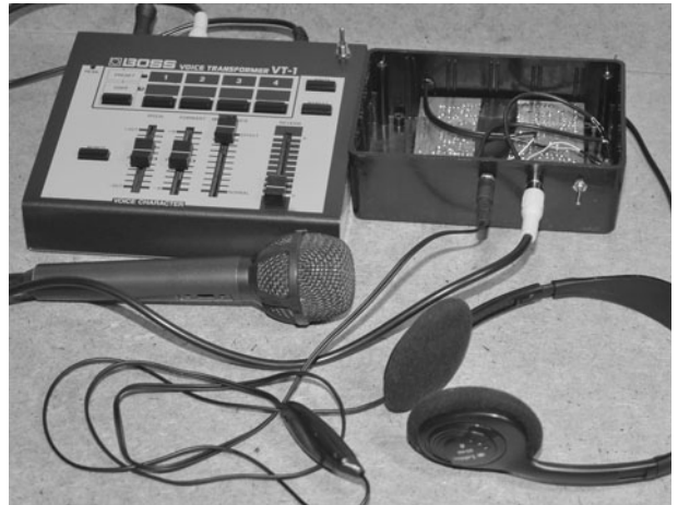
Figure 13-25 The completed telephone voice changer using the Boss Voice Transformer.
