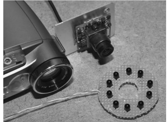
Figure 9-21 Infrared illumination will be provided by an LED ring light.
