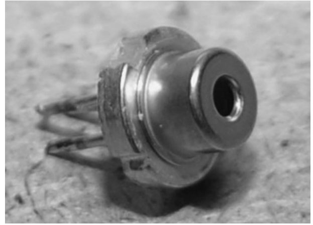
Figure 8-6 This is the bare 60-mW infrared laser diode from a CD burner.
