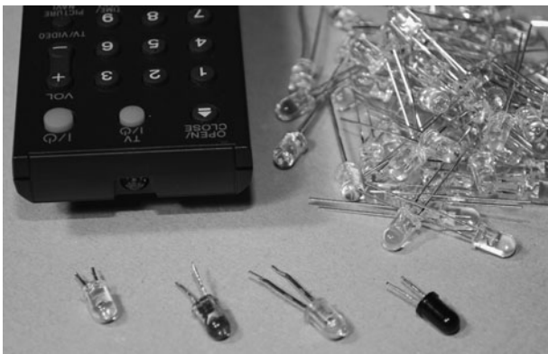
Figure 18-3 The pulses are sent to the appliance using an infrared LED.
