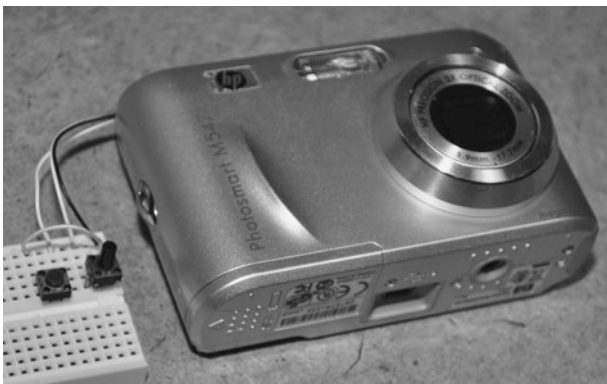
Figure 21-14 Once reassembled, the camera is tested using the breadboard and switches.
