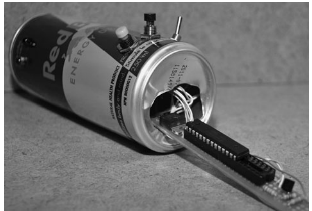
Figure 18-0 This hidden device can intercept remote control signals and play them back!
