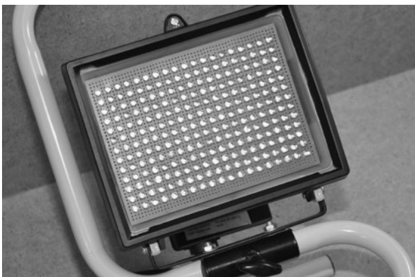
Figure 3-16 Using a large array of infrared LEDs to create a high-power illuminator.
