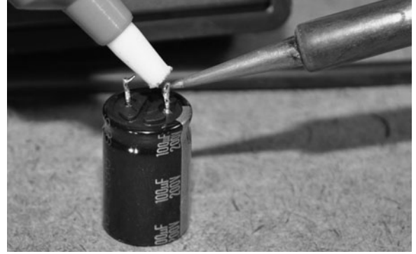
Figure 1-15 Clean the leads with the desoldering tool after removal.
