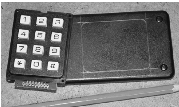
Figure 20-4 Marking the dimensions of the keypad for cutting.
