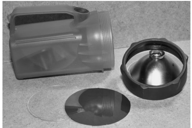
Figure 4-11 Making a larger more powerful illuminator using a flashlight.
