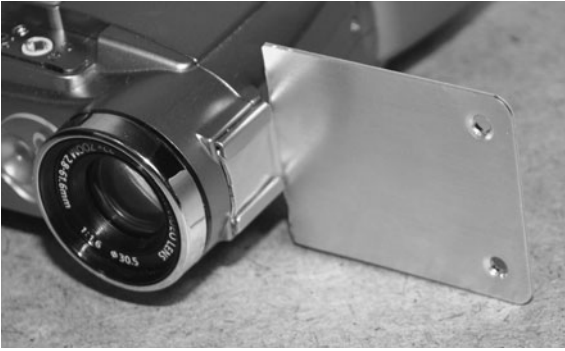
Figure 9-15 The aluminum part is bent into a 90 degree angle.
