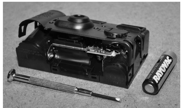
Figure 19-3 The camera shell will pry open into two halves.
