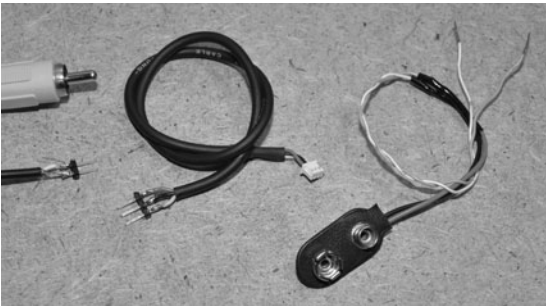
Figure 2-18 A complete set of breadboard-compatible cables for a micro camera.
