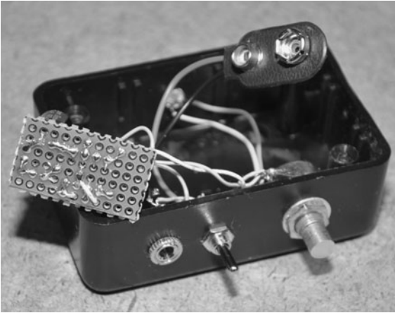
Figure 16-22 Installing the connecting wires to the circuit board.
