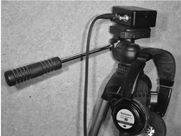
Figure 16-25 The tripod-mounted light-to-sound receiver.
