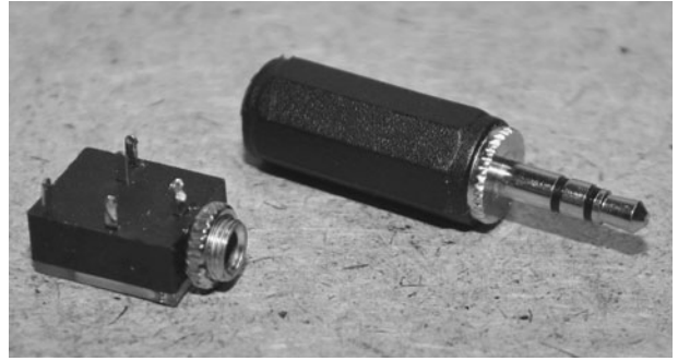
Figure 21-15 A three-conductor 1/8-in stereo jack will connect the camera to the device.
