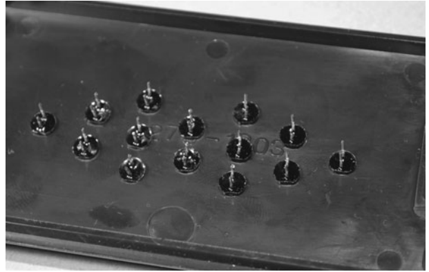
Figure 10-30 Install the LEDs in the same orientation.
