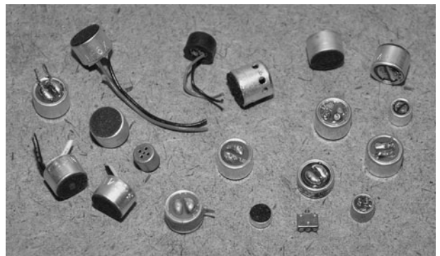
Figure 17-2 The electret microphone will drive the audio preamplifier stage.
