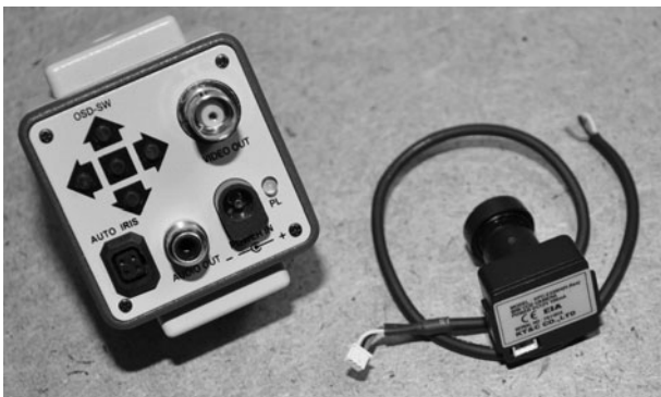
Figure 2-2 Camera connections for power, ground, and audio.
