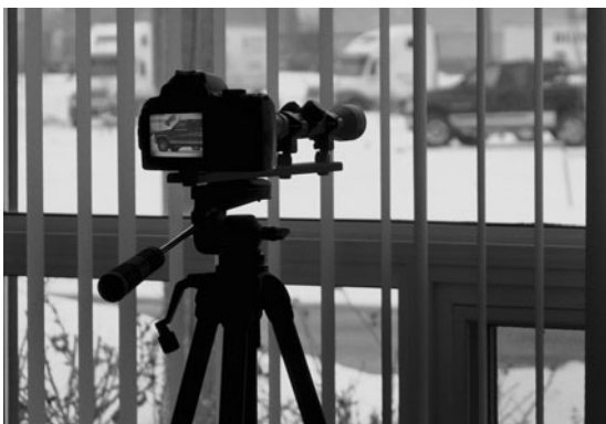
Figure 25-0 A digital camera can be adapted for ultra long range photography.
