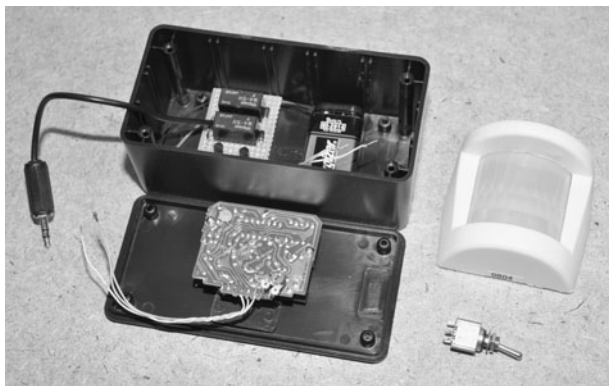
Figure 24-18 Creating a self-contained motion-sensing camera system.
