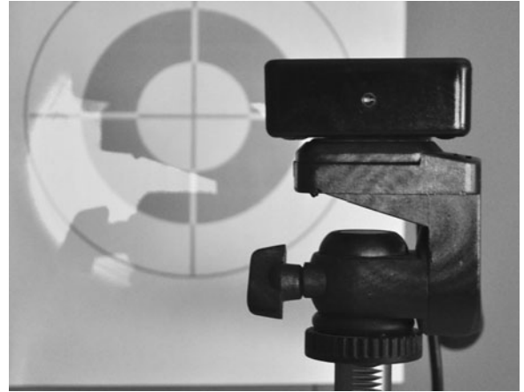
Figure 16-32 The edge of the beam is the optimal point for clear audio.
