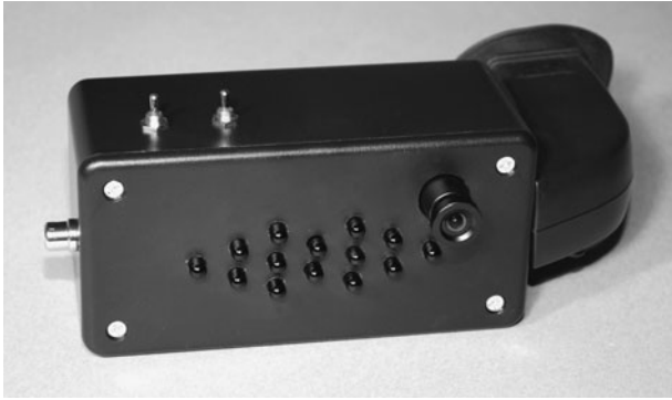
Figure 3-18 A portable night vision viewer made from an old camera viewfinder.
