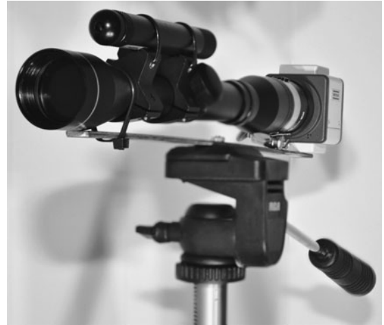
Figure 8-0 Build a long-range laser night vision illuminator.
