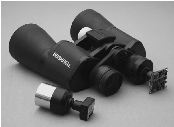
Figure 10-22 The lens cap makes a good camera mount.
