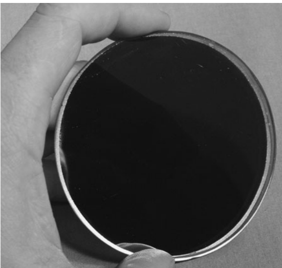
Figure 10-14 A 940-nm infrared pass filter glass.
