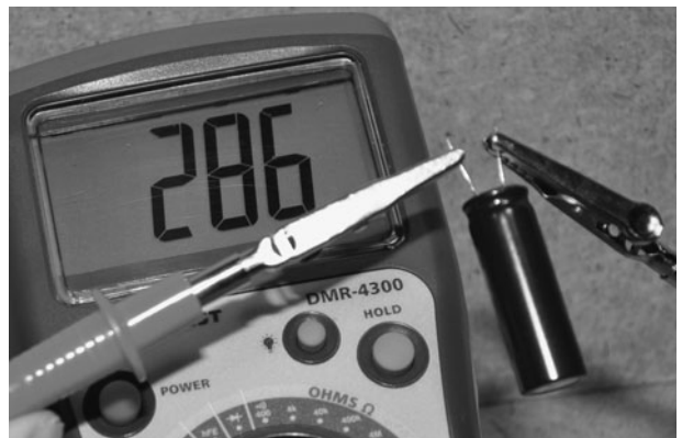
Figure 21-6 After more than 30 days, the capacitor still holds almost 300 V!
