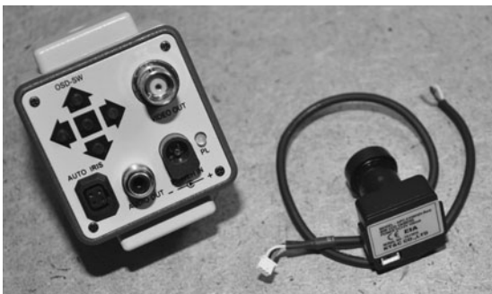
Figure 9-4 All video cameras will have connectors for power and video output.
