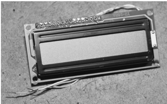
Figure 14-7 This is an easy to interface two-line serial LCD screen.
