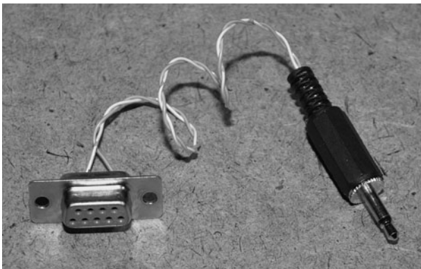
Figure 15-27 To retrieve the data, a 1/8 jack to 9-pin serial port cable is used.
