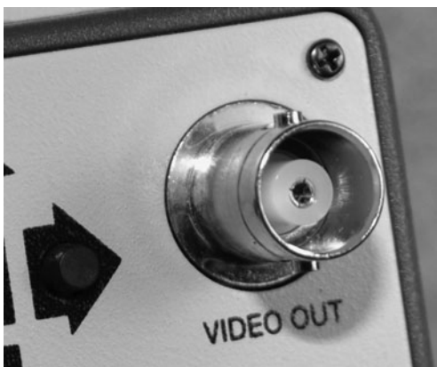
Figure 2-12 Some security cameras use a BNC-style video connector.
