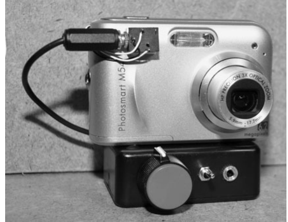
Figure 23-11 The completed sound-activated camera, waiting to spy on trespassers.
