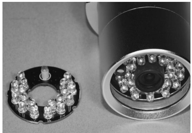
Figure 10-13 An alternative to individual LEDs.
