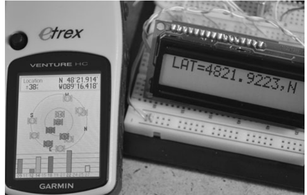
Figure 14-12 The GPS module and handheld GPS comparing latitude values.
