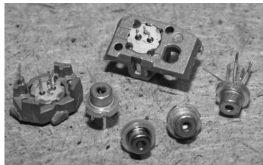
Figure 8-5 Several laser diodes removed from DVD and CD burner units.
