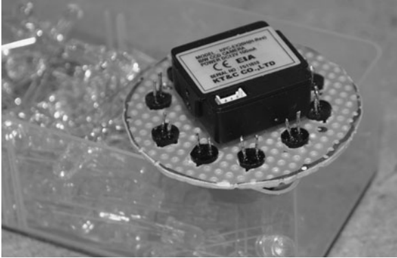
Figure 5-10 Checking the camera body and LED lead clearances.
