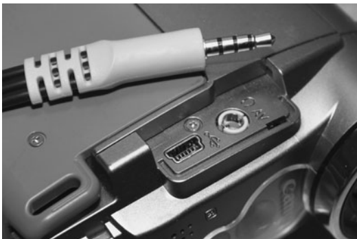
Figure 9-2 Our camcorder uses the 4-pin 1/8-in connector and is labeled AV.
