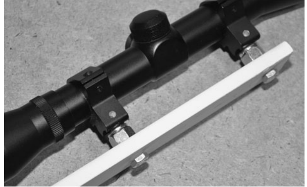
Figure 25-10 These bolts will lift the gun sight to the level of the camera lens.
