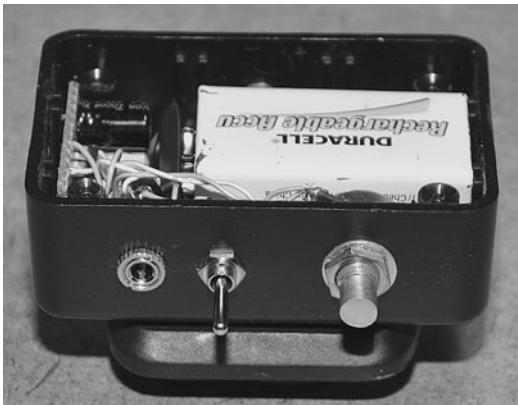
Figure 16-23 Fitting all of the hardware into the project box.
