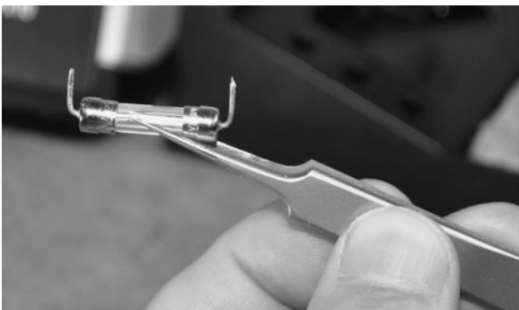
Figure 1-14 Leads are cleaned and straightened after removing a part.
