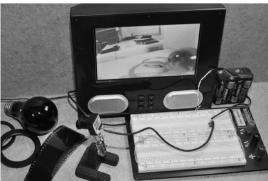
Figure 4-2 The test rig will consist of a low-lux video camera and small LCD monitor.
