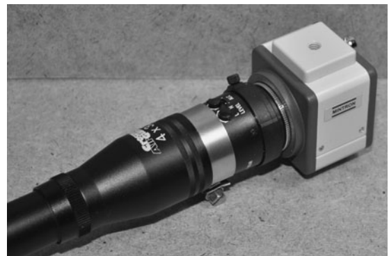
Figure 8-22 A steel clamp holds the C-mount camera lens directly to the gun sight.
