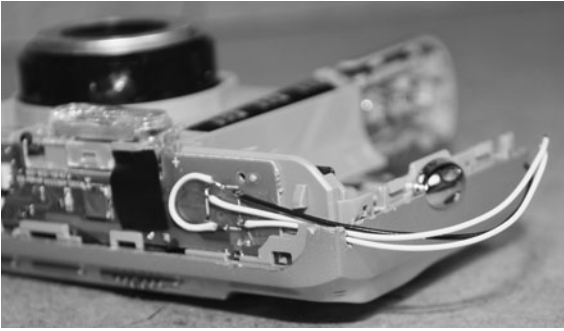
Figure 21-13 The wiring will be placed through a slot in the plastic casing.
