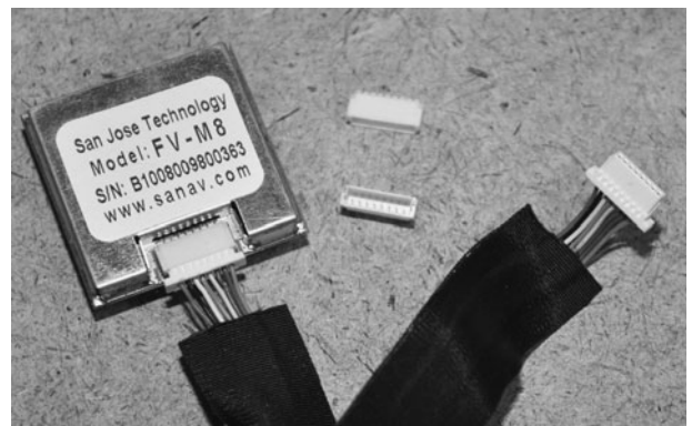
Figure 14-13 The GPS module came with a small 8-pin connector.
