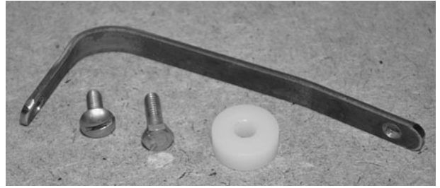
Figure 25-13 A piece of bent steel flatbar will be made into a binocular adapter.
