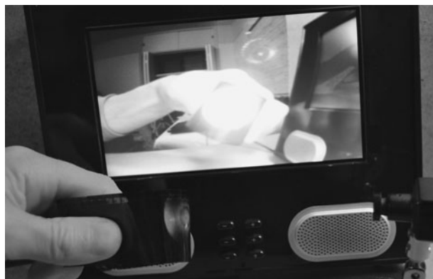
Figure 4-6 The camera film allows a lot of infrared light to pass through to the camera.
