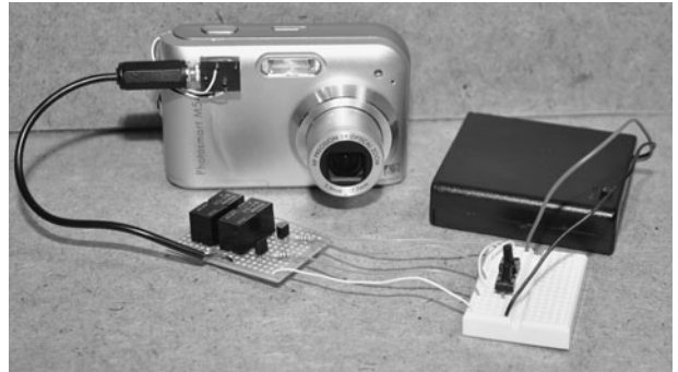
Figure 21-0 This external controller allows any device to control the shutter release.
