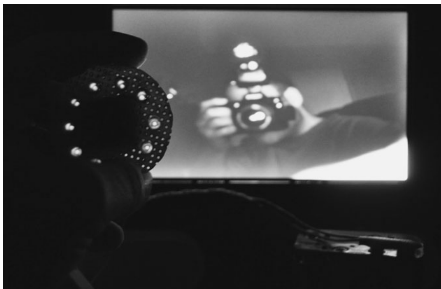
Figure 5-18 The infrared illuminator lights up our camera as we take this photo.
