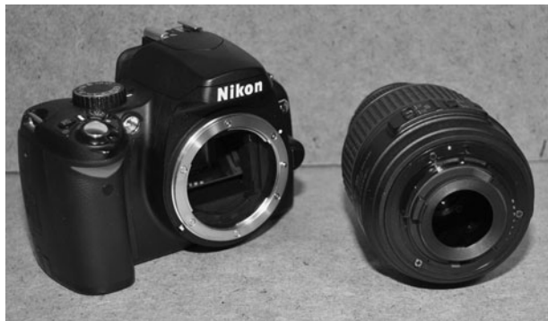
Figure 25-2 SLR digital cameras offer the ability to change the lenses.
