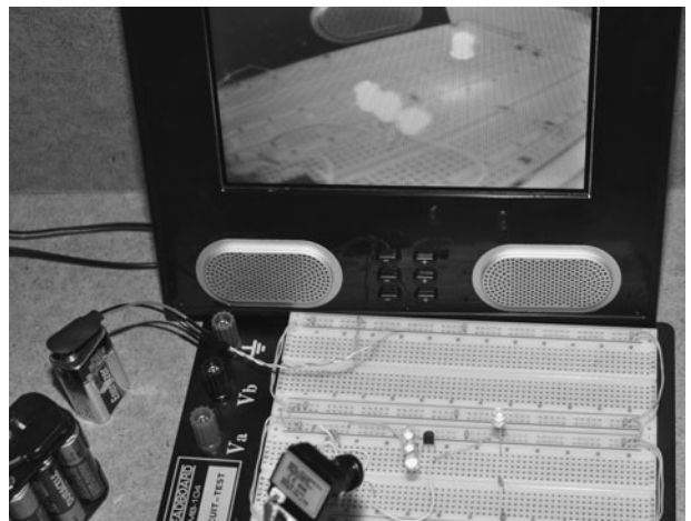
Figure 7-9 Testing the pulsing circuit with the camera and infrared LEDs.
