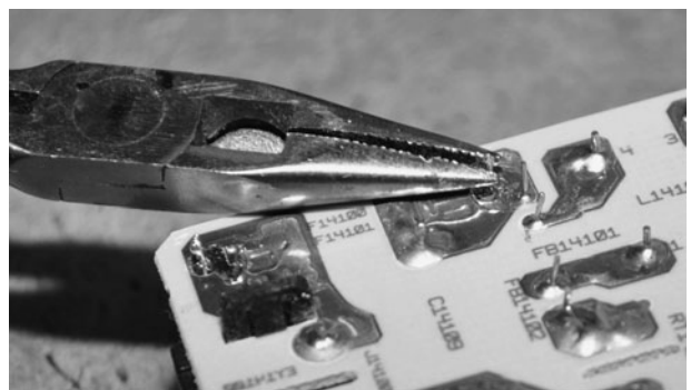
Figure 1-12 Sometimes the lead will be stuck to the side of the hole.
