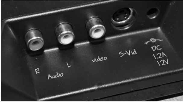
Figure 2-11 The back of a composite video monitor showing the RCA inputs.
