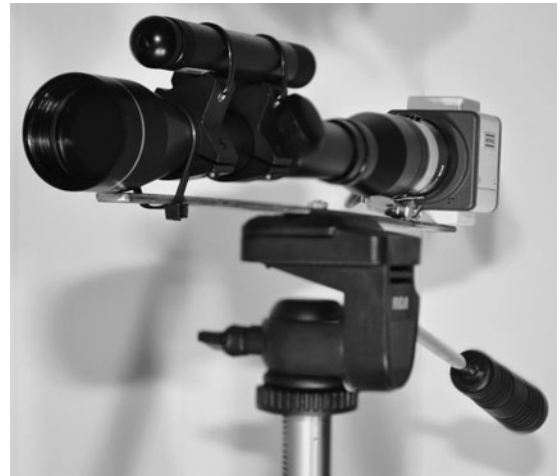
Figure 3-21 A long-range night vision system using a laser and optical magnification.
