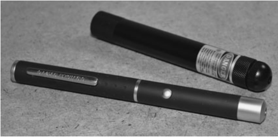
Figure 8-1 Laser pointers are now available that output infrared radiation.
