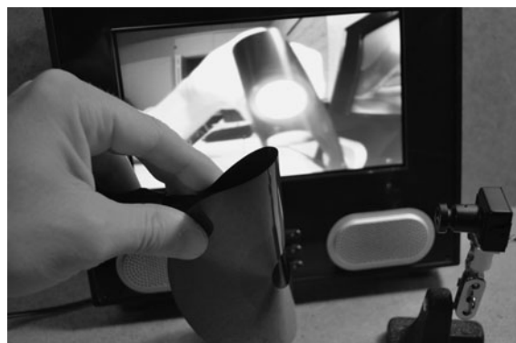
Figure 4-9 The disk material passes a good amount of infrared and blocks most visible light.
