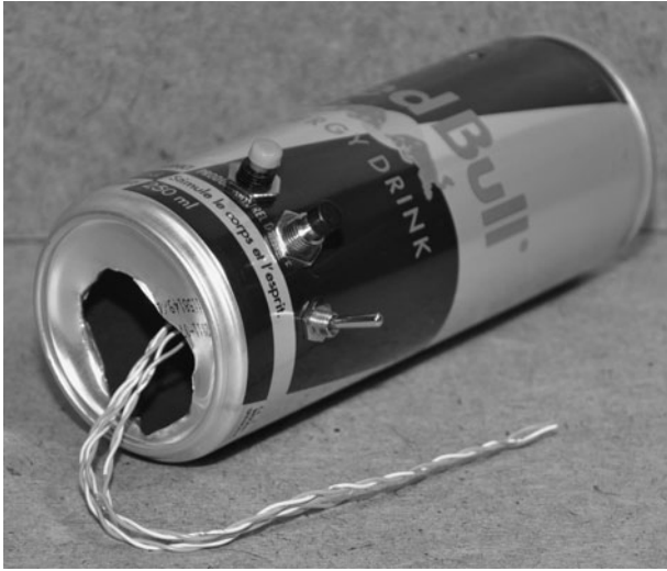
Figure 18-19 Making an opening for the battery and circuit board.
