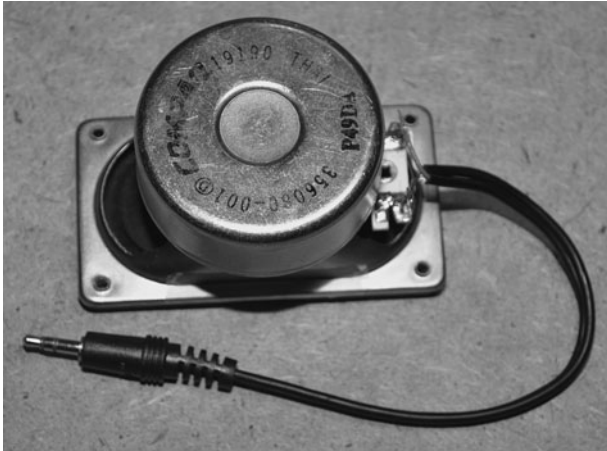
Figure 16-2 A small speaker will be used to simulate a vibrating window.
