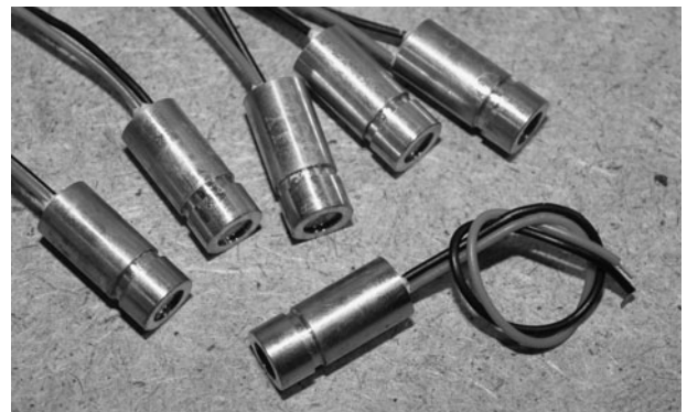
Figure 3-8 Laser modules are small and often include quality adjustable optics.
