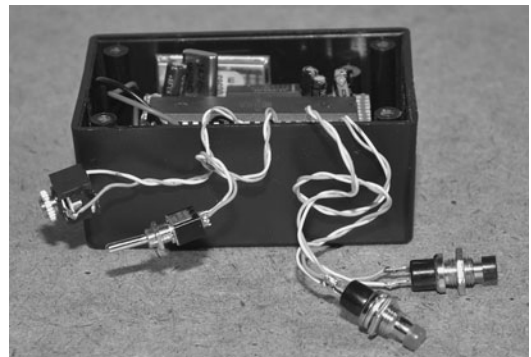
Figure 15-25 Fitting the circuit board and components into the small black box.
