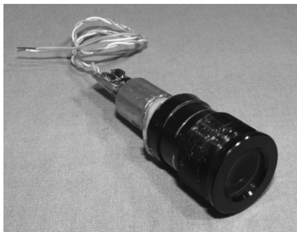
Figure 10-20 Beam spreading lens fit to the laser module.
