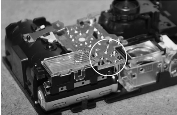
Figure 19-4 Identify the capacitor and its two output terminals.
