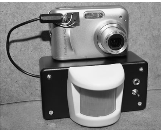
Figure 24-0 This rig will take a photo anytime it senses motion or heat changes.
