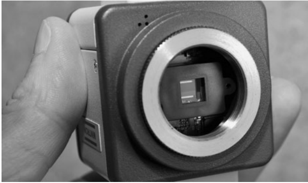
Figure 2-4 The CCD or CMOS imager shown with the lens removed.
