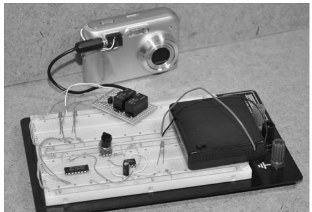
Figure 22-5 The complete system is being tested with the timer on a breadboard.
