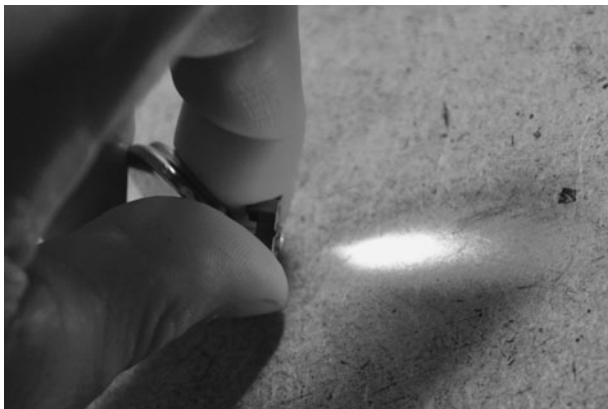
Figure 8-8 Powering up a bare laser diode using a 3-V coin battery.
