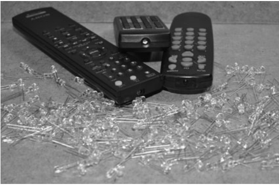
Figure 3-3 These 5-mm axial lead infrared LEDs are inexpensive and easy to work with.
