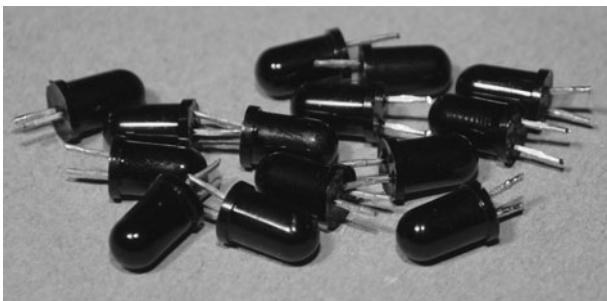
Figure 10-29 LED leads trimmed to a minimal length.
