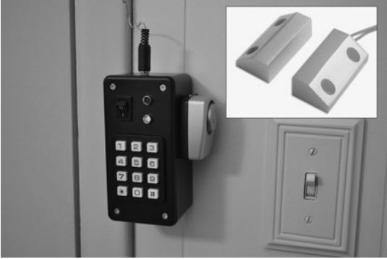
Figure 20-30 A semipermanent installation using a magnetic door switch.
