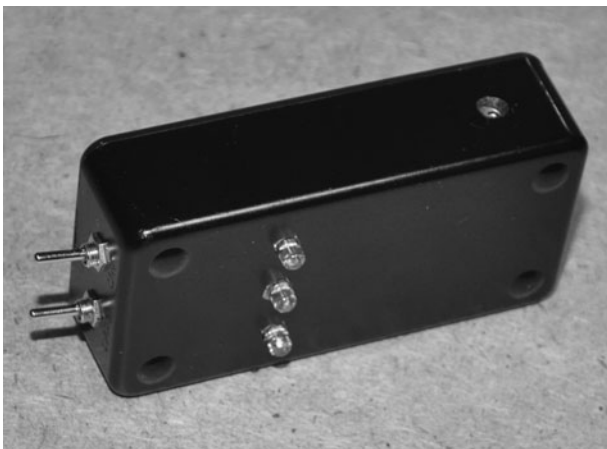
Figure 26-15 The completed and functional clap snap ready for use.
