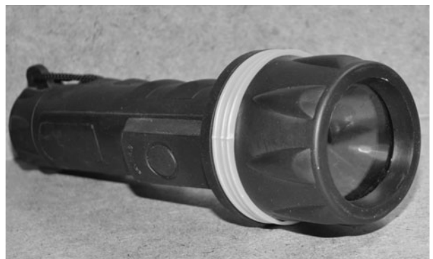
Figure 4-15 The completed near-infrared beam flashlight using the camera film.
