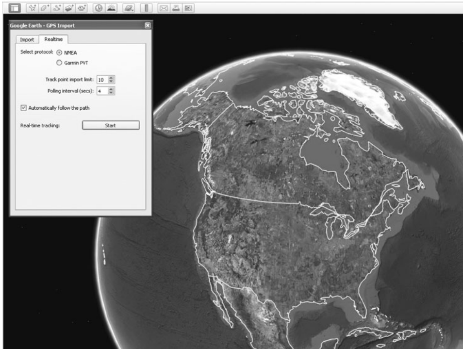
Figure 15-15 Setting Google Earth to display real-time NMEA data from a GPS.
