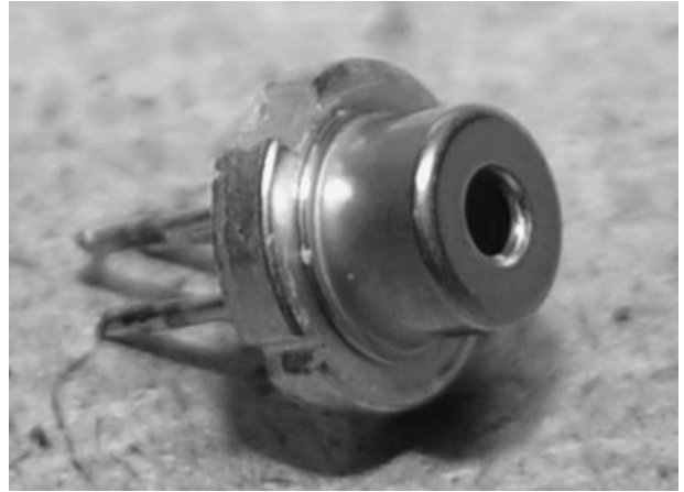
Figure 3-9 This is the bare 60-mW infrared laser diode from a CD burner.
