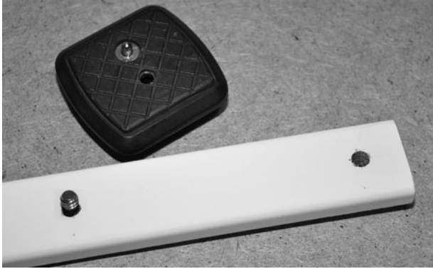
Figure 25-9 Using the mounting bolt from a tripod base to fasten the camera.
