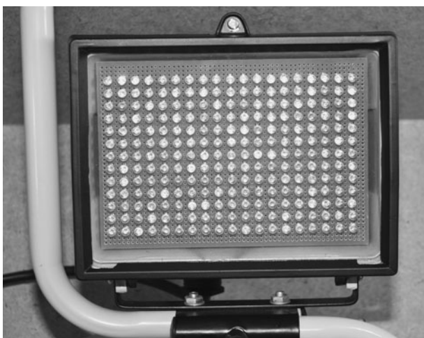
Figure 6-0 A long-range infrared illuminator can be made using many LEDs.
