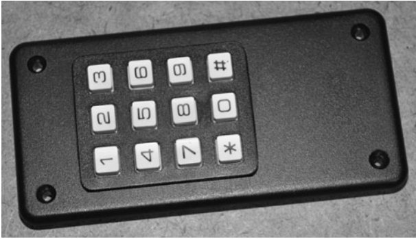
Figure 20-7 The keypad fits like a glove after cutting the opening.
