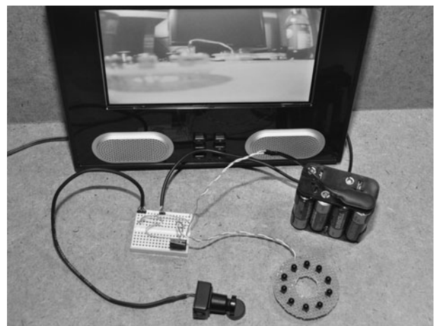
Figure 5-15 To test the infrared illuminator, you will need a video source and a monitor.
