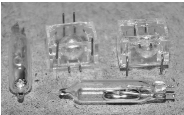
Figure 20-14 A few different motions switches for self-contained mode.
