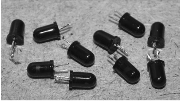
Figure 5-5 Some infrared LEDs include a band pass filter in their casings.
