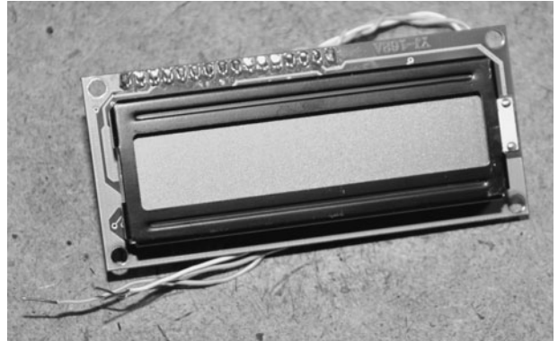
Figure 11-9 This is an easy-to-interface 16 character by two line LCD screen using a serial input.
