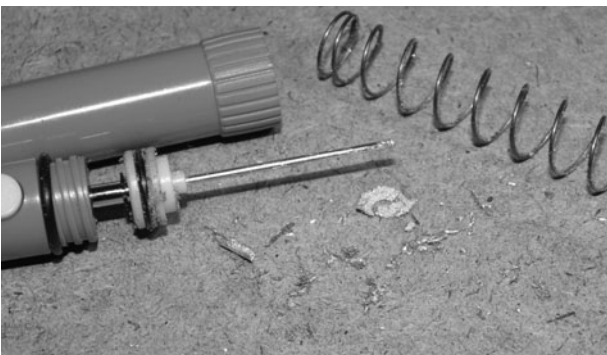
Figure 1-4 The desoldering tool will need to be cleaned every so often.
