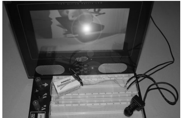
Figure 10-9 Testing the CCD camera's response to infrared light.
