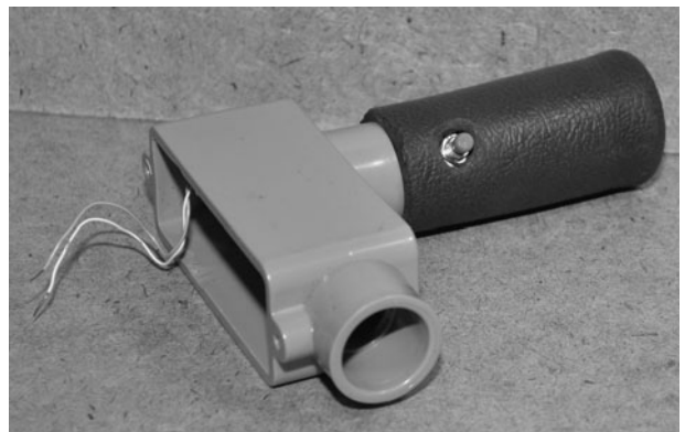
Figure 19-29 The handle grip is placed over the metal tubing.
