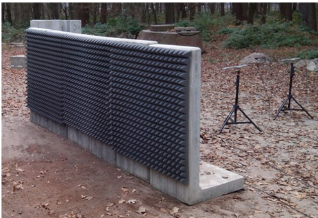
Fig. 2 Barriers equipped with foam acoustic sheeting
