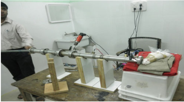
Fig. 5 Reddy tube used for study of blast-induced neurotrauma in rats
