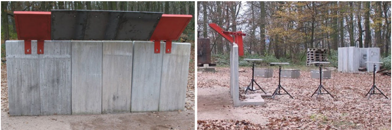
Fig. 4 Barriers equipped with steel extensions
