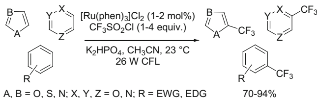
Scheme 1.4 Visible light photoredox-catalyzed trifluoromethylation of (hetero)arenes [83]
