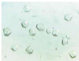
Fig. 5.10 Crystals of DUT-6 (Boron) ( 234 ) as synthesized. Ref. [61]—reproduced by permission of The Royal Society of Chemistry
