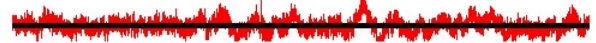
Fig. 6 Response (shown in black color) of the automatic HVS detection algorithm to a typical control signal (shown in red color) in Figure 3, using cmor9-1 wavelet. The response shown here remains same independent of the wavelet functions used in this study. Here the amplitude of control signal and the detector output are normalized to be in the range of 0 to 1.
