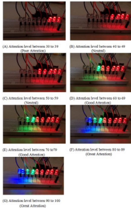
Fig. 3 LEDs attention level indicator for different range of attention level
