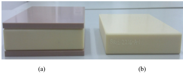
Fig. 2 The standard breast phantom with PGC of 50% (a) and BR-12 phantom (b)
