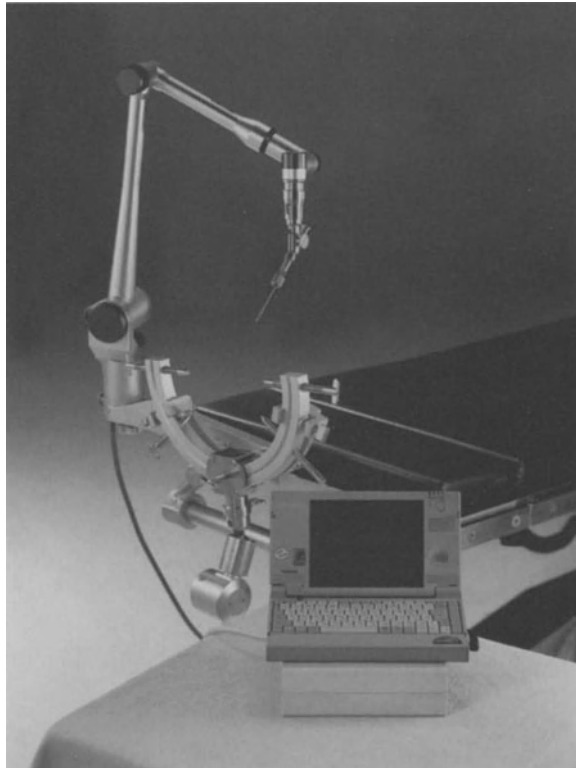
Fig. 1. Minimum construction of the neuronavigator, using palm-top PC with Windows 95
