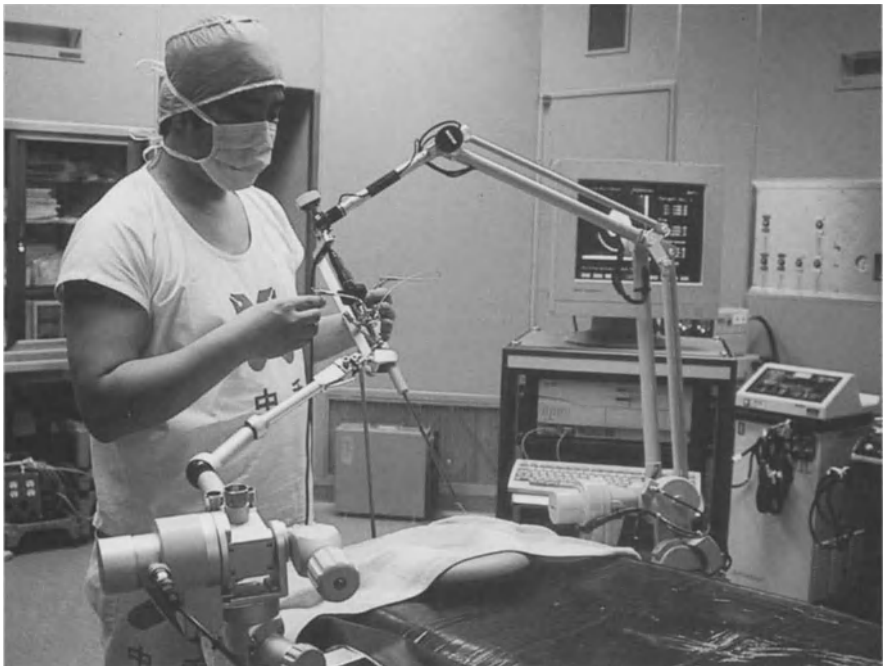
Fig. 4. The navigated endomicroscope consists of a lenscope, the Point Setter, and the Brain Pointer ( top ). A 3-D video system is also sometimes used. The motion of the system is smooth, and the endoscope can easily be set at any position and to any direction and also held very firmly ( bottom )
