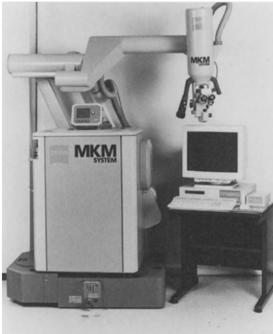
Fig. 1. The Mehrkoordinaten Manipulator (MKM) system created by Zeiss (Oberkochen, Germany) is one of a new generation of microscopes, incorporating a surgical microscope with a computer workstation
