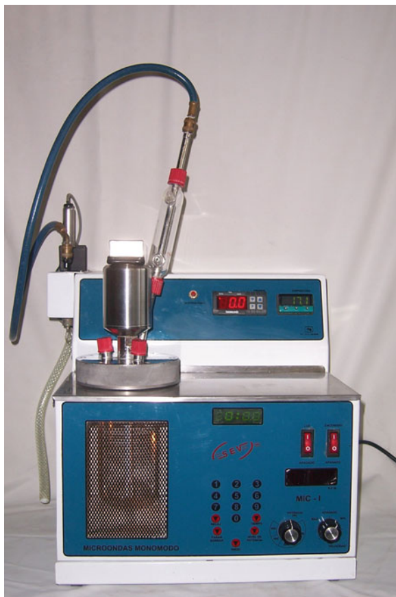
Fig. 1.2 Synthesis autoclave apparatus operated with microwave irradiation
