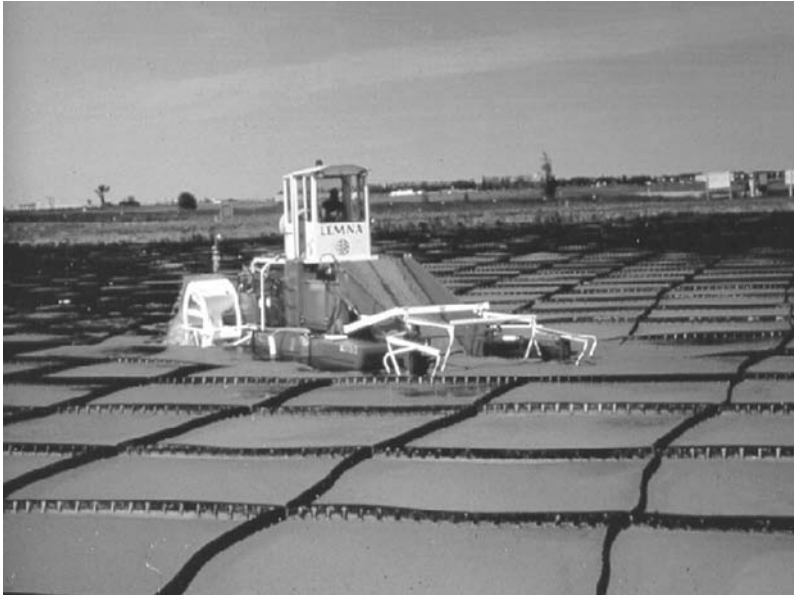
FIGURE 4.25 Photograph of Lemna harvesting equipment and floating barrier grid. (Courtesy of Lemna Technologies, Inc., Minneapolis, MN.)
