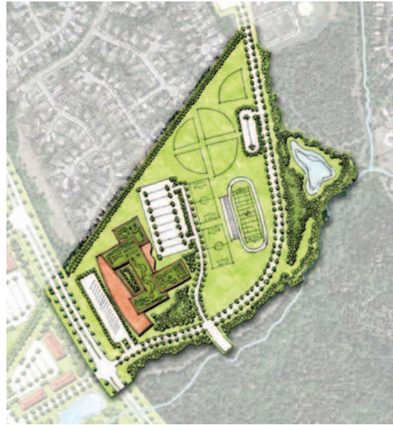
Figure 9.19 School site, Concord Parkway Master Plan, 2004; The Lawrence Group, Town Planners & Architects. The drawing indicates the use of green roofs and the building's siting provides good solar potential on the remaining roof area. Although these ideas of sustainable design are not commonplace in school construction in the conservative Charlotte region, the master plan takes every opportunity to push a sustainability agenda.
