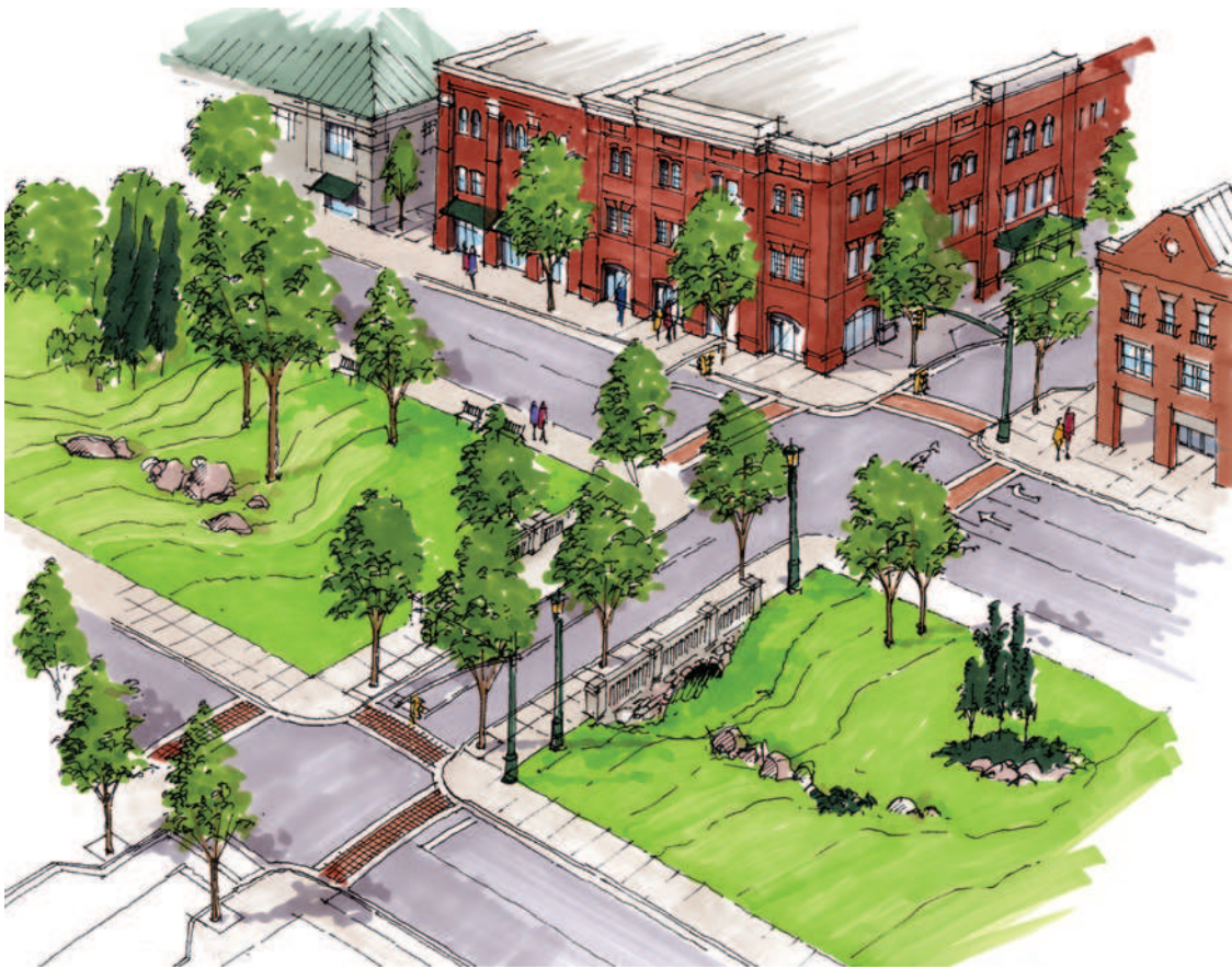
Figure 9.17 Sustainable Urban Drainage System (SUDS), Concord Parkway Master Plan, 2004; The Lawrence Group, Town Planners & Architects. Low Impact Development (LID) is beginning to influence American site design practices. This schematic depiction follows similar guidelines to SUDS in use in British developments such as Upton (see Figures 5.11 and 5.34).
