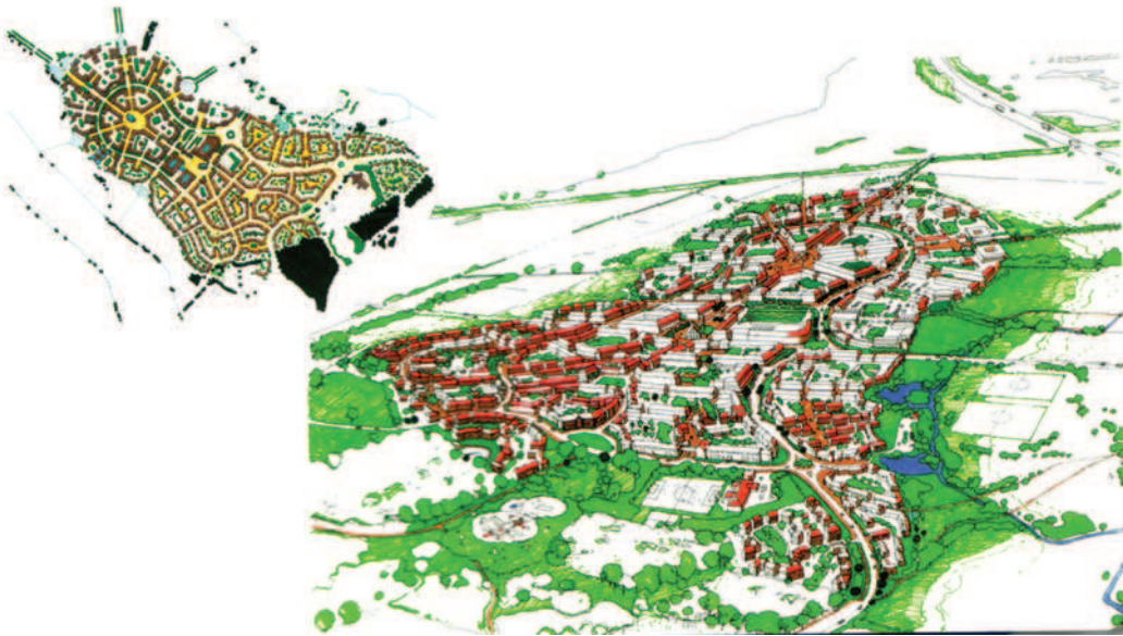
Figure 5.27 Typical British development brief, from Urban Design Guidance (Cowan, 2002). Development briefs can become very design specific. While not master plans in themselves, they illustrate preferred urban design solutions in schematic terms. (Reproduction courtesy of Thomas Telford Publishing)
