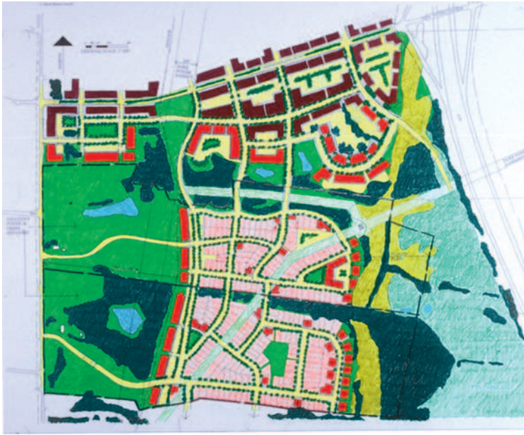
Figure 5.7 Site layout for development in Cornelius, NC, 1995; David Walters. This hypothetical design illustrated the ability for new development to integrate different commercial and residential uses, and achieve high densities while preserving important landscapes on a complex site traversed by utility easements.
