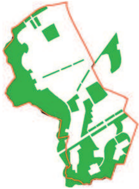
Figure 9.5 Green infrastructure diagram, Concord Parkway Master Plan, 2004; The Lawrence Group, Town Planners & Architects. Presenting the green spaces as a simple figure-ground diagram communicates the size and structure of the landscape system as a positive design element.
