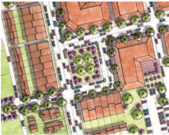
Figure 7.10 Plan detail with shadow; The Lawrence Group, Town Planners & Architects. This master plan excerpt depicts all buildings with one ‘naturalistic’ roof color. The uses of the buildings can be inferred from the sizes and shapes of the building footprints and roofscapes: this example shows town homes with rear garages, detached houses and commercial buildings. The buildings and urban spaces can be easily understood in a manner akin to an aerial photograph, and lining the buildings, trees and cars with shadows provides extra three-dimensional emphasis.
