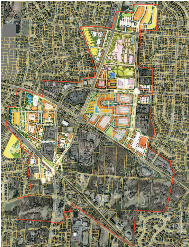
Figure 7.8 Photoshop collage; The Lawrence Group, Town Planners & Architects. Master plans are most easily produced by scanning or photographing detailed hand drawings and collaging them into an aerial photograph of the project area using Adobe Photoshop. This eliminates the previously arduous task of redrawing the whole area by hand.
