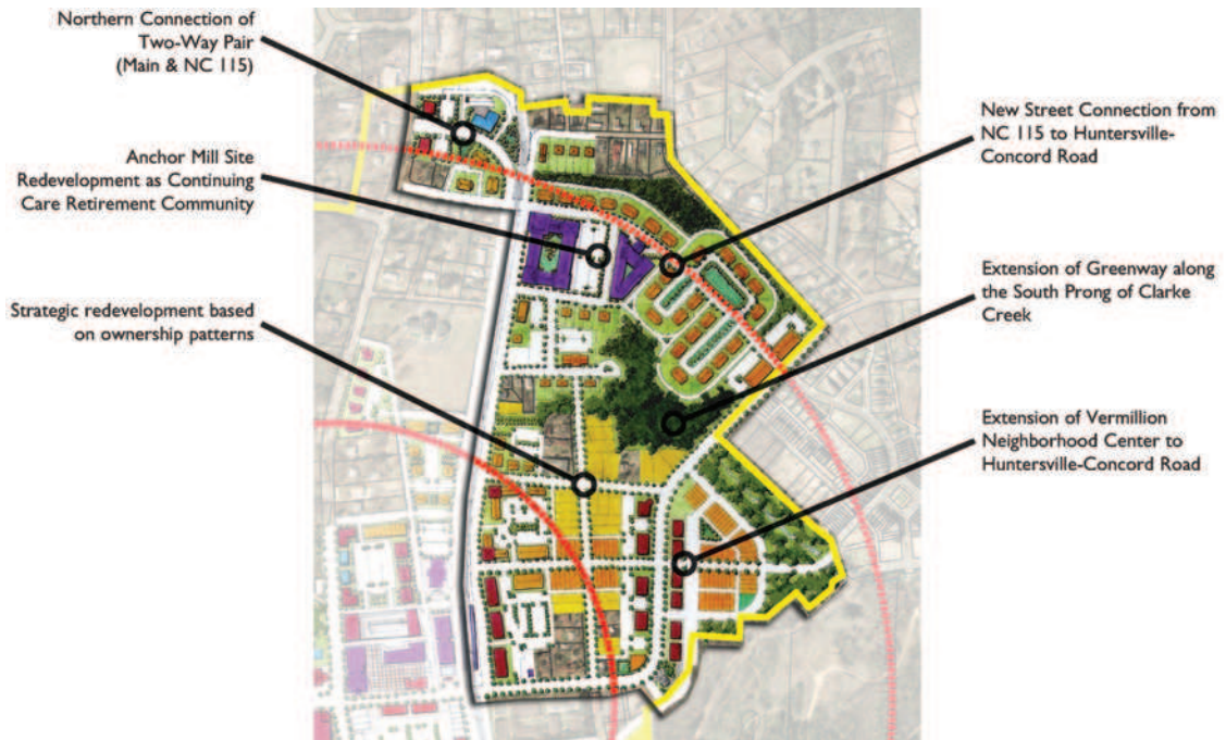
Figure 8.23 Mill neighborhood, Huntersville Master Plan, 2004; The Lawrence Group, Town Planners & Architects. The design team struggled with the relationship between the location of the retirement community and the need for a connecting street network (with the consequent potential for disruptive cut-through traffic). Eventually it was decided to allow one connecting street to penetrate the elderly housing area, but to design it so that vehicle speeds would be strictly reduced for pedestrian safety by means of narrow traffic lanes, on-street parking, stop signs and aggressive speed bumps. In this way, the attractiveness of the street as a cut-through for motorists could be sharply reduced.
