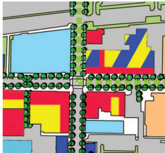
Figure 7.9 Plan detail with stripes; The Lawrence Group, Town Planners & Architects. Attempting to pinpoint uses in this way undercuts the central concept of form-based zoning that uses may change over time while building forms remain largely unaltered. This plan remains a functional diagram rather than a means of communicating the urban design qualities of buildings and spaces.
