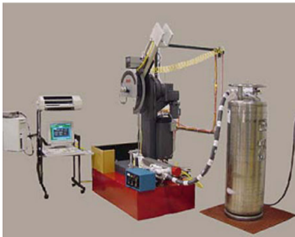
Fig. 10.6 Tinius Olsen Model 84 Instrumented Charpy impact machine equipped with in situ heating and cooling system, optical encoder for measuring the impact velocity, and motorized hammer (striker) return [43]
