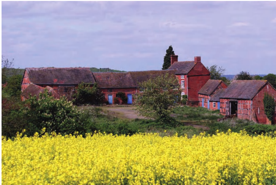
Figure 5.3 Farmstead in the Forest of Arden, retaining two timber-framed barns and a stable; the farmhouse and other buildings were rebuilt from the late eighteenth century (Peter Gaskell). The combination of timber frame and eighteenth–nineteenth-century brick is a characteristic feature of the anciently enclosed landscapes of the West Midlands.
