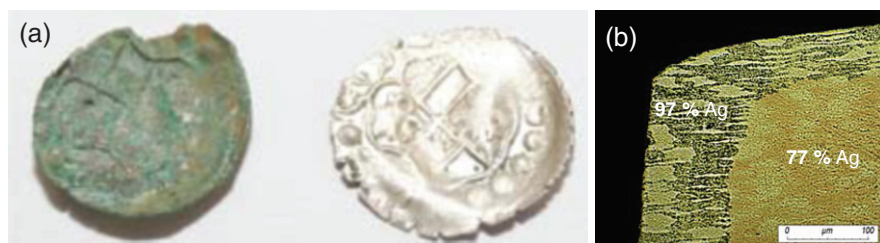
Fig. 5.12 (a) Medieval coins from the Preuschof's hoard, as found ( left ) and after cleaning with chemicals ( right ); (b) Cross section of a test sample (80% Ag/20% Cu) showing the influence of 48 h of immersion in a cleaning solution ("silver dip") on the surface composition (after [278])
