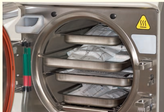
An autoclave can be used to sterilize many dry and liquid materials.
