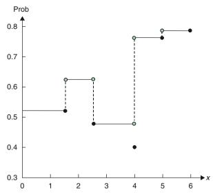
tion  $P(\max\{h_i d(i, x)\} > r)$  over the primary region [0, 6.0] is graphically depicted in Fig. 11.2. The optimum is reached at x = 4.
