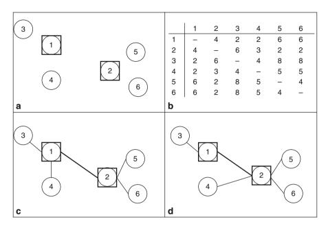
Fig. 12.2 Two different allocation schemes on an example network. a Network configuration. b Distance matrix. c Allocation scheme 1. d Allocation scheme 2
