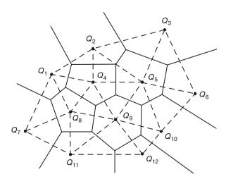
Fig. 19.8 Solid line Voronoi diagram for twelve seed points  $Q_1, Q_2, ..., Q_{12}$ , and broken line Delauney tessellation
