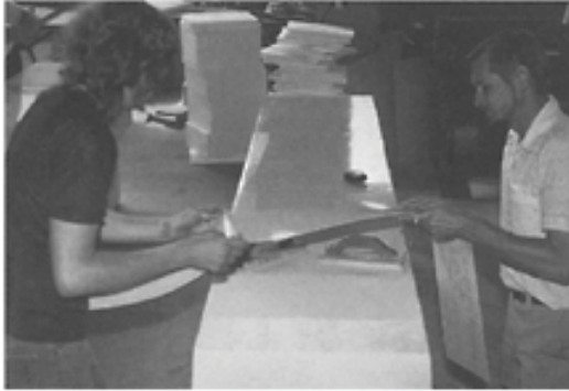
Manufacturing Plastic Covered Foam Blocks
