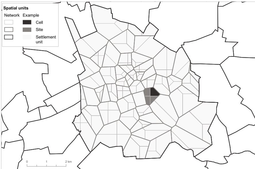
Fig. 17.2. Example of distribution network cells and sites in city of Tartu (100 000 inh.).
