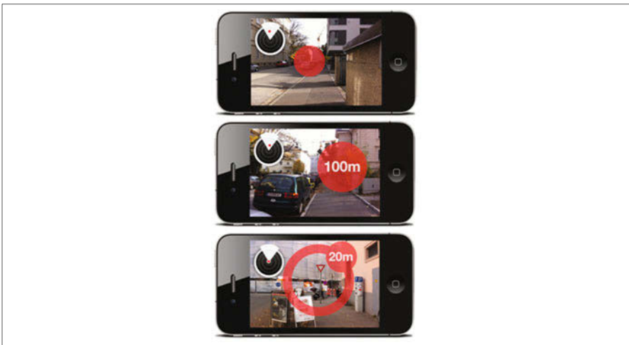
Fig. 1.2. Graphical indicators being displayed as augmented reality overlay over the camera view and changing their style upon the distance to a decision point.
