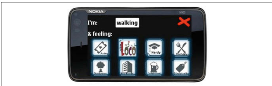
Fig. 3.4. I’m feeling LoCo interface. The interface displays the detected transportation mode of the user and presents eight buttons from which the user can select their current mood.
