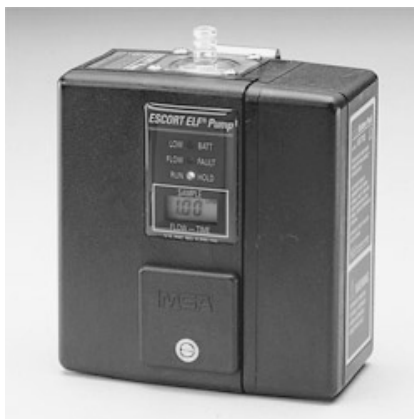
Figure 10.1 Personal air sampling pump. This model has an internal secondary standard that calibrates the pump continuously and is checked against a primary standard only once a month. (MSA—Escort ELF)
