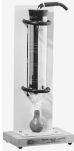
Figure 3.4 This portable standard flowmeter can be used in the office or laboratory, and in the field. (SKC)
