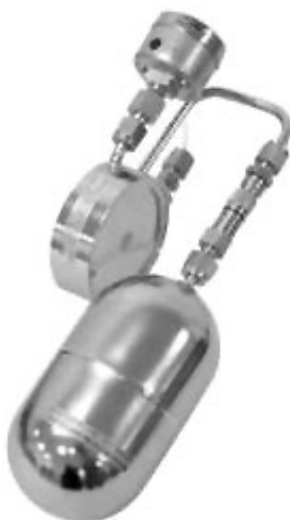
Figure 2.11 Stainless steel canisters are used for collecting air samples of VOCs and sulfur compounds over a wide concentration range (1 ppb to 10,000 ppm). This 400-cc unit can be placed at a sampling site for area sampling or attached onto a worker's belt for personal sampling. (SKC-MiniCans)
