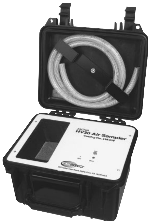
Figure 2.29 Dual-diaphragm pump for indoor and outdoor collection of particulates, PAHs, and other compounds requiring flows from 10 to 30 l/min. High-flow pumps are used for asbestos, PAHs in indoor air, PM10 and PM2.5 in indoor air, bioaerosol sampling, stack sampling, fence line monitoring, and background monitoring. (SKC—AirCheck HV30 Environmental Air Sampler)
