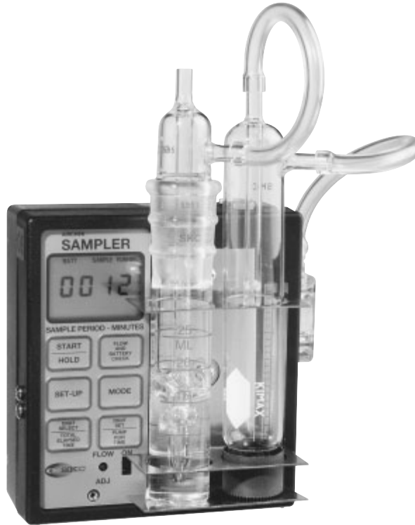
Figure 2.33 Impinger and in-line trap holder mounted on sample pump. Use a trap impinger to prevent impinger liquids from being drawn into the sample pump. Solid sorbents may be added to the trap to protect the pump chamber from exposure to vapors when volatile liquids are used. (SKC)
