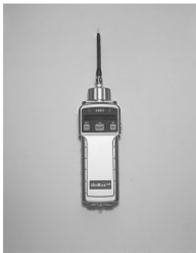
Figure 2.3 Photoionization detector with a 10.6 eV detector. (RAE Systems)
