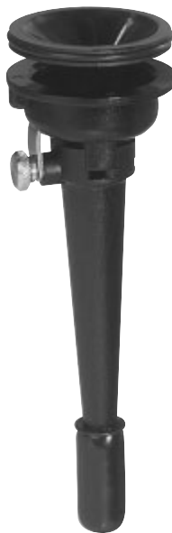
Figure 2.42 The GS cyclone is a conductive plastic unit that holds a filter cassette for collecting respirable dust particles. The GS cyclone has a 50% cut point of 4.0 \mu\text{m} at 2.75 l/min. (SKC)
