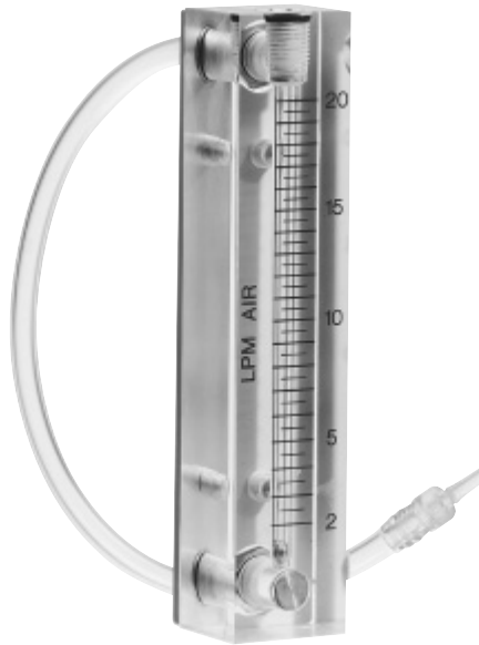
Figure 3.10 Secondary standard rotameters are used in the field to calibrate air-sampling pumps. Rotameters are calibrated to a primary standard. Flow rates must be corrected for standard temperature and pressure. (SKC)
