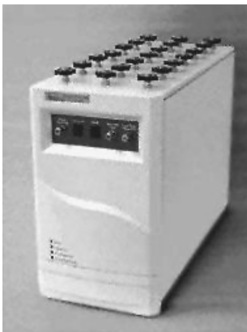
Figure 2.10 The Tedlar Bag Autosampler automates the introduction of up to 21 samples into a GC for quantitative analysis. (Entech Instruments Inc.)
