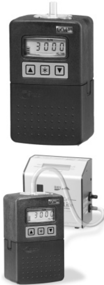
Figure 3.8 An electronic adapter is available to automatically calibrate an air sampling pump. (SKC—AirCheck® 2000 air sampling pump, CalCheck® Communicator with DC-Lite calibrator). (Bios International Corp.)
