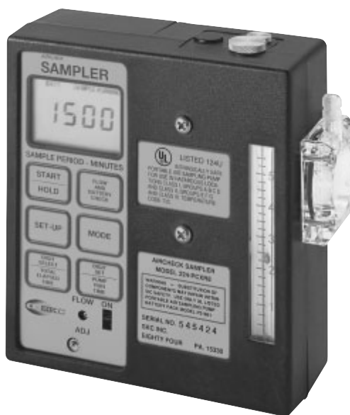
Figure 2.60 A sampling pump can be used in high flow (750–5000 ml/min) or low flow (5–500 ml/min). Low flow requires an adjustable low-flow holder. (SKC—Model 224-PCXR8)
