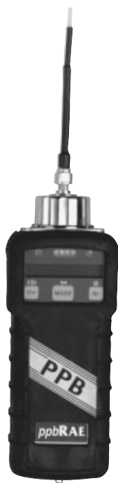
Figure 2.4 Handheld VOC monitor with parts per billion detection. (RAE Systems)
