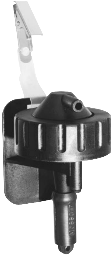
Figure 2.44 The conductive plastic respirable dust cyclone is a lightweight conductive plastic unit. The unit is designed for a 50% cut point of 5.0 \mu\text{m} at 1.9 l/min and 4.0 \mu\text{m} at 2.2 l/min. Conductive plastic construction eliminates static problems. (SKC)
