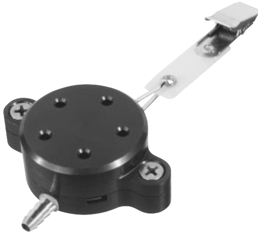
Figure 2.58 The PEM is a lightweight, personal sampling device consisting of a single-stage impactor and a final filter. Aerosol particulates are sampled through the single-stage impactor to remove particulates above the 2.5 or 10 \mu\text{m} cut point, depending on which sampling head is chosen. (SKC)
