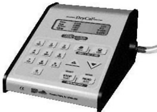
Figure 3.9 The electronic standardization and communication module provides time/date stamping; employee, pump, and sample ID numbers; volumetric flow rate readings; and readings at user-defined time intervals for flow stability testing. (Bios International Corp.)
