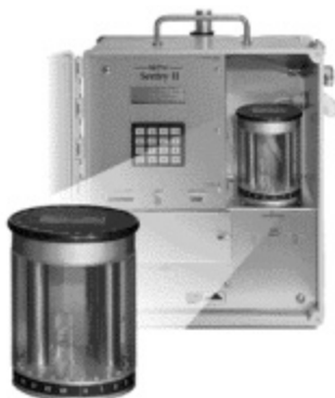
Figure 9.1 Fenceline monitoring equipment can be used for IAQ investigations, ambient air monitoring, and hazardous waste site evaluation. This model can sample a maximum of 24 sequential sorbent tube samples in a single sampling sequence. Time, date, mass flow, tube number, temperature, and wind direction and speed can be automatically logged into memory and printed or downloaded into a personal computer. (BIOS International Corp.)
