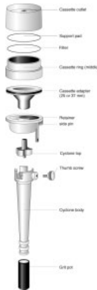
Figure 2.48 Exploded view of a respirable dust cyclone cassette assembly. (SKC)
