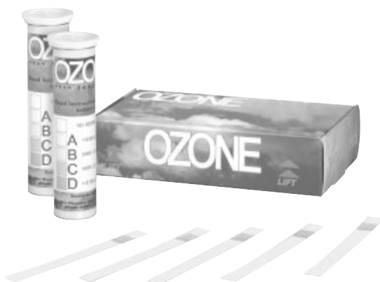
Figure 2.25 Ozone strips provide quick indication of ambient levels of ozone in both indoor and outdoor air. Ozone strips are chemically treated to react with ozone. Test strips are placed in the area to be tested. After 10 min, compare the test strip with the color scale on the test strip package. Results display in four distinct colors from light yellow to to brown. Each represents a certain level of ozone concentration. (SKC)
