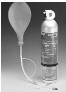
Figure 3.11 Bump testing needs to be performed regularly to ensure that real-time air monitoring instrumentation is functioning properly. (MSA)
