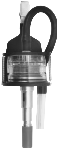
Figure 2.51 Cassette holder on aluminum cyclone with filter cassette (37 mm). (SKC)
