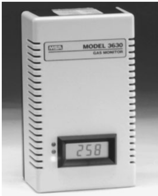
Figure 2.6 An infrared gas monitor measures carbon dioxide and sends a signal to the ventilation control system.
