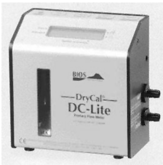
Figure 3.7 An electronic flow calibrator is available that does not use soap; instead it uses a graphite/carbon-composite piston that rises in the chamber like the bubble. (Bios International Corp.)
