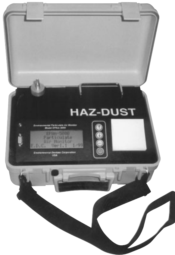
Figure 2.61 Real-time dust monitoring offers immediate real-time determinations and data recordings of airborne particle concentration in milligrams per cubic meter. Interchangeable size-selective sampling heads allow PM 10 , PM 2.5 , or PM 1.0 monitoring. (HAZ-DUST—EPAM-5000 Environmental Particulate Air Monitor) (SKC)
