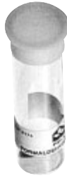
Figure 2.26 A formaldehyde passive air sampler for indoor air sampling. Easy to use, it is designed for long-term measurement (5 to 7 days). Its detection limit is 0.01 ppm. (SKC)
