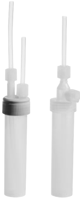
Figure 2.35 Teflon PFA (fluoropolymer) impingers. These vessels are completely inert to virtually all chemicals and perform well in both high temperature and cryogenic applications. (SKC)
