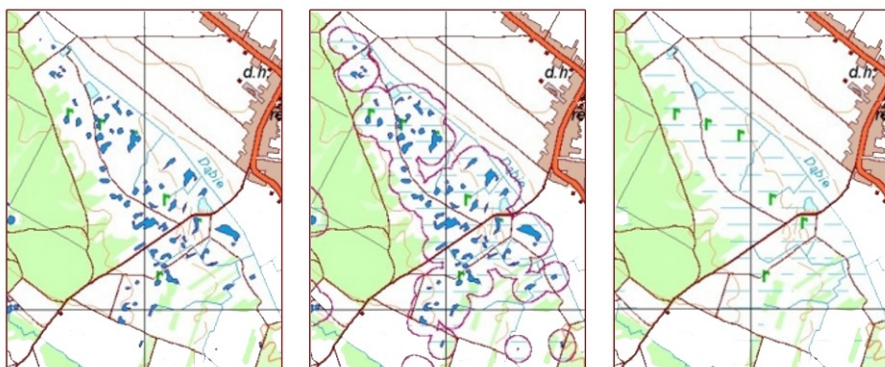
Fig. 6.5. Presentation of wet areas, marked in dark blue, by means of equi-distance lines (buffers), which delineate the final linear pattern
