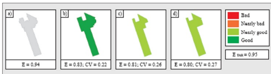
Fig. 9.13. Evaluation results of elongation constraint (ratio of mbr axes): a) initial map object; b) manual generalised map object; c) and d) automatically generalised map objects.
