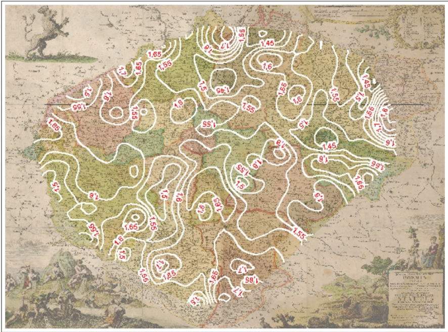
Fig. 33.6. Scale isolines of the longitudes of Vogt's map generated with the step 0.05
