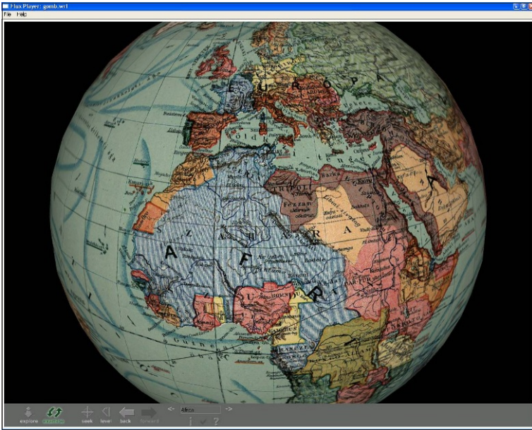
Fig. 18.4. Moire effect appearing due to the interference of the sampling grid and the printing raster
