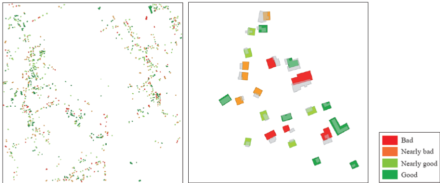
Fig. 9.10. Evaluation of absolute position constraint on manual generalised building map objects from TD Kadaster at 1:50k. Left figure shows an extract of the data set.
