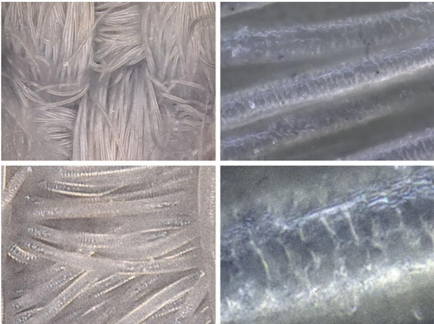
**Fig. 5.2** Microscopic pictures of laser-treated polyester fabrics, taken with different magnifications (*upper panels*), and respective details (*lower panels*)
