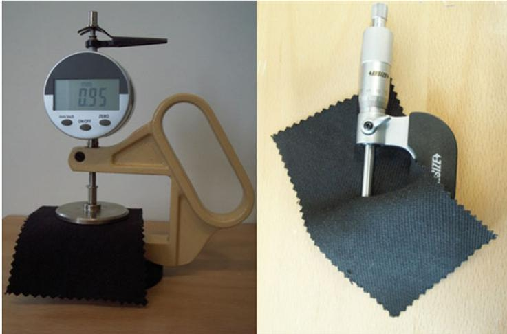
**Fig. 10.18** Thickness measurements on the same fabric using a device based on EN ISO 5084 (*left panel*) and a usual micrometer gauge (*right panel*)
