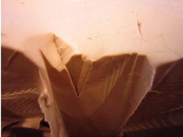
**Fig. 11.5** Digging out the penetration channel in the Plasticine after a VPAM-KDIW test
