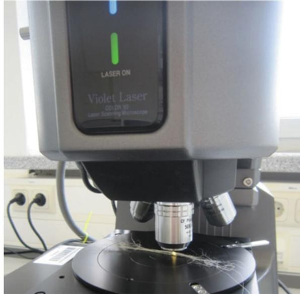
Confocal laser scanning microscopes contain a common white light source in combination with a laser beam. Since the possible resolution of a picture is proportional to the wavelength of the light used, these lasers often use violet light (e.g., 408 nm wavelength). However, less expensive devices are available with red lasers (658 nm).
