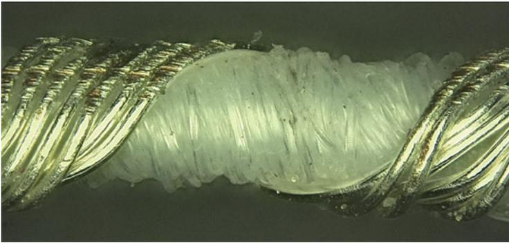
**Fig. 2.14** Wrap yarn composed of textile core and wound metal braid after weaving with damages due to the machine takedown. Wire diameters are approximately 20  $\mu\text{m}$
