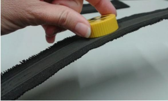
**Fig. 3.5** One magnetic layer 3D printed on a polyester woven fabric
