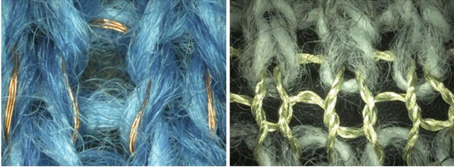
**Fig. 2.6** Conduction lines in knitted fabrics, using copper strand (*left panel*) or silver-coated polyamide filaments (*right panel*)
