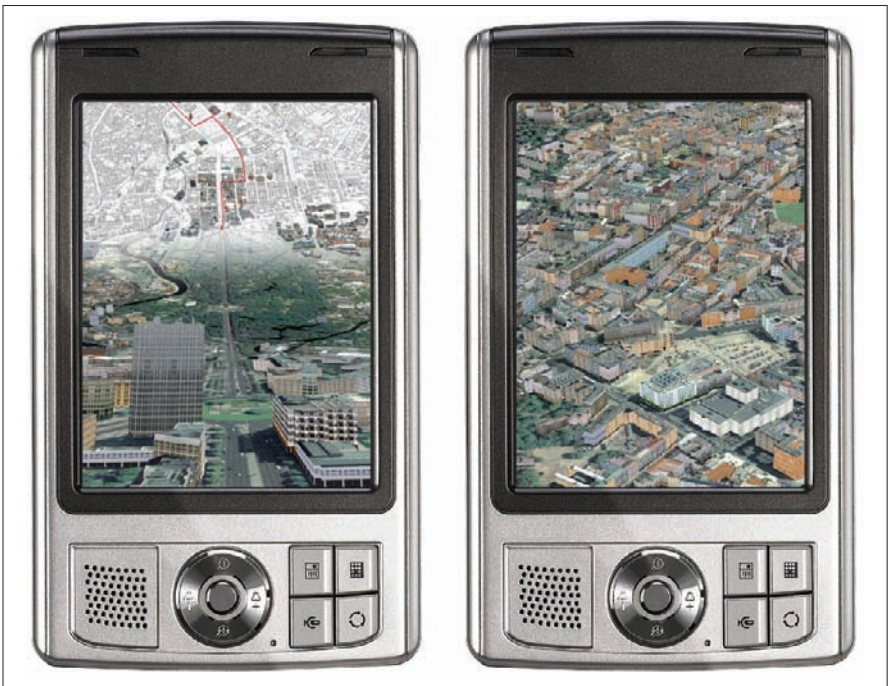
Fig. 13.5. In order to avoid “dead pixel values” and use the transmission plane more efficiently, a degressive central projection may deliver better results than the traditional central perspective.
