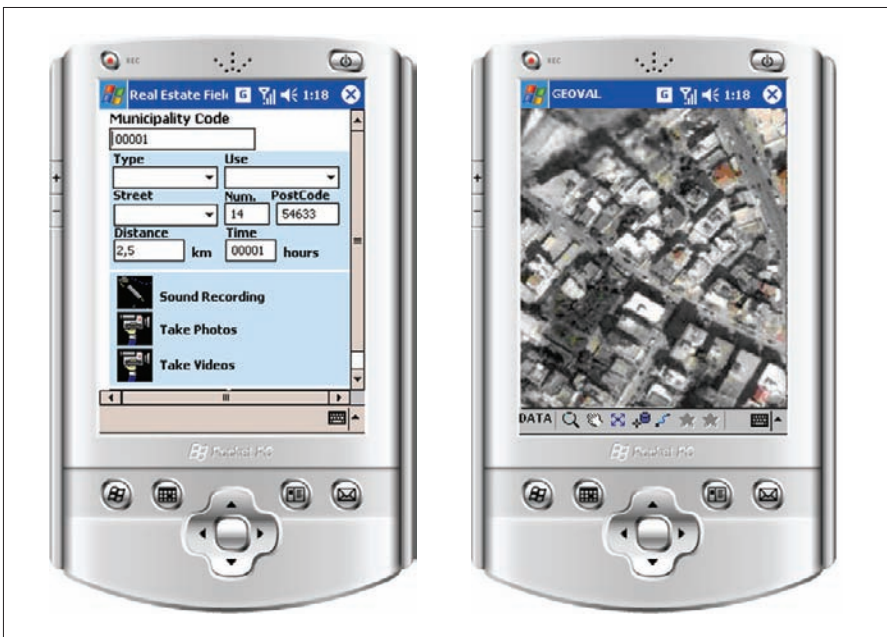
Fig. 19.4. (a) Field data collection through mobile GIS and (b) The satellite image representation in the field GIS application.
