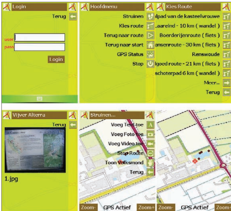
Fig. 15.6. Screenshots of the mobile DIWI client (from left to right: login screen, user modes, predefined routes, personal POI (dummy example), dynamic map and user location and personal records menu).
