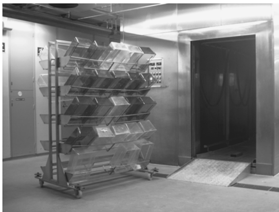
Figure 8.21 A batch-type cage and rack washer that is not pit mounted, thus requiring a ramp to load rolling equipment into the washer. Pit mounting is much preferred in that it avoids the potentially dangerous ergonomic problems associated with the ramp. The wash rack alongside the washer is useful for holding small cages and other small equipment in the cage and rack washer.
