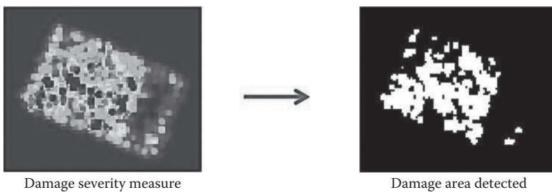
FIGURE 20.14 Segmentation performed by Otsu's thresholding method.
