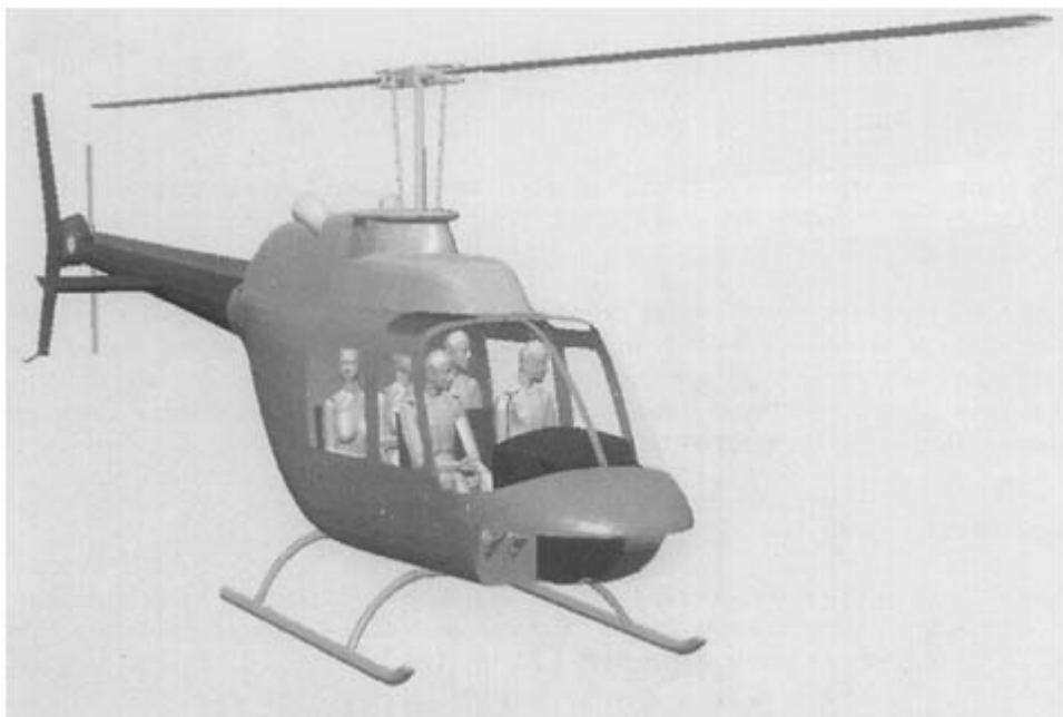
Figure 6.26 Computer reconstruction showing the engineering scale anthropometric human body models of the victims mated to the helicopter model.
