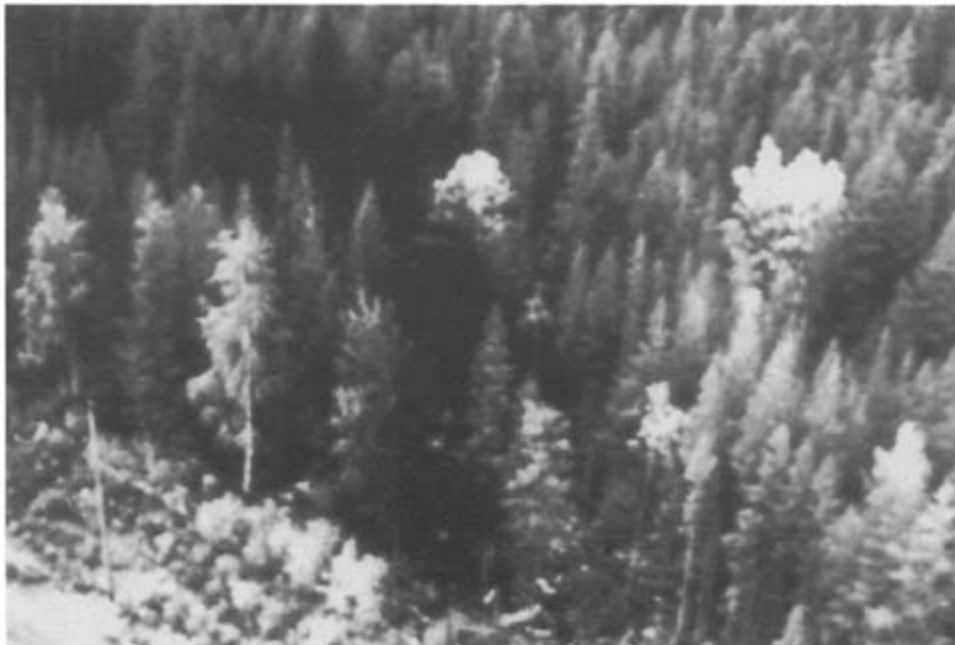
Figure 6.4 Black and white rendition of a false colour infrared photograph showing vegetation stress (dark area) around aircraft wreckage in trees.
