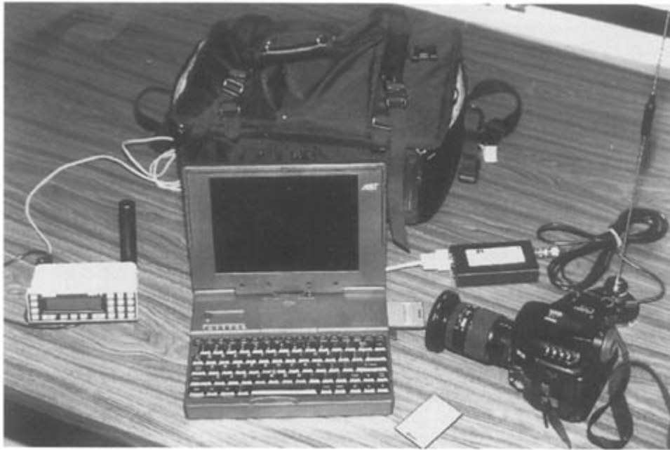
Figure 6.10 General view of a portable multi-media GIS system comprised of a laptop computer (equipped with a removable hard disk and CD-ROM; built-in video capture board, speakers and microphone); interfaced to a mega-pixel digital camera, differential GPS receiver, and radio modem.
