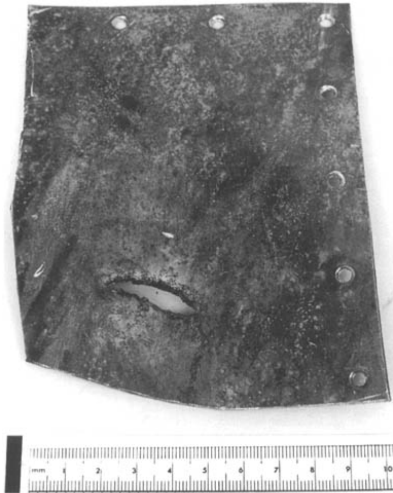
Figure 13.26 Damage to part of engine nacelle.
