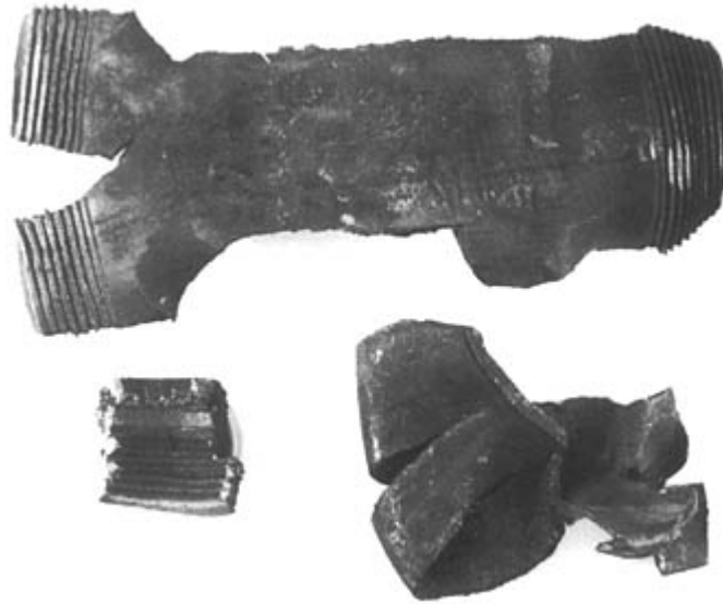
Figure 11.25 Double base smokeless powder pipe bomb (10 inches long; 1.5 inches od) initiated by flame.
