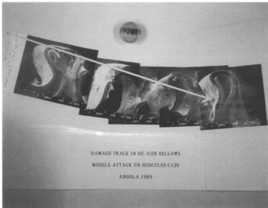
Figure 13.29 Fragment embedded in de-icer can bellows after passing through 13 thicknesses of metal.
