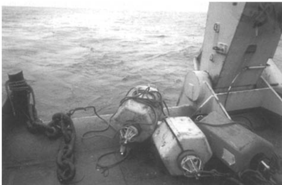
Figure 6.7 Underwater acoustic transponders in flotation jackets being deployed to establish a navigation array.
