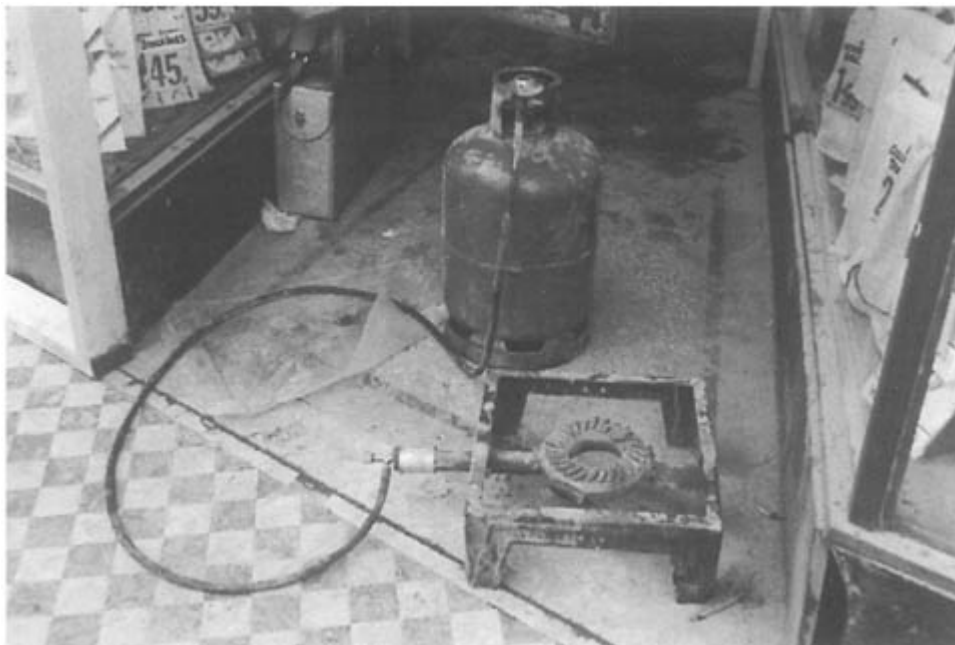
Figure 7.18 Butane cylinder and gas ring recovered from basement.
