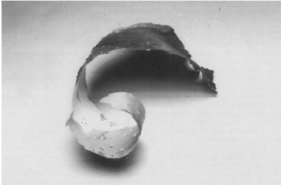
Figure 6.16 Side view of a petal or curl created in the exterior skin of an aircraft fuselage following the detonation of an improvised explosive device (fabricated from a high performance plastic explosive). The dark sooted end is near the center of the blow hole created by the blast.
