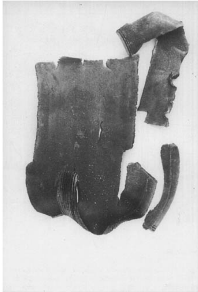
Figure 11.27 Single base smokeless powder pipe bomb (10 inches long; 1.5 inches od) initiated by blasting cap.
