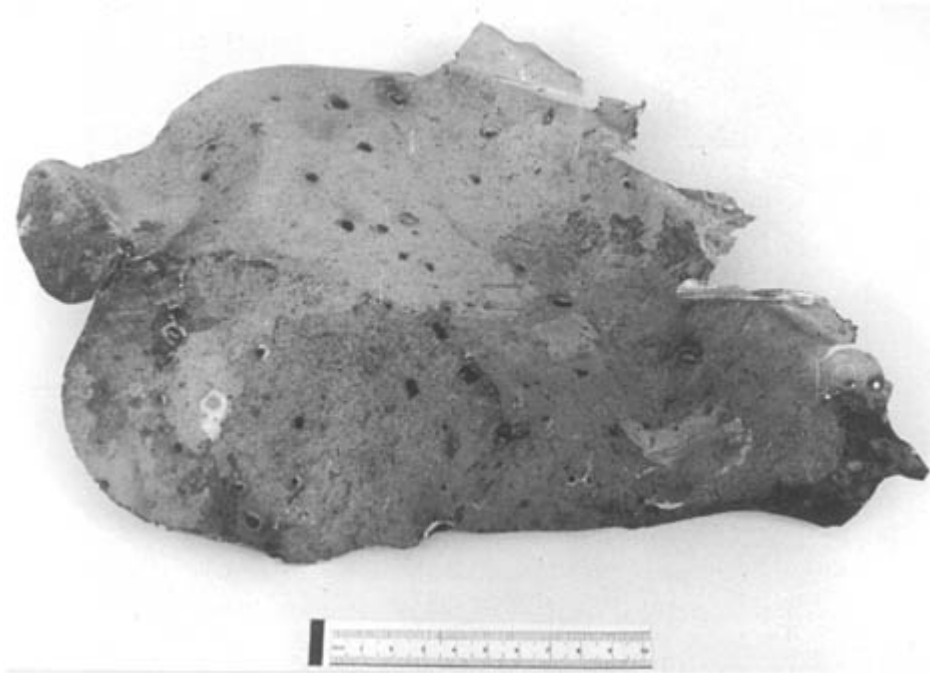
Figure 13.27 Peppering on landing gear wheel door.
