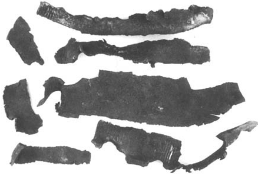
Figure 11.26 Double base smokeless powder pipe bomb (10 inches long; 1.5 inches od) initiated by blasting cap.
