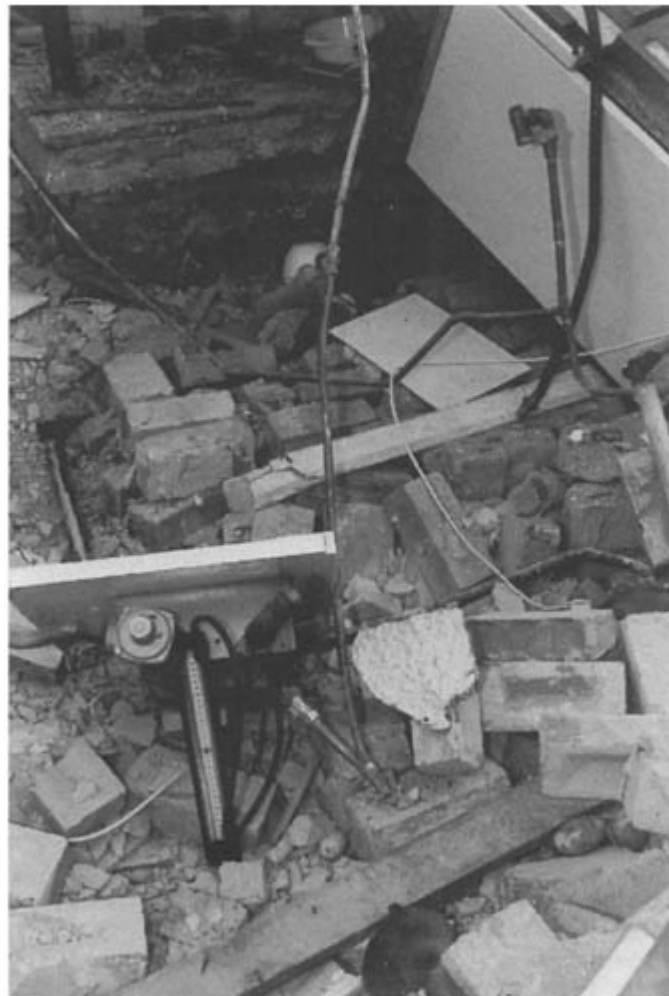
Figure 7.7 U-tube manometer used to test pipes for leaks.
