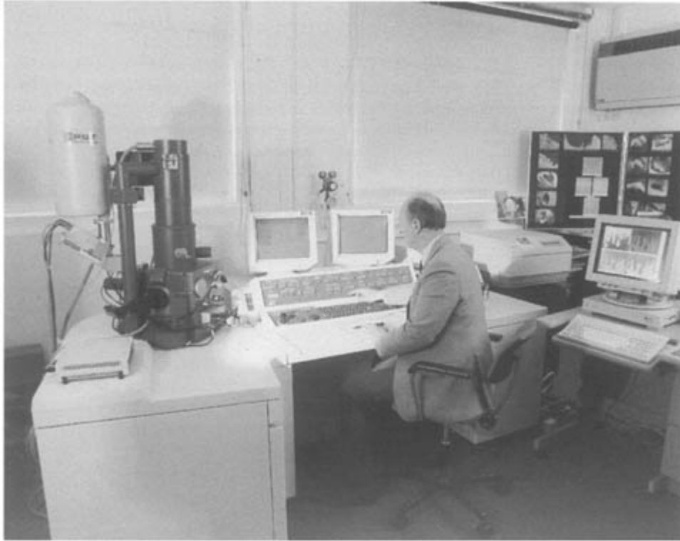
Figure 13.2 Leica-Cambridge scanning electron microscope.
