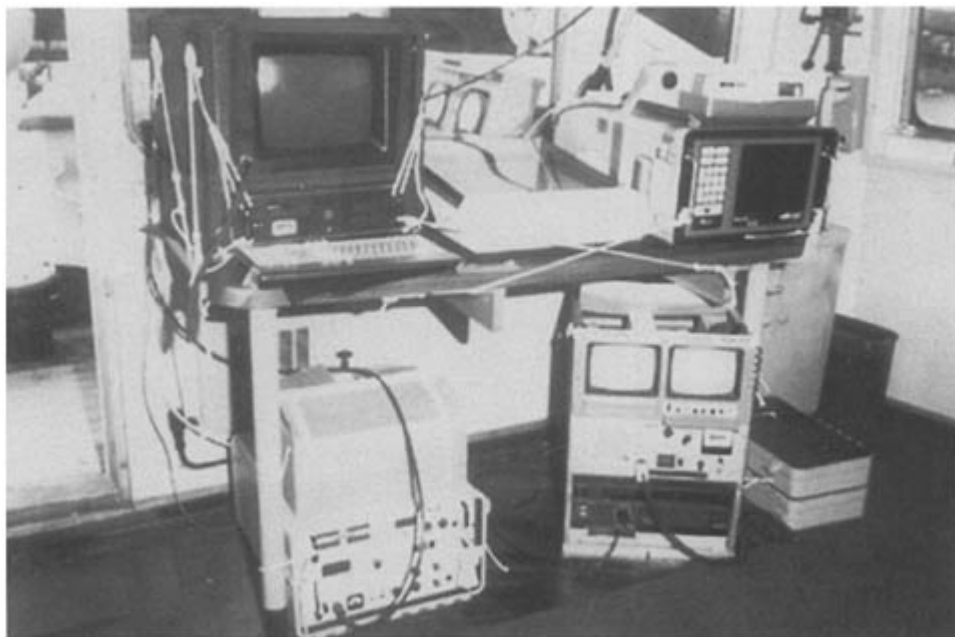
Figure 6.8 Navigation consoles used to integrate surface and subsurface positioning (e.g. vessel and ROV operations).
