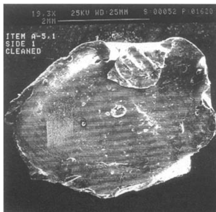
Figure 13.25 Aluminium flake showing craters, and rolled edges.
