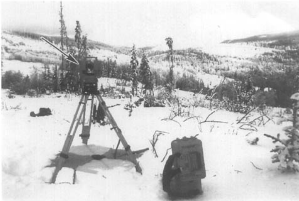
Figure 6.23 General view of an electronic theodolite being used to determine the coordinates of target blanket markers placed around the periphery of the scene to establish survey control for photogrammetry.
