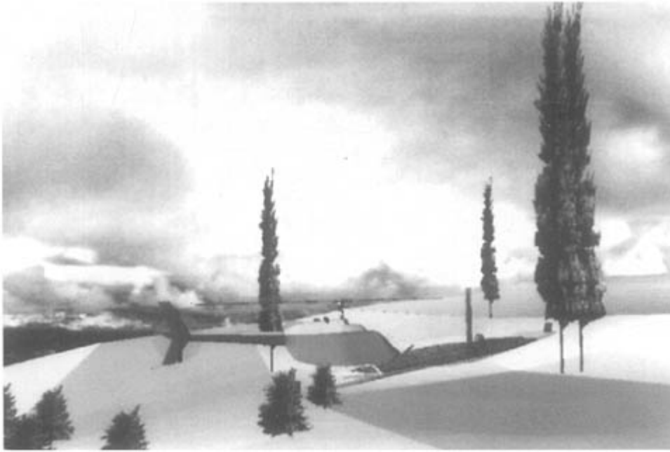
Figure 6.25 Computer reconstruction showing the engineering scale helicopter model mated to ground scars on the terrain model.
