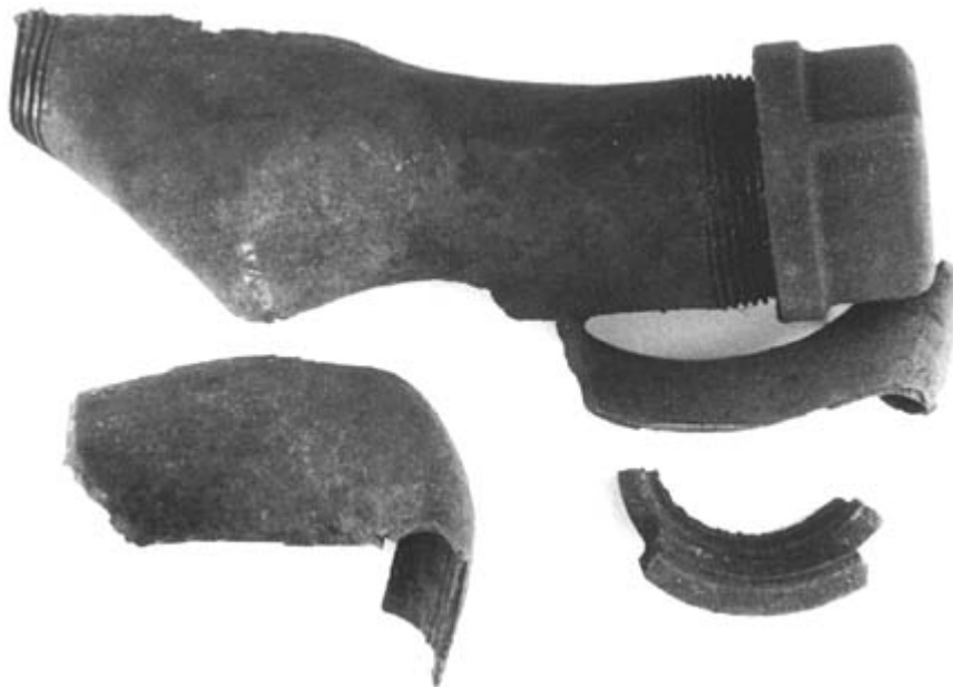
Figure 11.1 Damage to a pipe (10 inches long by 1.5 inches diameter) caused by a low explosive (black powder).
