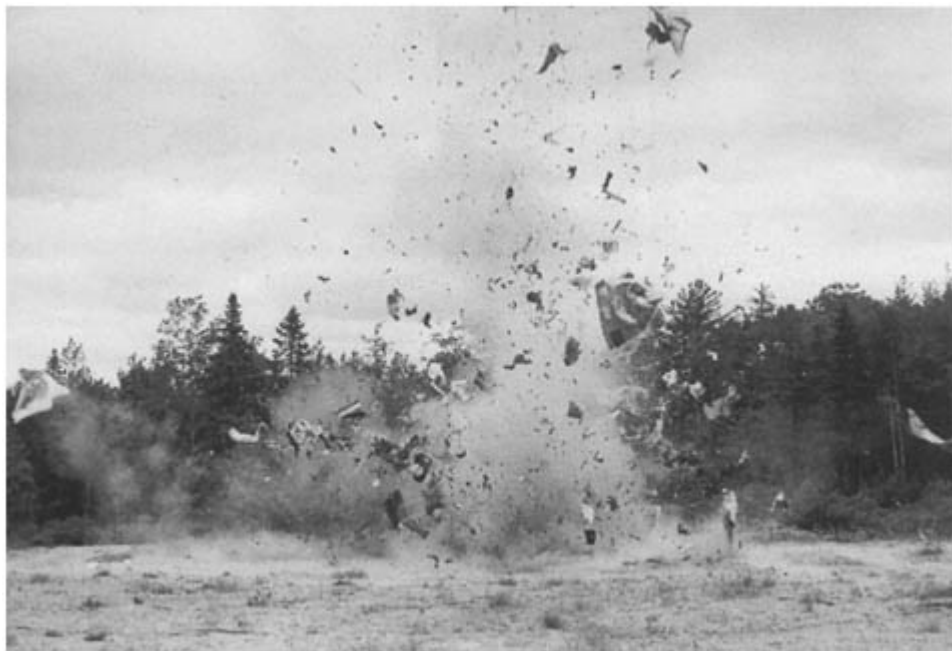
Figure 4.3 Detonation of dynamite in a baggage container.
