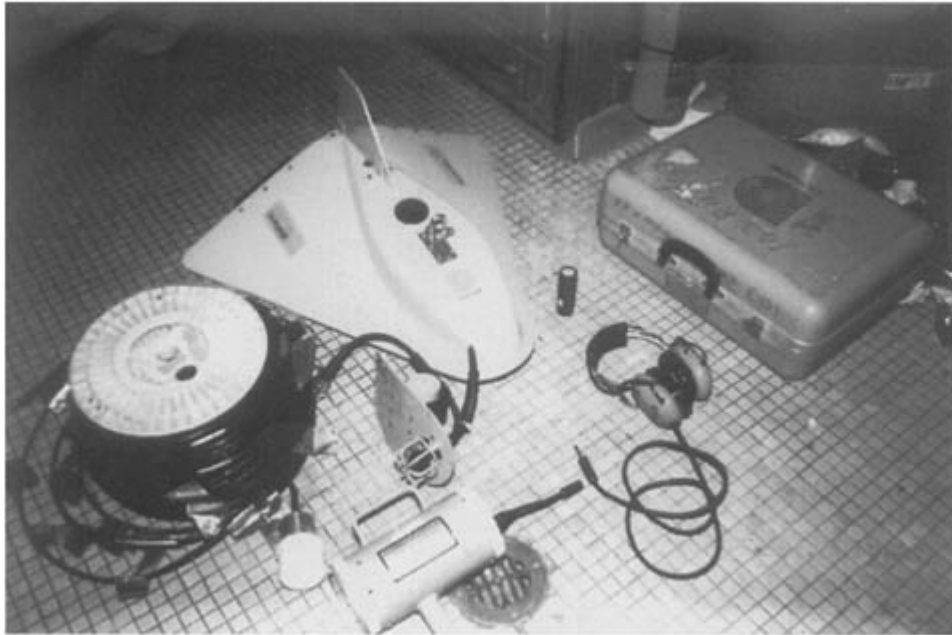
Figure 6.13 Oblique view of towed and hand held underwater acoustic homing equipment.
