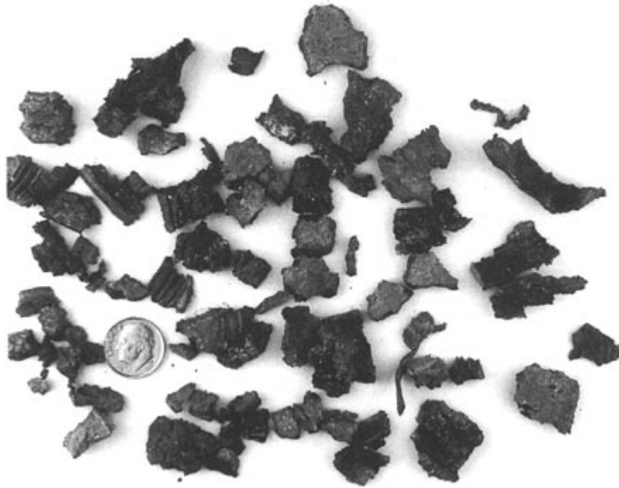
Figure 11.2 Damage to a pipe (10 inches long by 1.5 inches diameter) caused by a high explosive (RDX: military C-4).
