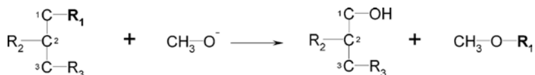
Fig. 6.1 A reaction for the transesterification of a triacylglycerol to yield a fatty acid methyl ester (FAME) and diacylglycerol
