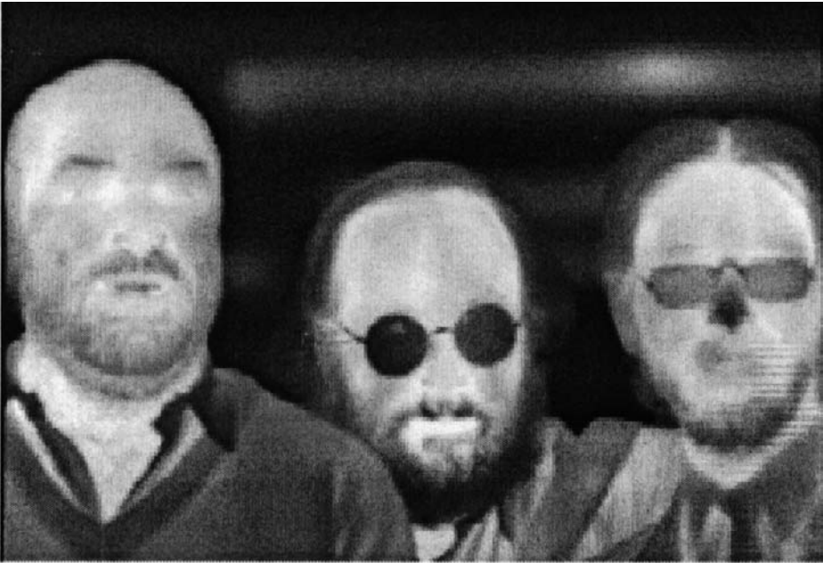
Fig. 7.14 A thermal image produced by an infrared camera exploiting uncooled pyroelectric ceramic detection technology. (Courtesy of QinetiQ Limited.)
