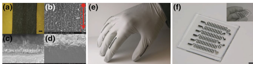
Fig. 11.5 Surface and film architecture details [73]. a Photograph of the carbonized polyimide. Scale bar 250 μm. b SEM image of the aligned particles in the traces with the arrow showing the direction of laser ablation. c Cross-sectional image of the carbon traces showing the porosity of the carbonized material. d Cross-sectional SEM of stretchable carbon traces embedded in PDMS. e Glove equipped with strain sensors at the joints. f Stretchable array of pH sensors
