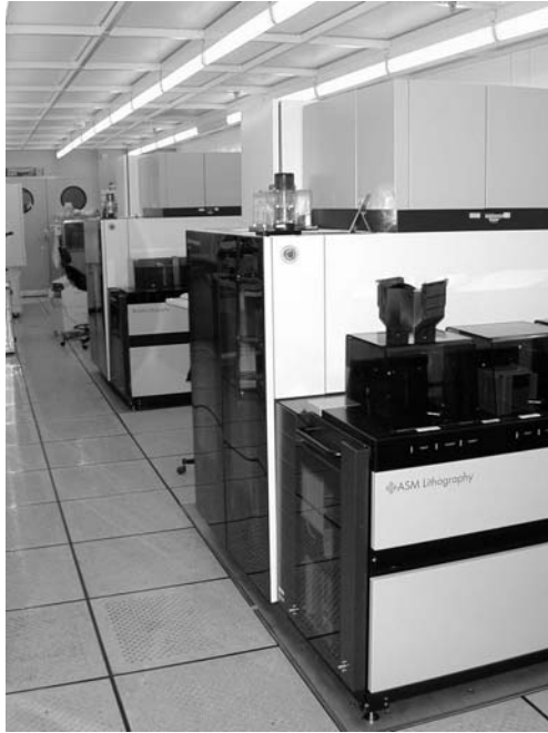
Figure 7.6 A 0.5- \mu\text{m} stepper for 6-in.-diameter wafers. (Source: Bookham Inc., 2006. All Rights Reserved.)
