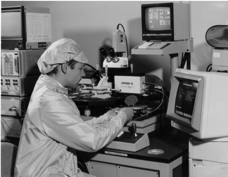
Figure 8.5 The author (in earlier days) loading a 3-in. GaAs wafer onto a RFOW probe station. (Source: Bookham Inc., 2006. All Rights Reserved.)
