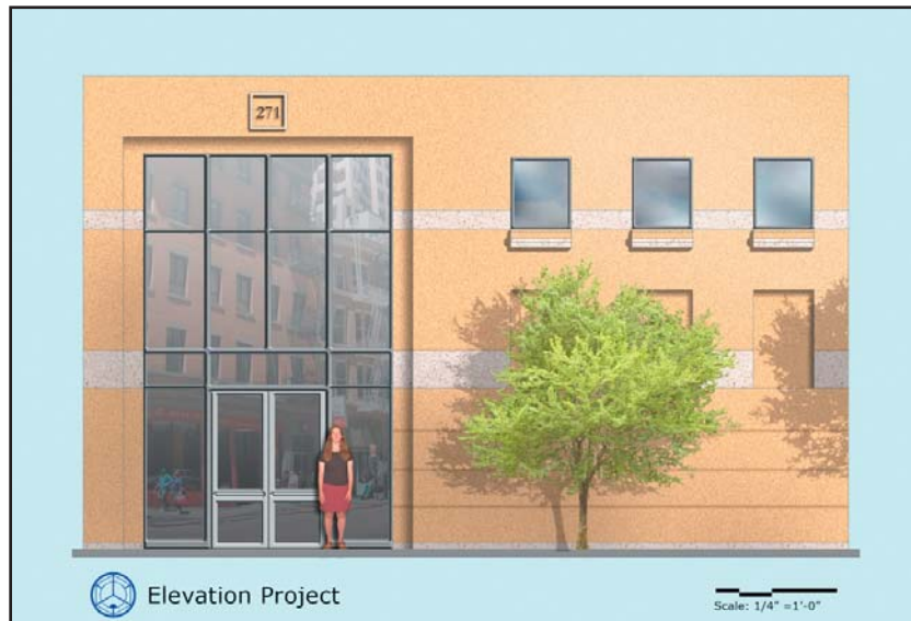
TOP: Original elevation drawing with line weights shown in AutoCAD. BOTTOM: Completed elevation project from Chapter 6. Layer styles, textures, reveals, shading, shadows, reflection, refraction, and entourage were added in Photoshop to enhance the composition.
