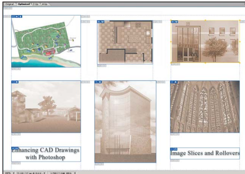
TOP: Original graphic from Chapter 9 to be shown to clients as an optimized web page with rollovers. BOTTOM: Slices and rollovers are applied in ImageReady.
