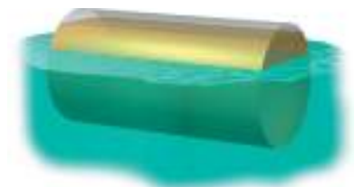
The barrel is not quite full of oil—the top 0.2 foot of the barrel is empty. Figure 8.11
