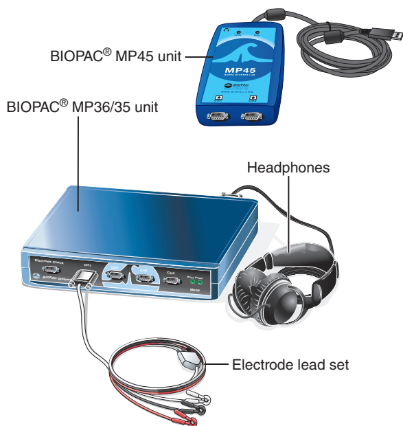
Figure 14.5 Setting up the BIOPAC® equipment to observe recruitment and temporal summation. Plug the headphones into the back of the MP36/35 data acquisition unit or into the top of the MP45 unit, and the electrode lead set into Channel 1. Electrode leads and headphones are shown connected to the MP36/35 unit.
