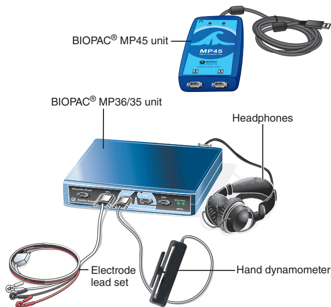
Figure 14.10 Setting up the BIOPAC ® equipment to observe graded muscle contractions and muscle fatigue. Plug the headphones into the back of the MP36/35 data acquisition unit or into the top of the MP45 unit, the electrode lead set into Channel 1, and the hand dynamometer into Channel 2. Electrode leads and dynamometer are shown connected to the MP36/35 unit.
