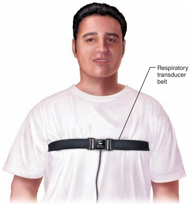
Figure 20.4 Proper placement of the respiratory transducer belt around the subject's thorax.
