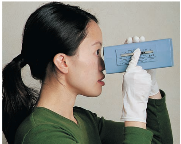
(d) The colors of the green split screen are found by moving the slide with the right index finger. When the two colors match in density, the grams/100 ml and % Hb are read on the scale.
