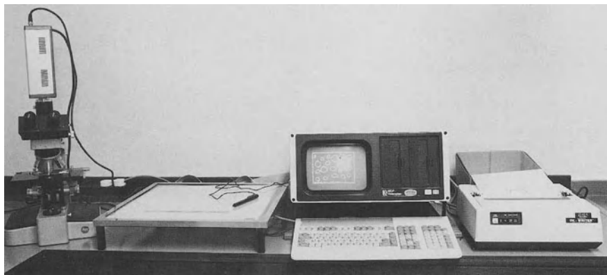
Fig. 3. The digitising tablet, to the right of the microscope, is a commonly used electromagnetic device for transferring stylus coordinates to the computer. It is seen here connected to the MOP-Videoplan, a manual video-based image analysis system (Kontron Electronics, St. Albans, England)
