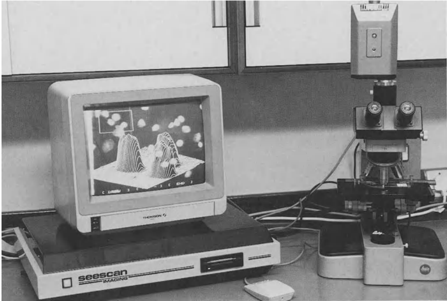
Fig. 4. The mouse ( foreground ) is an increasingly popular interactive peripheral for driving the cursor in interactive image analysis. It is seen here as part of the Seescan Solitaire Plus semiautomatic image analysis system (Seescan Ltd, Cambridge, England)
