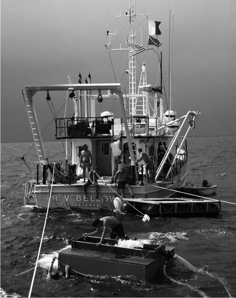
Fig. 2.7 Image showing effluent end of hydraulic dredge dumping into a screen being monitored topside
