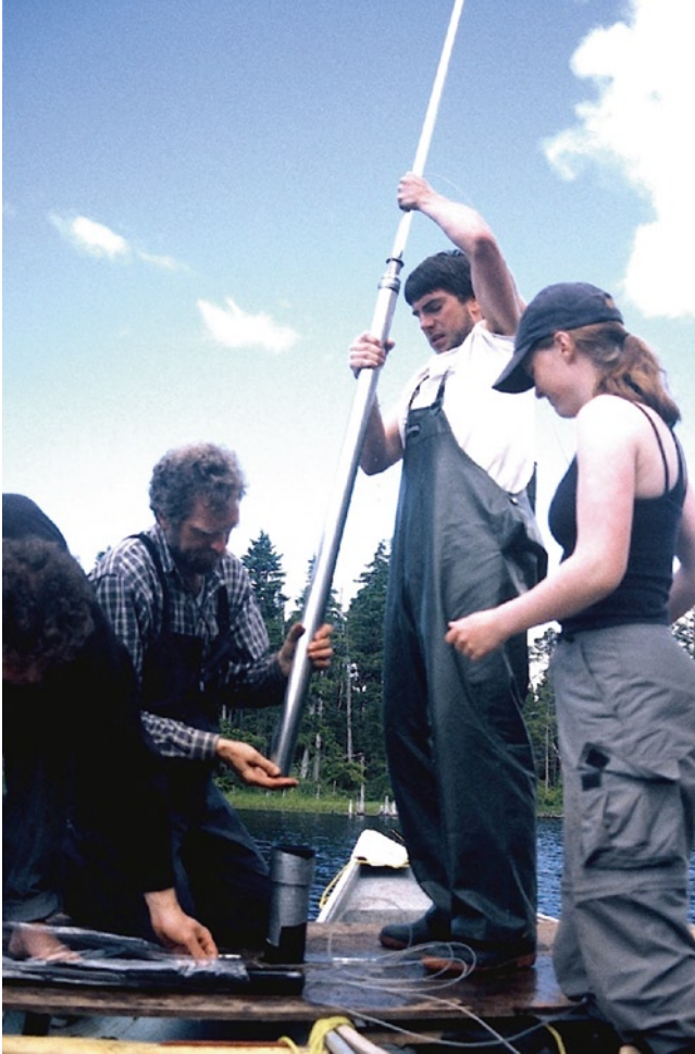
Fig. 3.2 Use of Livingstone core sampler from canoe-based platform, 2001. Sediment cores provide a number of palaeoenvironmental proxies, including vegetation, climate, and sea-level history. Q. Mackie photo
