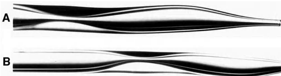
Fig. 2. (A) Photograph of a 5-nL constriction pipet. (B) Photograph of constriction within 5-nL pipet shown in (A). Note that if the constriction were any thinner than this, it would be difficult to take up samples and/or reagents. If the constriction were any larger, the pipet would be difficult to use because the sample/reagent would not stop readily at the constriction.
