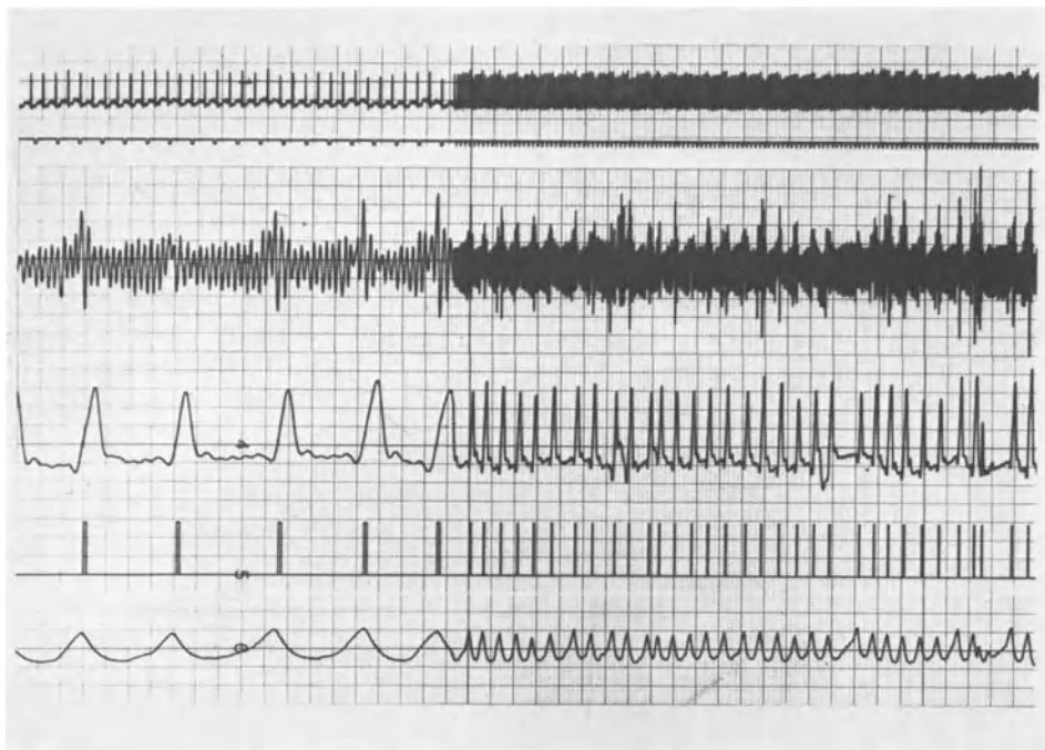
Fig. 1. Analog recording of ECG (trace 1 from above, BRG (trace 2), respiration curve from the BRG (trace 3), respiratory triggers from the BRG (trace 4) and respiration curve from a thermistor probe
