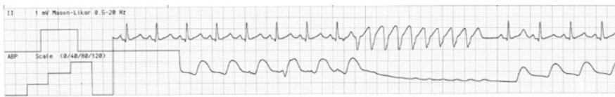
Fig. 6.1 Electrocardiograph (ECG) trace during irreversible electroporation (IRE) treatment of a hepatic tumor below the heart. The synchronizer was not used, and ventricular capture of the IRE pulse resulted in a loss of the arterial pulse because of insufficient time for filling of the left ventricle (Adapted from Ball et al.)
